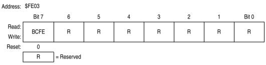
Figure 16-6. Break Flag Control Register (BFCR)
