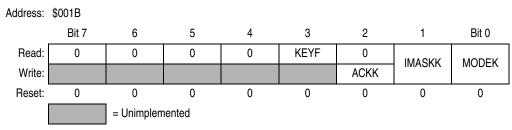
Figure 7-4. Keyboard Status and Control Register (KBSCR)
