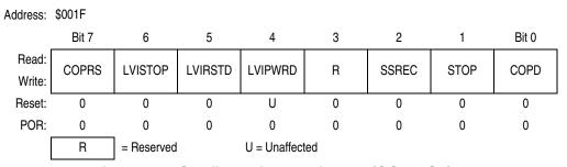
Figure 3-2. Configuration Register 1 (CONFIG1)
