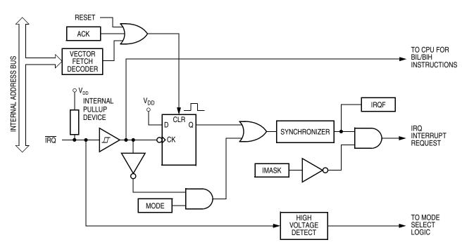
Figure 11-1. IRQ Module Block Diagram
