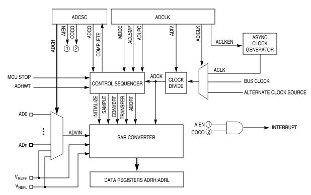
Figure 8-2. ADC10 Block Diagram
