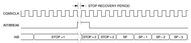
Figure 4-19. Stop Mode Recovery from Interrupt or Break
