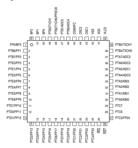
Figure 1-2. 52-Pin LQFP Pin Assignment
