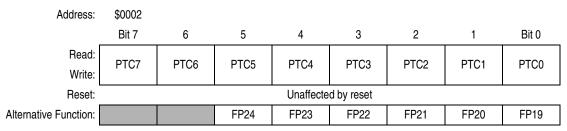
Figure 10-9. Port C Data Register (PTC)
