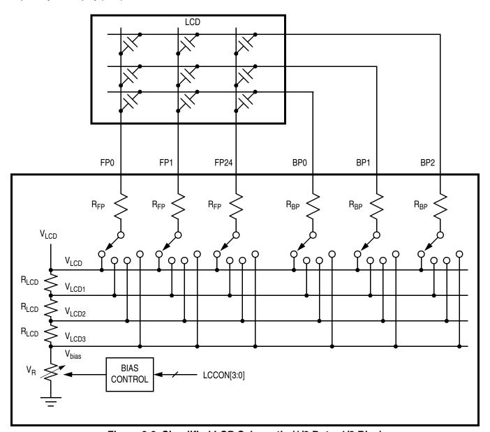
Figure 9-3. Simplified LCD Schematic (1/3 Duty, 1/3 Bias)
