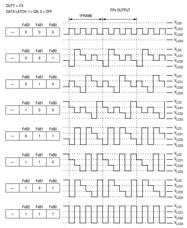
Figure 9-9. 1/3 Duty LCD Frontplane Driver Waveforms
