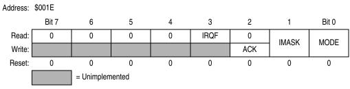
Figure 11-3. IRQ Status and Control Register (INTSCR)
