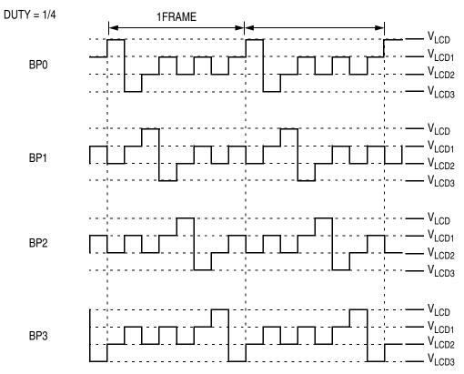
Figure 9-7. 1/4 Duty LCD Backplane Driver Waveforms
