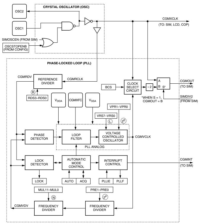
Figure 5-1. CGM Block Diagram
