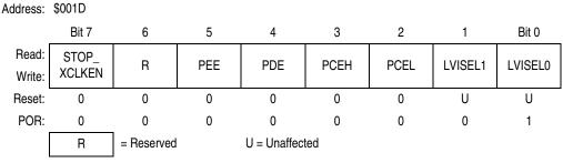
Figure 3-3. Configuration Register 2 (CONFIG2)
