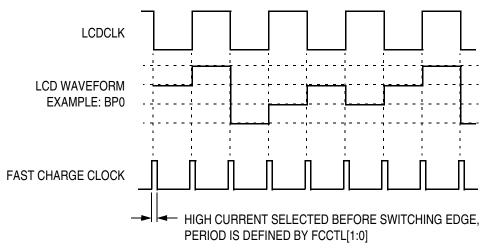
Figure 9-4. Fast Charge Timing
