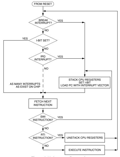
Figure 4-10. Interrupt Processing
