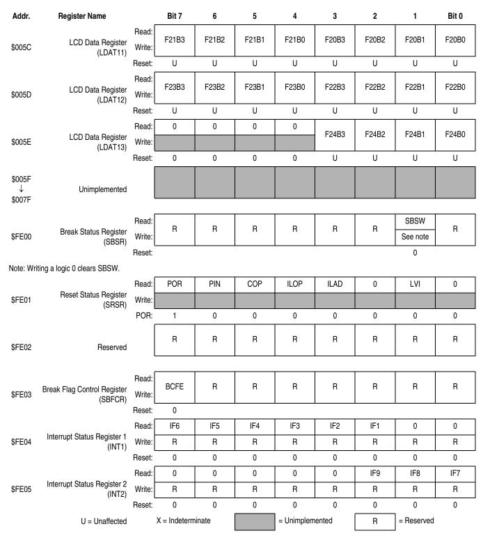
Figure 2-2. Control, Status, and Data Registers (Sheet 7 of 8)
