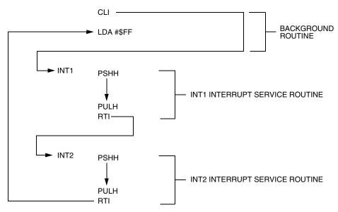
Figure 4-11. Interrupt Recognition Example
