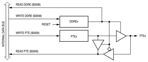
Figure 10-17. Port E I/O Circuit
