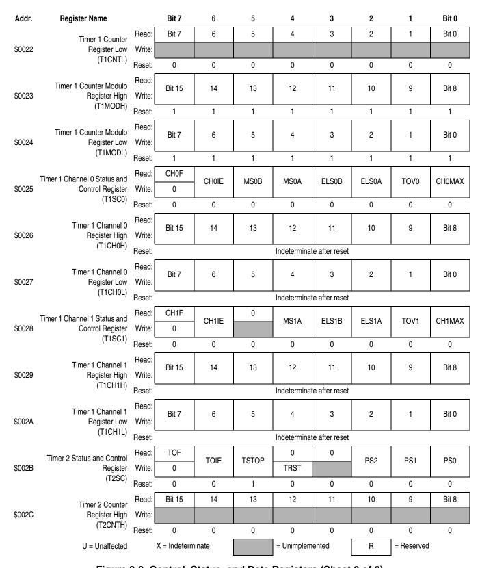
Figure 2-2. Control, Status, and Data Registers (Sheet 3 of 8)
