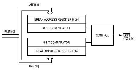
Figure 16-1. Break Module Block Diagram
