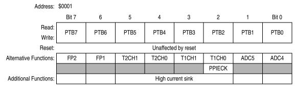
Figure 10-5. Port B Data Register (PTB)
