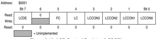
Figure 9-16. LCD Control Register (LCDCR)
