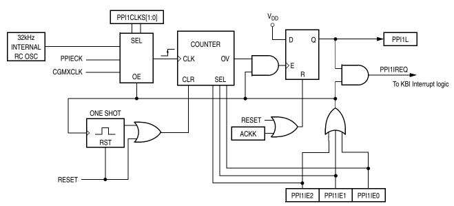
Figure 7-1. Programmable Periodic Interrupt Block Diagram
