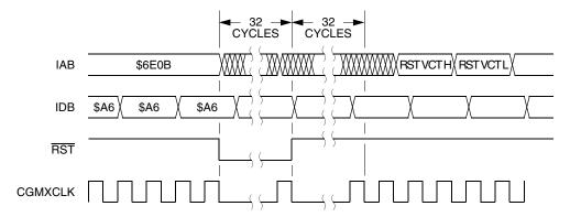
Figure 4-17. Wait Recovery from Internal Reset
