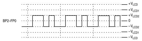
Figure 9-15. "e" Segment Voltage Waveform
