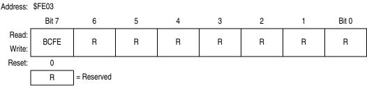
Figure 4-22. Break Flag Control Register (BFCR)
