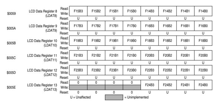
Figure 9-18. LCD Data Registers 1-13 (LDAT1-LDAT13)
