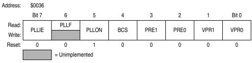
Figure 5-4. PLL Control Register (PCTL)
