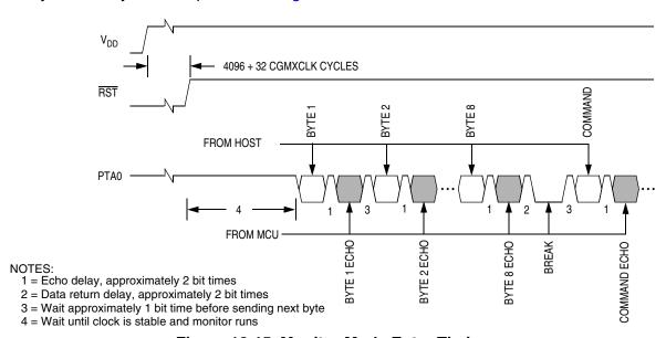
Figure 16-15. Monitor Mode Entry Timing
