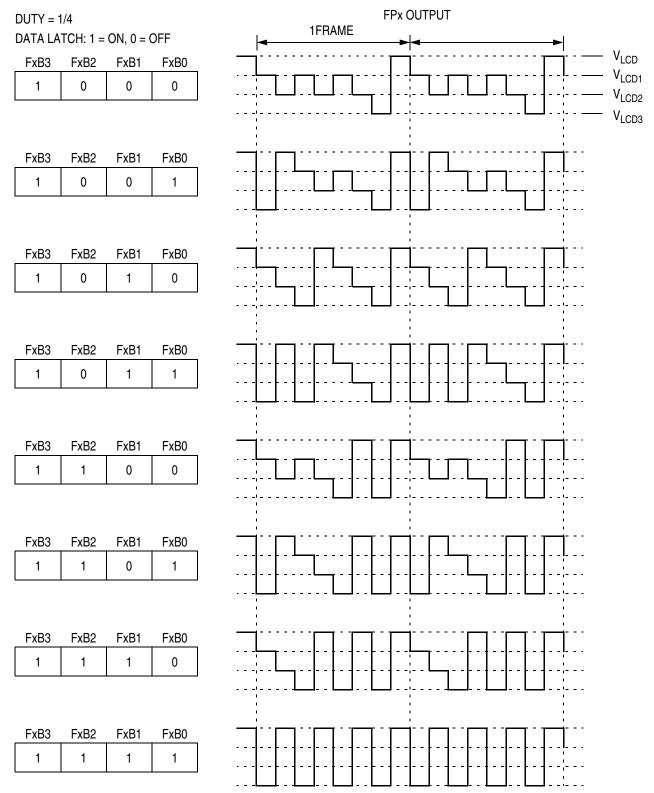
Figure 9-11. 1/4 Duty LCD Frontplane Driver Waveforms (continued)
