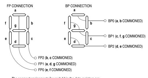
The segment assignments for each bit in the data registers are:
