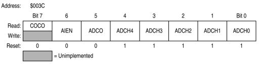
Figure 8-3. ADC10 Status and Control Register (ADCSC)
