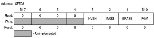
Figure 2-3. FLASH Control Register (FLCR)
