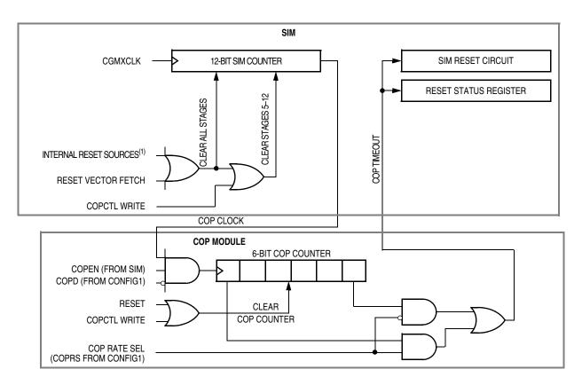
Figure 13-1. COP Block Diagram
