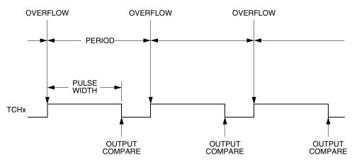
Figure 6-3. PWM Period and Pulse Width
