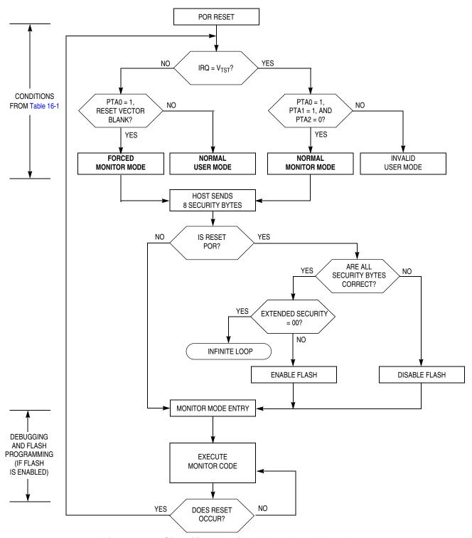
Figure 16-7. Simplified Monitor Mode Entry Flowchart
