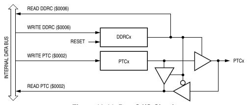
Figure 10-11. Port C I/O Circuit
