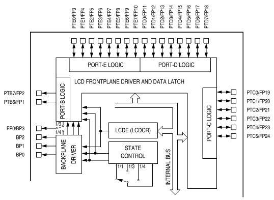
Figure 9-2. LCD Block Diagram
