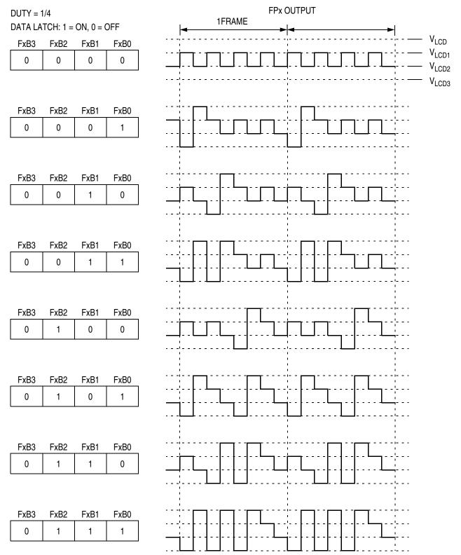
Figure 9-10. 1/4 Duty LCD Frontplane Driver Waveforms
