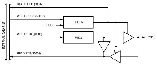
Figure 10-14. Port D I/O Circuit
