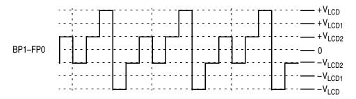
Figure 9-14. "f" Segment Voltage Waveform
