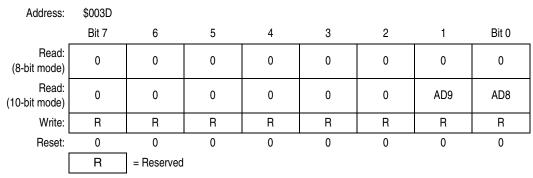
Figure 8-4. ADC10 Data Register High (ADRH)
