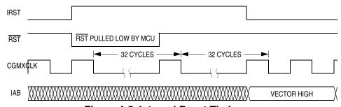
Figure 4-5. Internal Reset Timing
