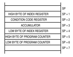
Figure 16-14. Stack Pointer at Monitor Mode Entry
