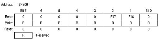
Figure 4-14. Interrupt Status Register 3 (INT3)
