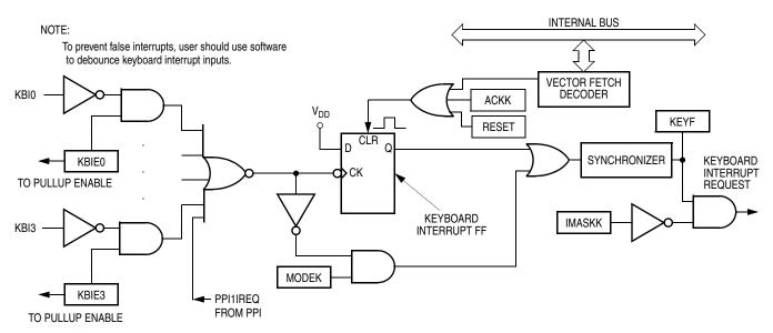
Figure 12-2. Keyboard Interrupt Block Diagram
