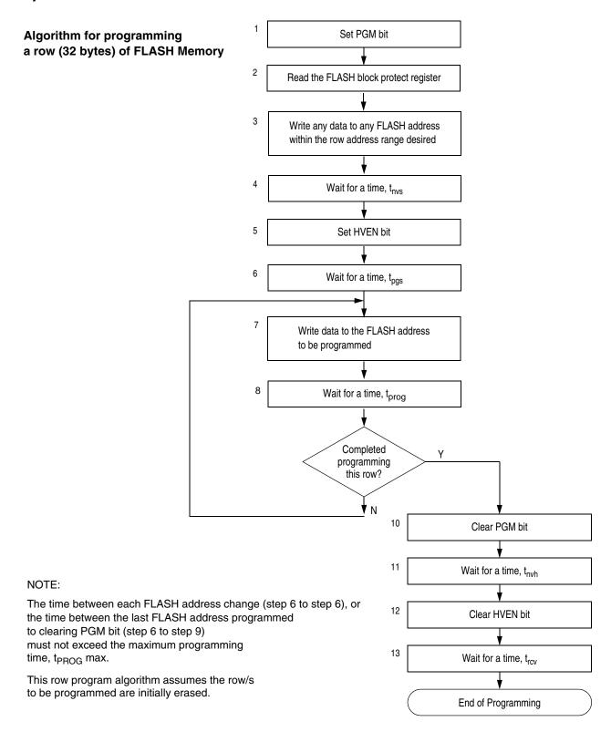
Figure 2-4. FLASH Programming Flowchart
