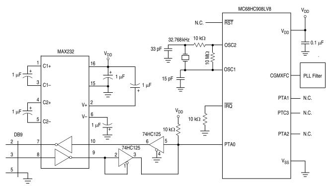
Figure 16-9. Forced Monitor Circuit ( $V_{\overline{IRQ}} = V_{SS}$ )
