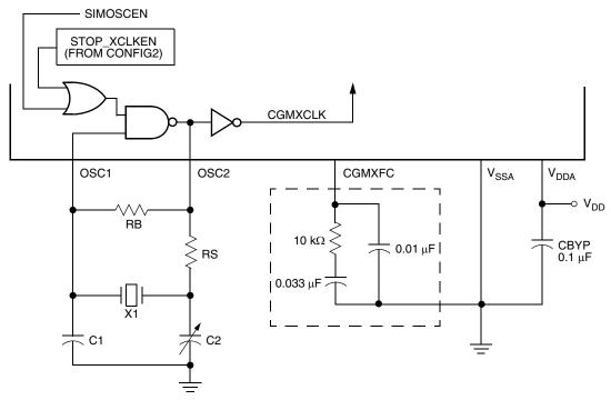
Note: Filter network in box can be replaced with a 0.47 µF capacitor, but will degrade stability.
