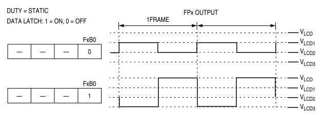
Figure 9-8. Static LCD Frontplane Driver Waveforms
