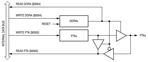
Figure 10-4. Port A I/O Circuit
