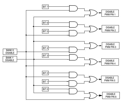
Figure 12-27. PWM Disabling Decode Scheme
