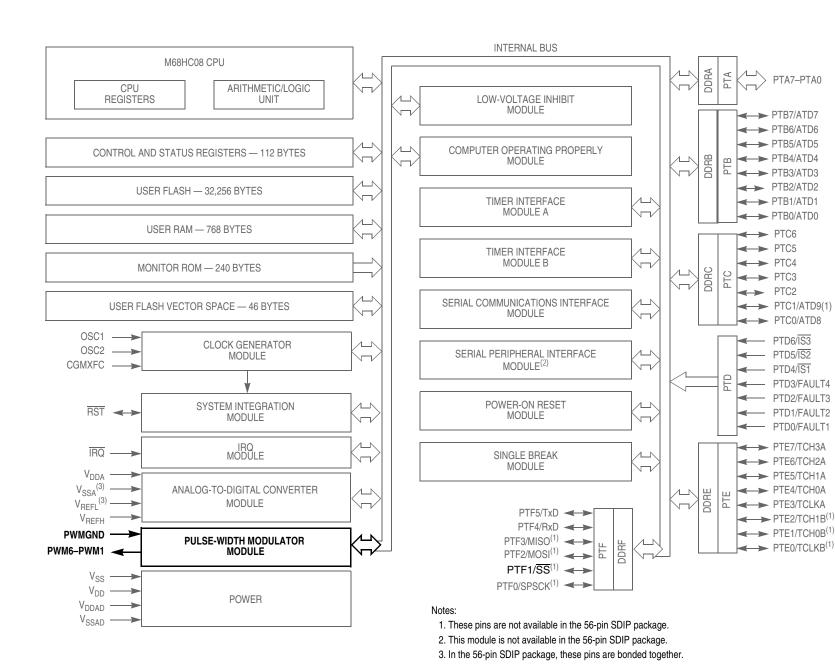
Figure 12-1. Block Diagram Highlighting PWMMC Block and Pins
