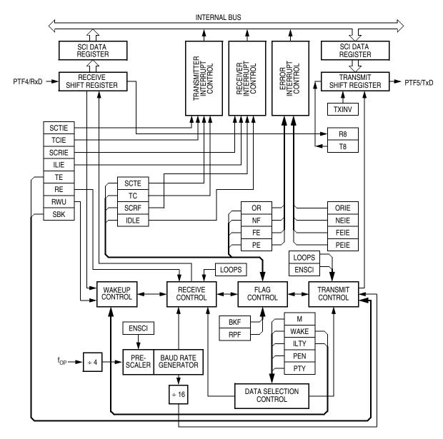
Figure 13-2. SCI Module Block Diagram
