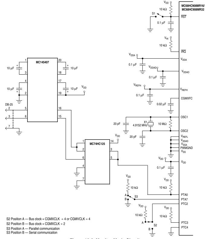
Figure 18-8. Monitor Mode Circuit
