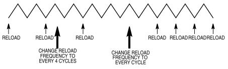
Figure 12-6. Reload Frequency Change
