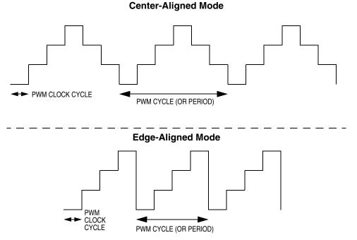
Figure 12-47. PWM Clock Cycle and PWM Cycle Definitions
