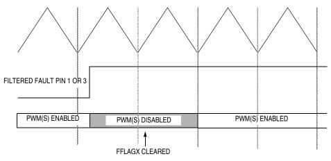
Figure 12-29. PWM Disabling in Manual Mode (Example 1)
