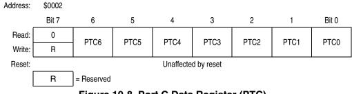
Figure 10-8. Port C Data Register (PTC)
