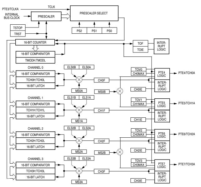
Figure 16-2. TIMA Block Diagram
