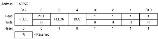
Figure 4-5. PLL Control Register (PCTL)
