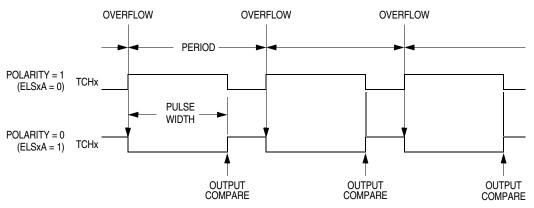
Figure 17-4. PWM Period and Pulse Width
