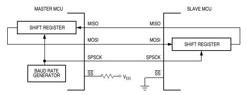
Figure 15-4. Full-Duplex Master-Slave Connections
