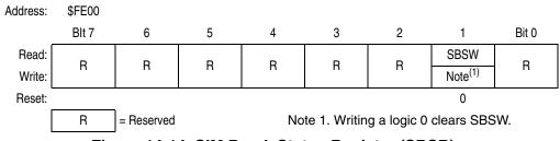
Figure 14-14. SIM Break Status Register (SBSR)
