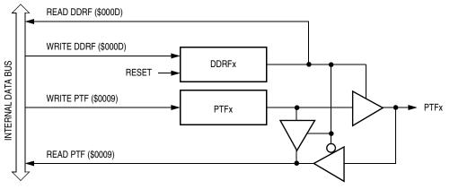
Figure 10-18. Port F I/O Circuit
