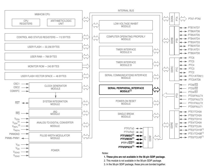
Figure 15-1. Block Diagram Highlighting SPI Block and Pins
