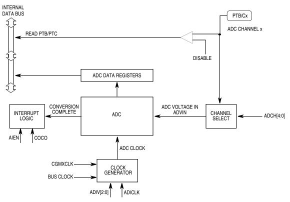
Figure 3-2. ADC Block Diagram
