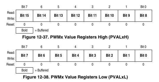
The 16-bit signed value stored in this register determines the duty cycle of the PWM. The duty cycle is defined as: (PWM value/modulus) x 100.
