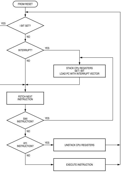
Figure 8-3. IRQ Interrupt Flowchart
