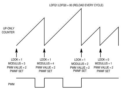
Figure 12-11. Edge-Aligned Modulus Loading
