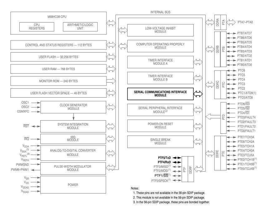
Figure 13-1. Block Diagram Highlighting SCI Block and Pins
