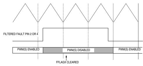
Figure 12-30. PWM Disabling in Manual Mode (Example 2)
