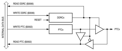
Figure 10-10. Port C I/O Circuit
