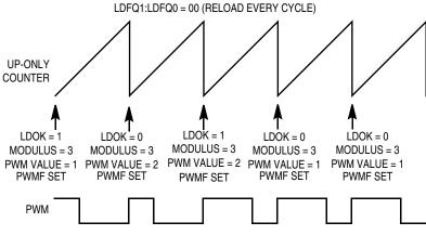
Figure 12-10. Edge-Aligned PWM Value Loading
