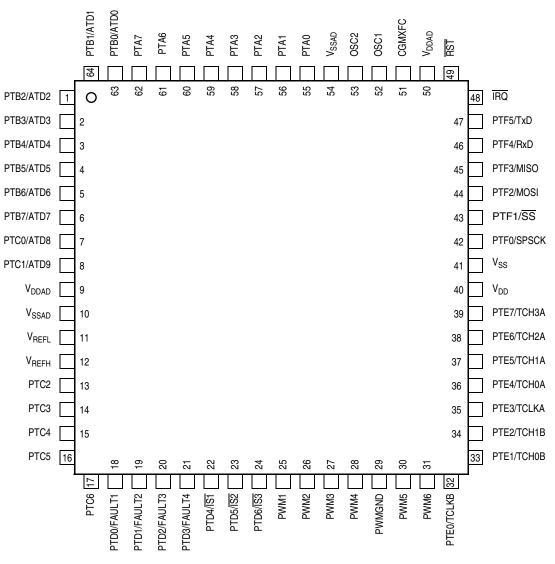
Figure 1-2. 64-Pin QFP Pin Assignments
