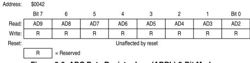
Figure 3-9. ADC Data Register Low (ADRL) 8-Bit Mode
