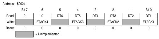
Figure 12-45. Fault Acknowledge Register (FTACK)
