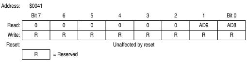
Figure 3-6. ADC Data Register High (ADRH) Right Justified Mode
