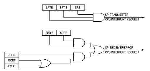
Figure 15-11. SPI Interrupt Request Generation
