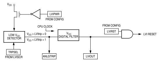
Figure 9-1. LVI Module Block Diagram
