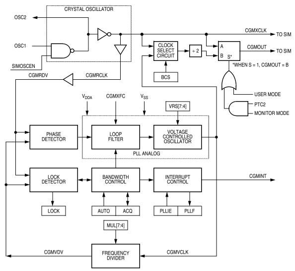
Figure 4-1. CGM Block Diagram
