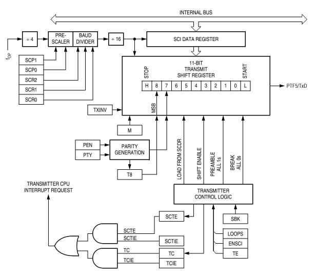
Figure 13-5. SCI Transmitter
