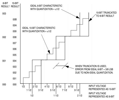
**NOTE** Quantization error is affected when only the most significant eight bits are
