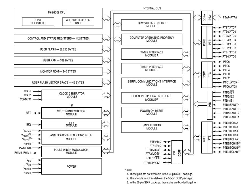
Figure 1-1. MCU Block Diagram
