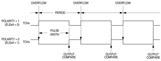
Figure 16-4. PWM Period and Pulse Width
