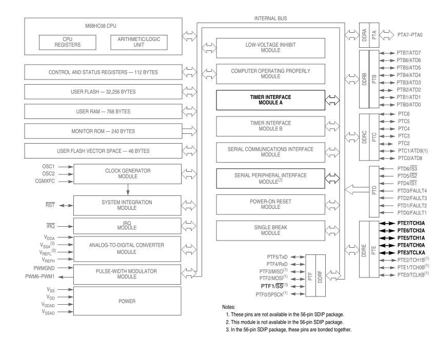
Figure 16-1. Block Diagram Highlighting TIMA Block and Pins
