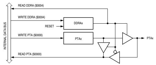
Figure 10-4. Port A I/O Circuit
