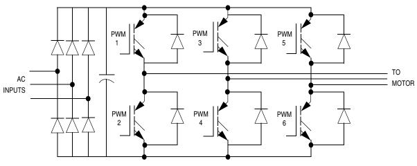
Figure 12-13. Typical AC Motor Drive
