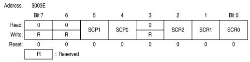
Figure 13-15. SCI Baud Rate Register (SCBR)
