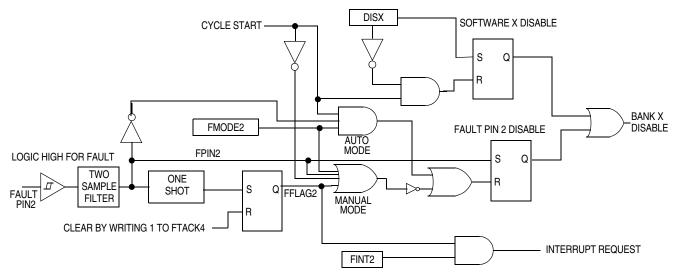
The example is of fault pin 2 with DISX. Fault pin 4 with DISY is logically similar and affects BANK Y disable.
