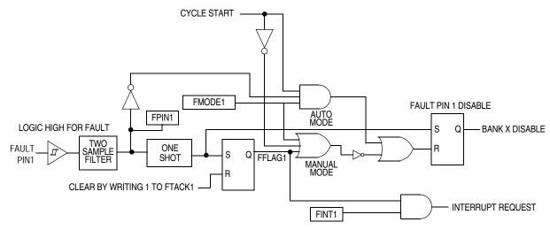
The example is of fault pin 1. Fault pin 3 is logically similar and affects BANK Y disable.
