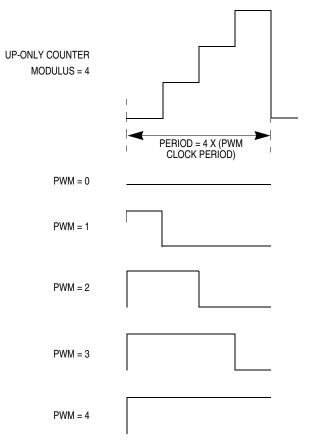
Figure 12-5. Edge-Aligned PWM (Positive Polarity)
