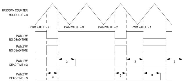
Figure 12-17. Dead-Time and Small Pulse Widths
