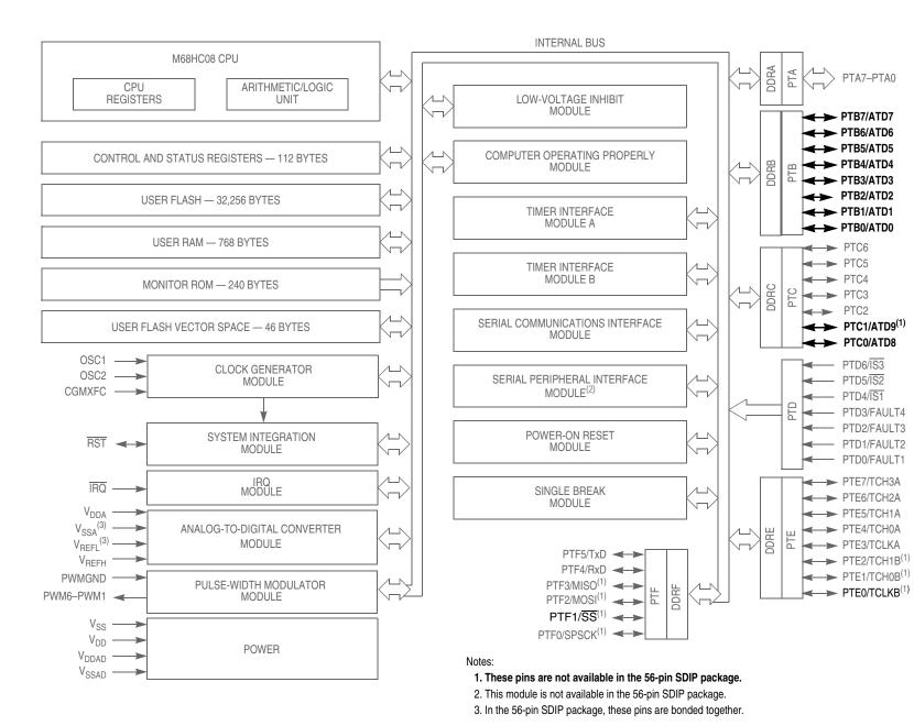
Figure 3-1. Block Diagram Highlighting ADC Block and Pins
