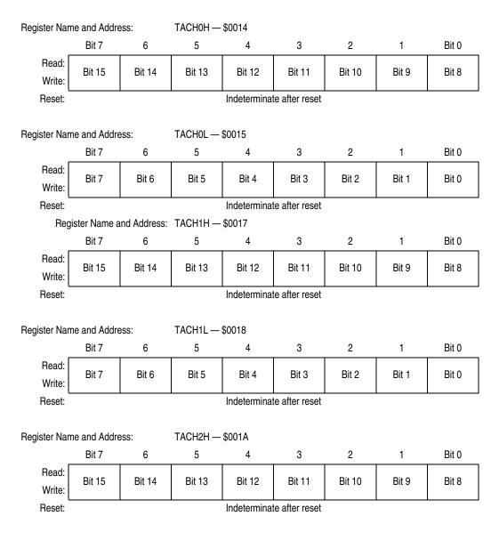
Figure 16-10. TIMA Channel Registers (TACH0H/L–TACH3H/L)
