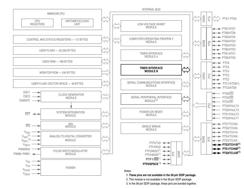
Figure 17-1. Block Diagram Highlighting TIMB Block and Pins
