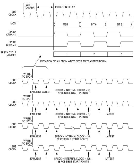
Figure 15-8. Transmission Start Delay (Master)
