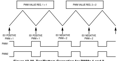
Figure 12-20. Top/Bottom Correction for PWMs 1 and 2
