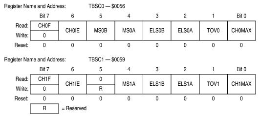
Figure 17-8. TIMB Channel Status and Control Registers (TBSC0–TBSC1)
