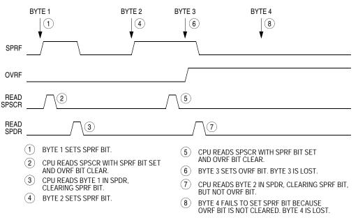
Figure 15-9. Missed Read of Overflow Condition
