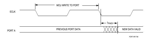
Figure 21-7. Port Write Timing Diagram
