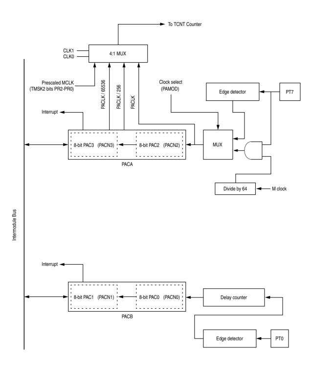
Figure 15-4. 16-Bit Pulse Accumulators Block Diagram
