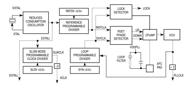
Figure 12-2. PLL Functional Diagram
