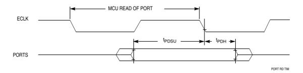
Figure 21-6. Port Read Timing Diagram
