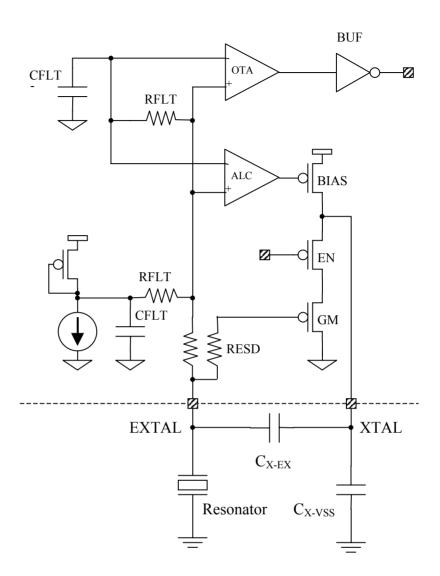
Figure 13-2. MC68HC912Dx128C Colpitts Oscillator Architecture
