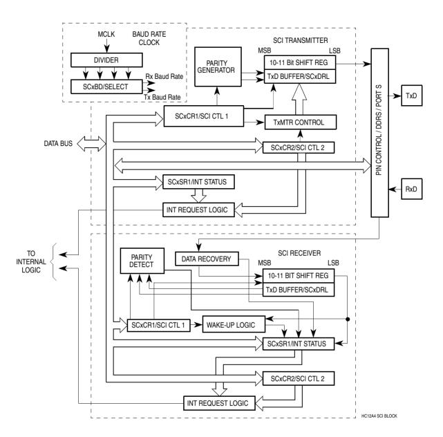
Figure 16-2. Serial Communications Interface Block Diagram
