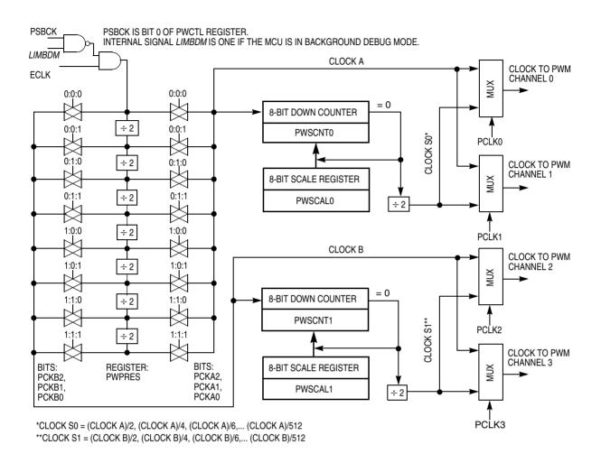
Figure 14-3. PWM Clock Sources
