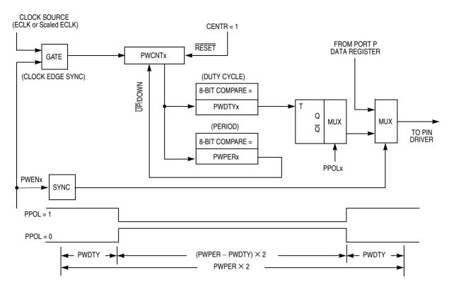
Figure 14-2. Block Diagram of PWM Center-Aligned Output Channel
