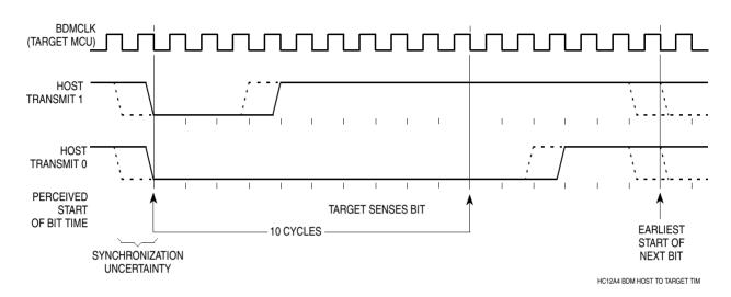
Figure 20-1. BDM Host to Target Serial Bit Timing
