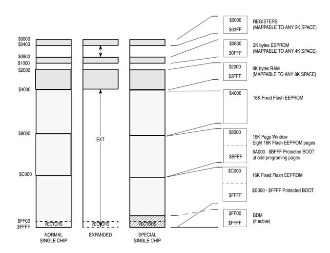
Figure 6-1. MC68HC912DT128A Memory Map after reset
