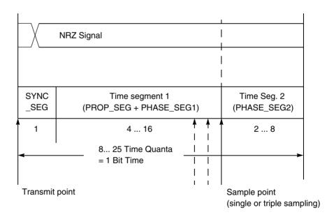
Figure 18-8. Segments within the Bit Time
