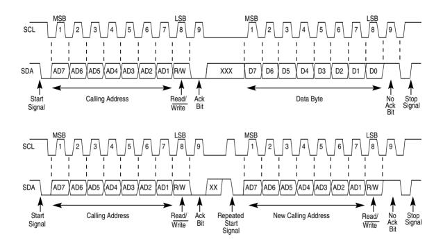
Figure 17-2. IIC Transmission Signals
