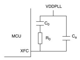
Figure 3-4. PLL Loop Filter Connections
