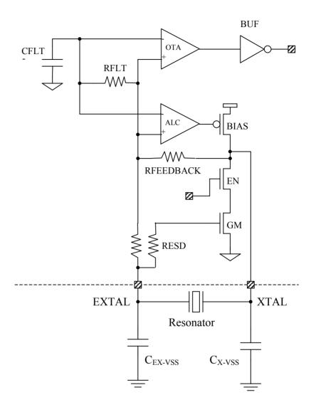
Figure 13-4. MC68HC912Dx128P Pierce Oscillator Architecture
