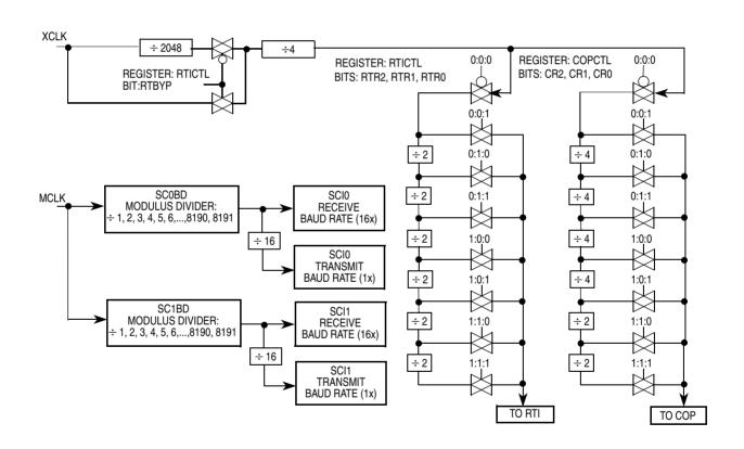
Figure 12-7. Clock Chain for SCI0, SCI1, RTI, COP
