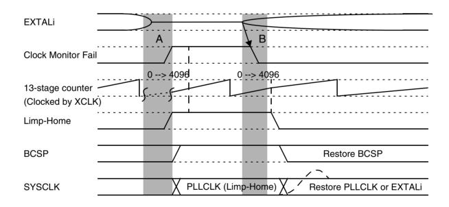
Figure 12-3. Clock Loss during Normal Operation
