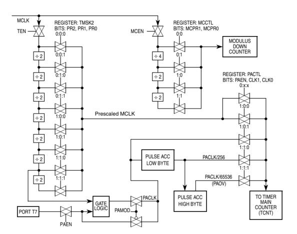
Figure 12-8. Clock Chain for ECT
