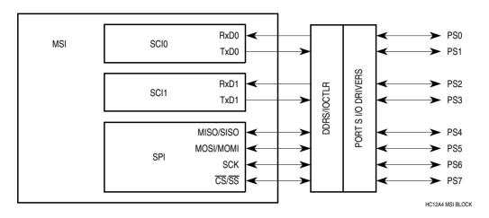
Figure 16-1. Multiple Serial Interface Block Diagram
