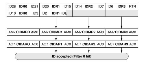
Figure 18-3. 32-bit Maskable Identifier Acceptance Filters
