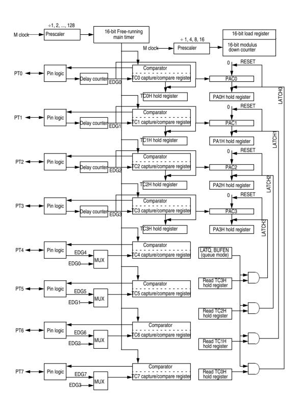
Figure 15-2. Timer Block Diagram in Queue Mode
