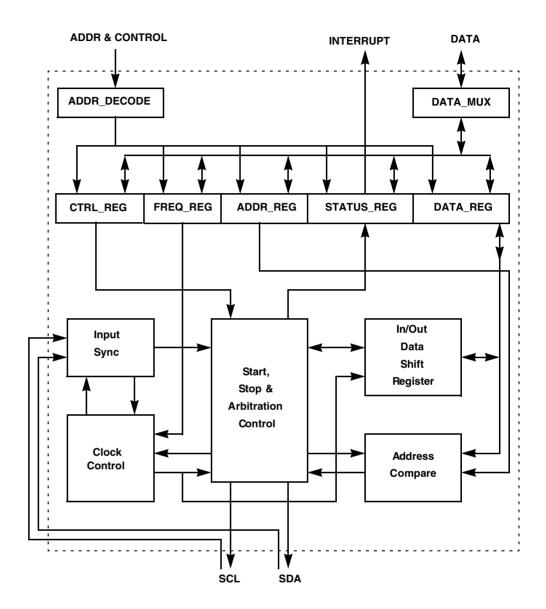
Figure 17-1. IIC Block Diagram
