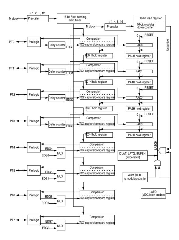
Figure 15-1. Timer Block Diagram in Latch Mode
