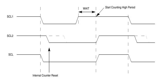
Figure 17-3. IIC Clock Synchronization
