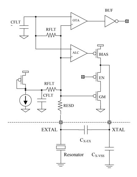
Figure 13-1. MC68HC912DT128A Colpitts Oscillator Architecture
