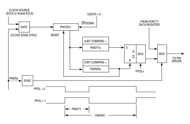
Figure 14-1. Block Diagram of PWM Left-Aligned Output Channel
