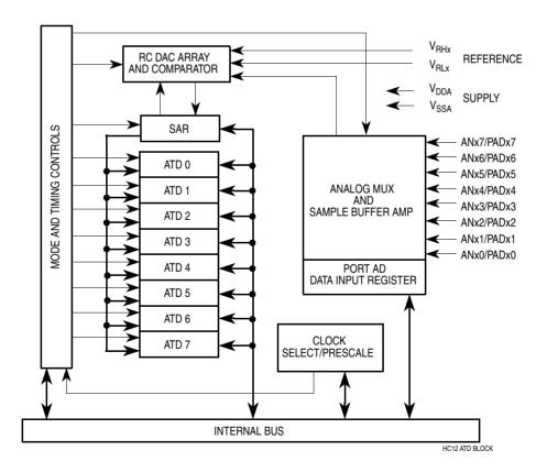
Figure 19-1. Analog-to-Digital Converter Block Diagram
