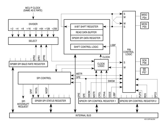
Figure 16-3. Serial Peripheral Interface Block Diagram
