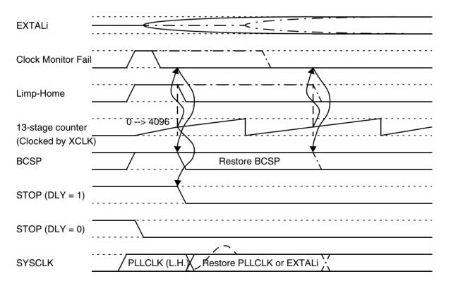
Figure 12-5. STOP Exit and Fast STOP Recovery
