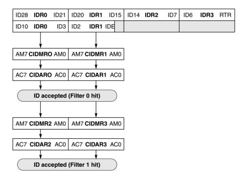
Figure 18-4. 16-bit Maskable Acceptance Filters
