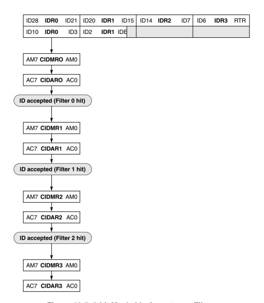
Figure 18-5. 8-bit Maskable Acceptance Filters
