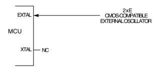
Figure 3-5. External Oscillator Connections
