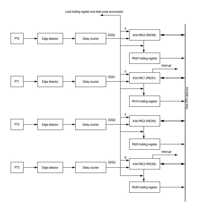
Figure 15-3. 8-Bit Pulse Accumulators Block Diagram
