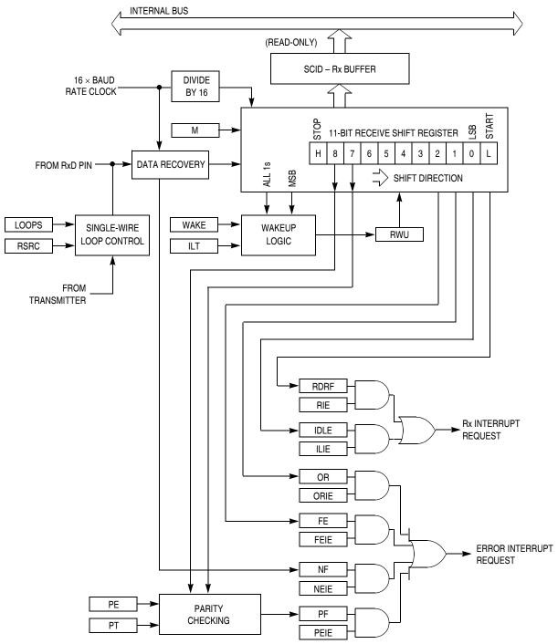
Figure 11-3. SCI Receiver Block Diagram
