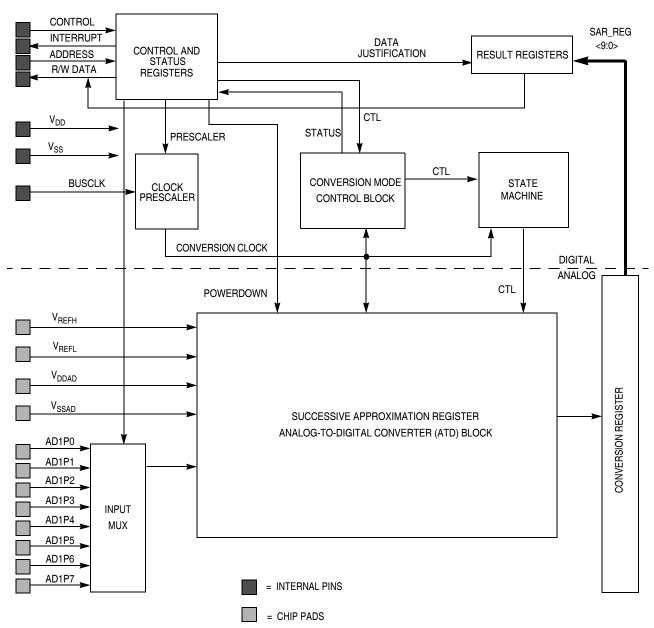
Figure 14-2. ATD Block Diagram
