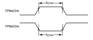
Figure A-15. Timer Input Capture Pulse
