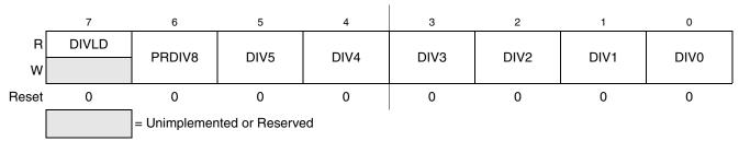
Figure 4-4. Flash Clock Divider Register (FCDIV)
