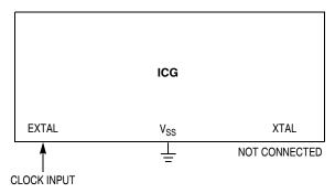
Figure 7-4. External Clock Connections
