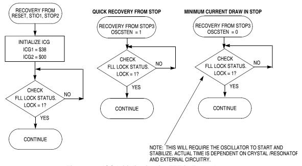
Figure 7-8. ICG Initialization for FEE in Example #1
