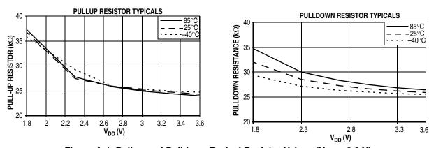
Figure A-1. Pullup and Pulldown Typical Resistor Values ( $V_{DD} = 3.0 \text{ V}$ )
