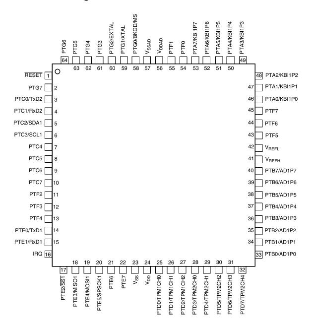
Figure 2-1. MC9S08GBxxA in 64-Pin LQFP Package
