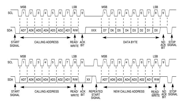
Figure 13-8. IIC Bus Transmission Signals
