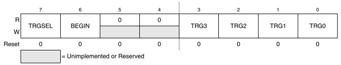
Figure 15-8. Debug Trigger Register (DBGT)
