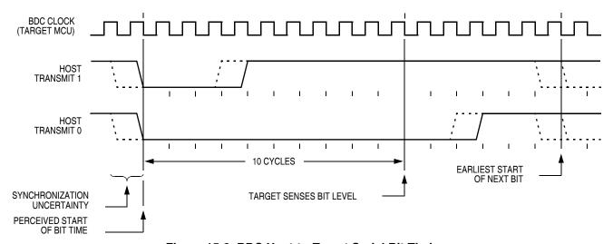
Figure 15-2. BDC Host-to-Target Serial Bit Timing
