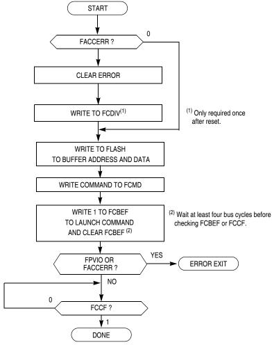
Figure 4-2. Flash Program and Erase Flowchart
