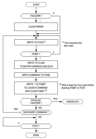
Figure 4-3. Flash Burst Program Flowchart
