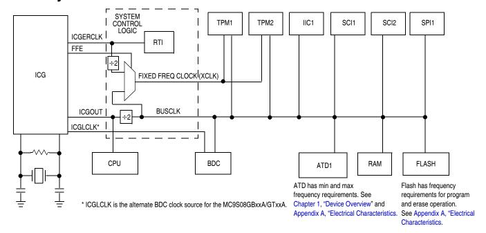
Figure 1-2. System Clock Distribution Diagram
