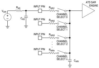
Figure 14-3. Resistor and Capacitor Placement
