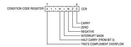
Figure 8-2. Condition Code Register
