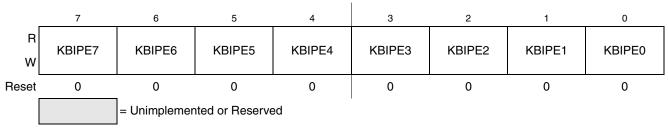
Figure 9-5. KBI Pin Enable Register (KBI1PE)
