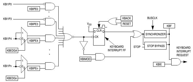
Figure 9-3. KBI Block Diagram
