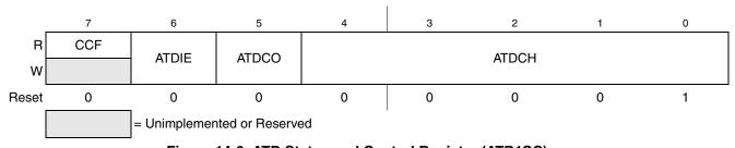
Figure 14-6. ATD Status and Control Register (ATD1SC)
