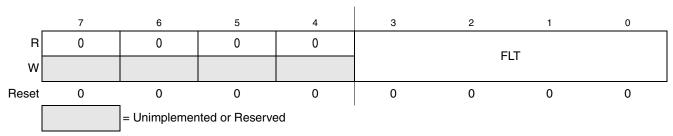
Figure 7-16. ICG Upper Filter Register (ICGFLTU)
