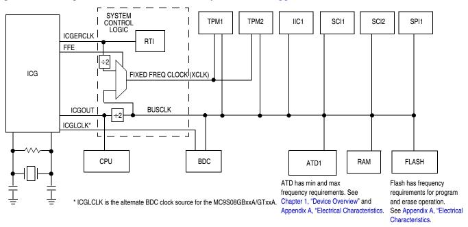
Figure 7-1. System Clock Distribution Diagram
