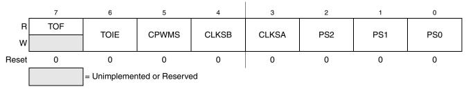
Figure 10-5. Timer x Status and Control Register (TPMxSC)
