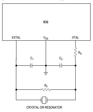
Figure 7-5. External Frequency Reference Connection
