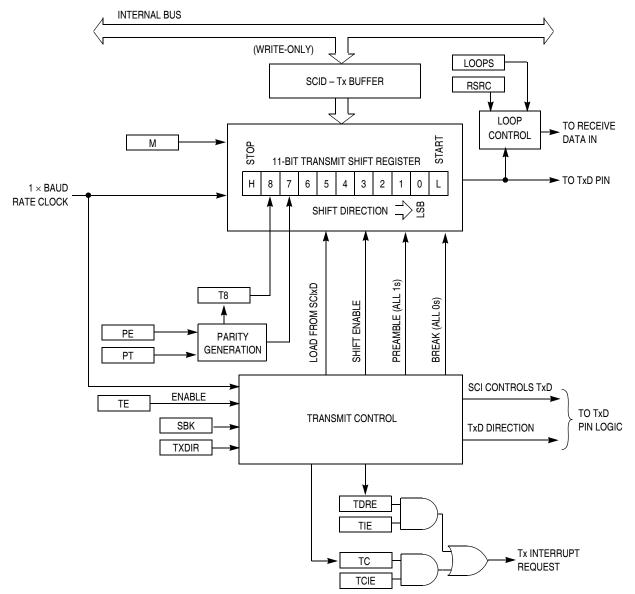
Figure 11-2. SCI Transmitter Block Diagram
