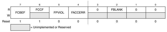
Figure 4-8. Flash Status Register (FSTAT)
