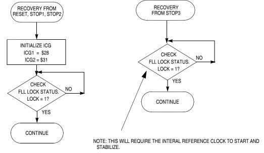
Figure 7-10. ICG Initialization and Stop Recovery for Example #3
