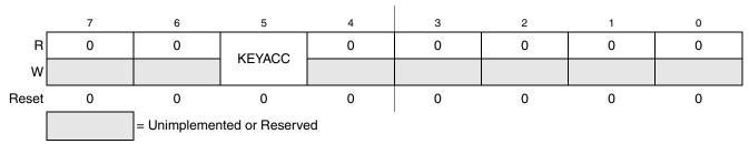
Figure 4-6. Flash Configuration Register (FCNFG)
