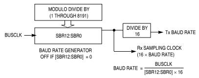
Figure 11-12. SCI Baud Rate Generation
