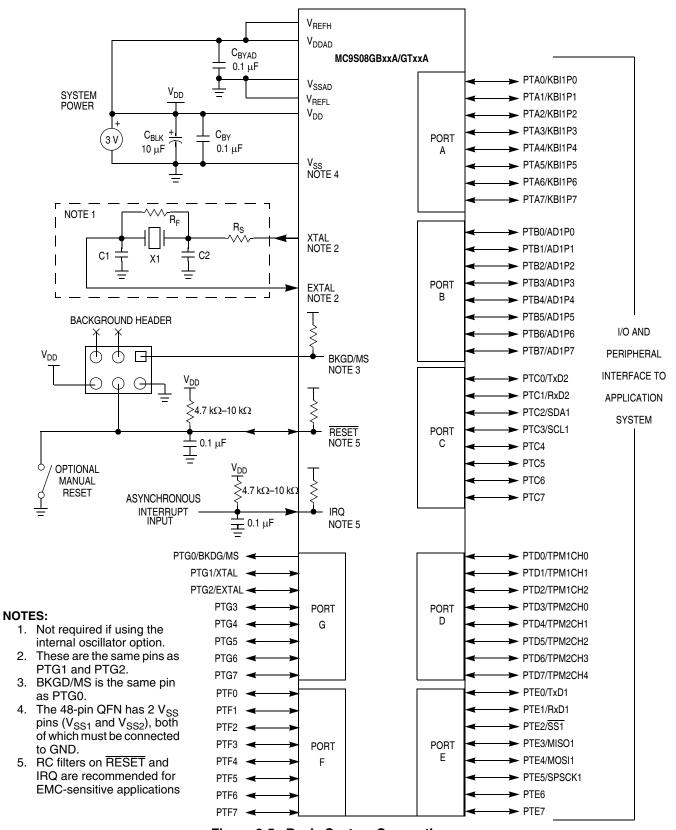
Figure 2-5. Basic System Connections
