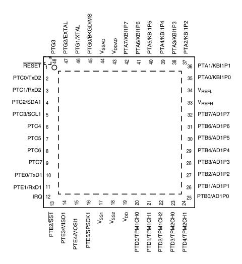
Figure 2-2. MC9S08GTxxA in 48-Pin QFN Package
