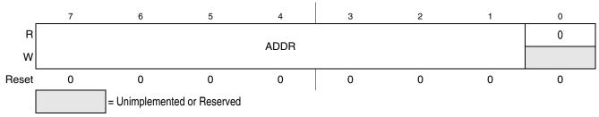
Figure 13-3. IIC Address Register (IIC1A)
