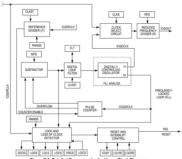
Figure 7-6. Detailed Frequency-Locked Loop Block Diagram
