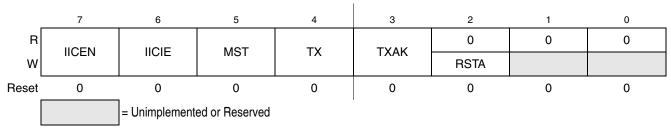
Figure 13-5. IIC Control Register (IIC1C)
