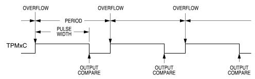
Figure 10-3. PWM Period and Pulse Width (ELSnA = 0)
