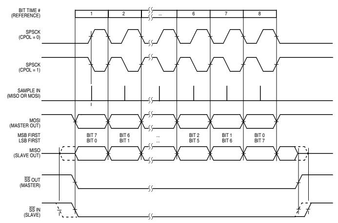
Figure 12-11. SPI Clock Formats (CPHA = 0)
