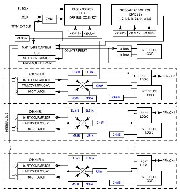
Figure 10-2. TPM Block Diagram
