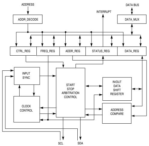
Figure 13-2. IIC Functional Block Diagram
