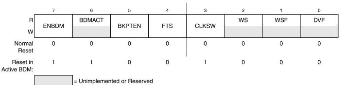
Figure 15-5. BDC Status and Control Register (BDCSCR)
