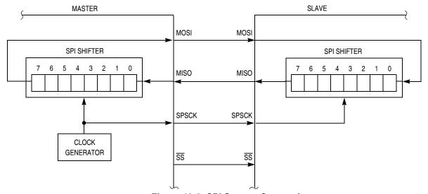
Figure 12-2. SPI System Connections
