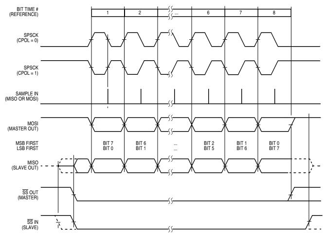
Figure 12-10. SPI Clock Formats (CPHA = 1)
