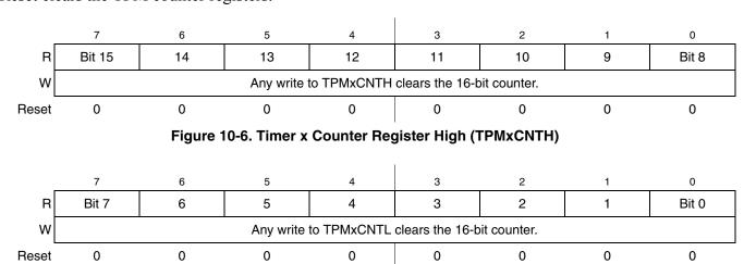
Figure 10-7. Timer x Counter Register Low (TPMxCNTL)
