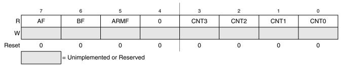
Figure 15-9. Debug Status Register (DBGS)
