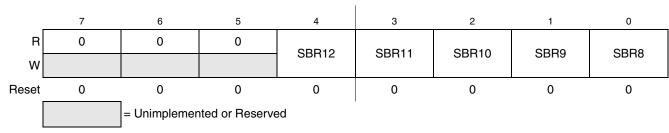
Figure 11-4. SCI Baud Rate Register (SCIxBDH)
