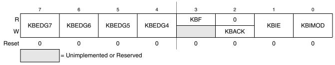
Figure 9-4. KBI Status and Control Register (KBI1SC)
