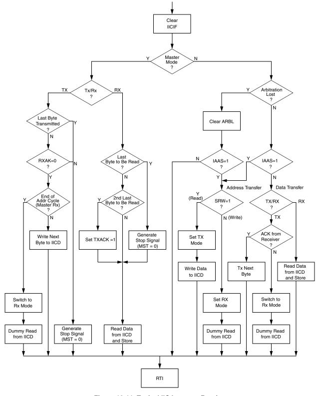
Figure 13-11. Typical IIC Interrupt Routine
