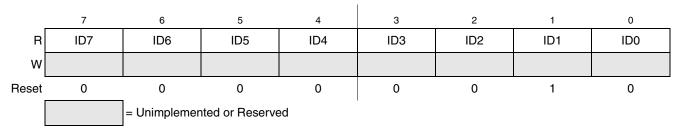
Figure 5-7. System Device Identification Register Low (SDIDL)
