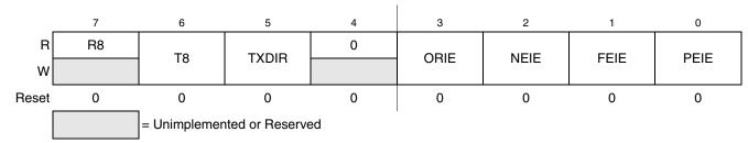
Figure 11-10. SCI Control Register 3 (SCIxC3)
