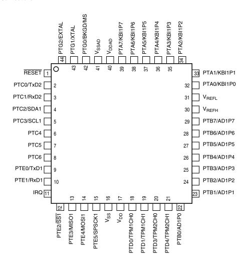
Figure 2-3. MC9S08GTxxA in 44-Pin QFP Package
