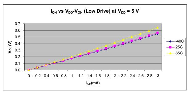
Figure 6. Typical  $I_{OH}$  (Low Drive) vs  $V_{DD}$ - $V_{OH}$  at  $V_{DD}$  = 5 V
