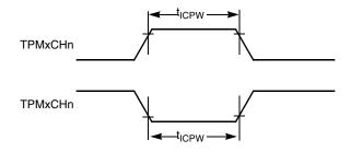
**Figure 17. Timer Input Capture Pulse**
