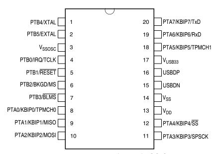
Figure 3. MC9S08JS16 Series in 20-pin SOIC Package
