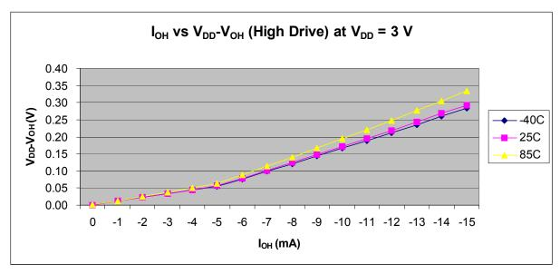
Figure 5. Typical  $I_{OH}$  (High Drive) vs  $V_{DD}$ - $V_{OH}$  at  $V_{DD}$  = 3 V
