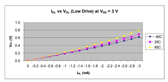
Figure 10.  $I_{OL}$  vs  $V_{OL}$  (Low Drive) at  $V_{DD}$  = 3 V
