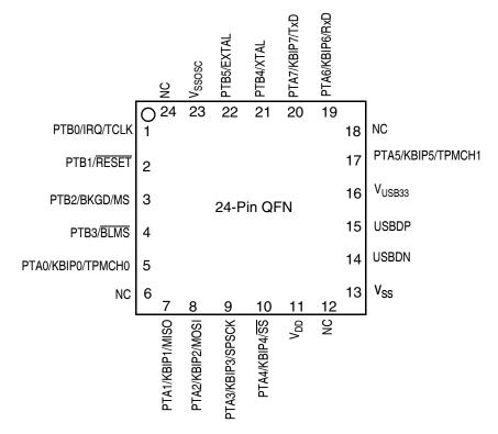
Figure 2. MC9S08JS16 Series in 24-QFN Package
