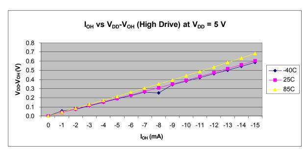
Figure 7. Typical  $I_{OH}$  (High Drive) vs  $V_{DD}$ - $V_{OH}$  at  $V_{DD}$  = 5 V
