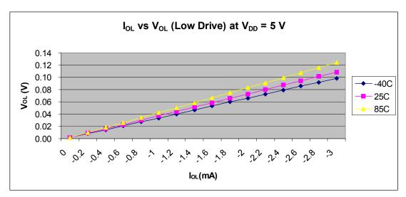
Figure 8.  $I_{OL}$  vs  $V_{OL}$  (Low Drive) at  $V_{DD}$  = 5 V
