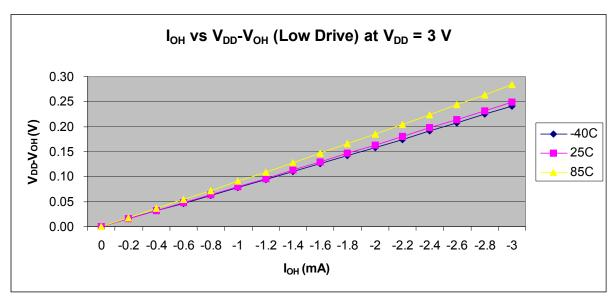
Figure 4. Typical  $I_{OH}$  (Low Drive) vs  $V_{DD}$ - $V_{OH}$  at  $V_{DD}$  = 3 V
