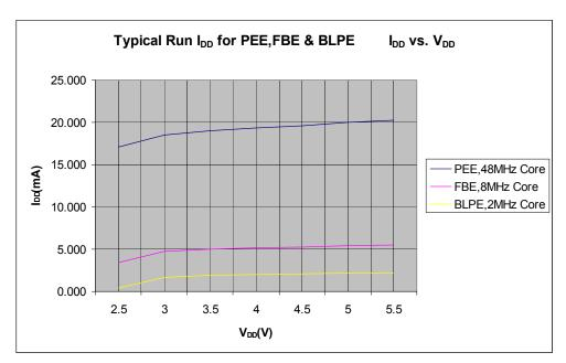
Figure 12. Typical Run  $\rm I_{DD}$  for PEE, FBE and BLPE Modes ( $\rm I_{DD}$  vs.  $\rm V_{DD})$
