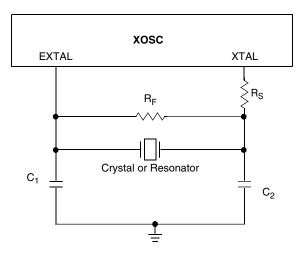
Figure 16. Typical crystal or resonator circuit
