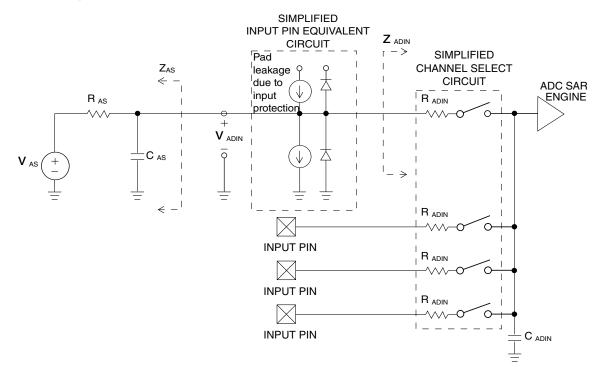
Figure 17. ADC input impedance equivalency diagram
