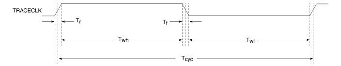
Figure 12. TRACE\_CLKOUT specifications
