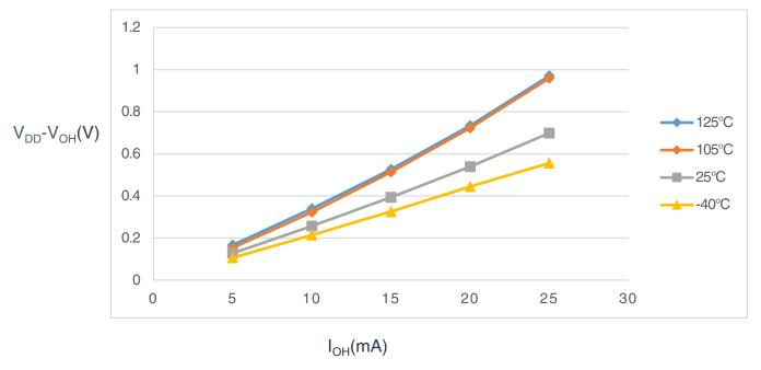
Figure 5. Typical  $I_{OH}$  Vs.  $V_{DD}$ - $V_{OH}$  (high drive strength) ( $V_{DD}$  = 3 V)
