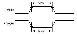
Figure 15. Timer input capture pulse
