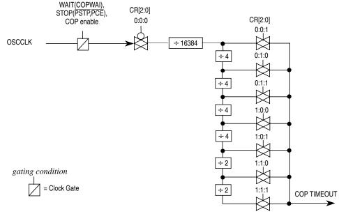
Figure 4-21. Clock Chain for COP
