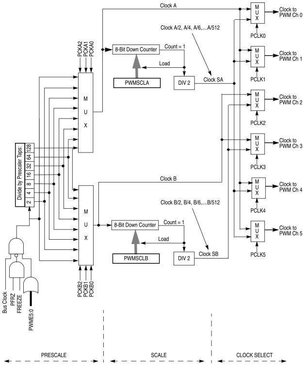
Figure 12-34. PWM Clock Select Block Diagram
