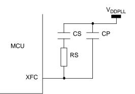
Figure 4-2. PLL Loop Filter Connections
