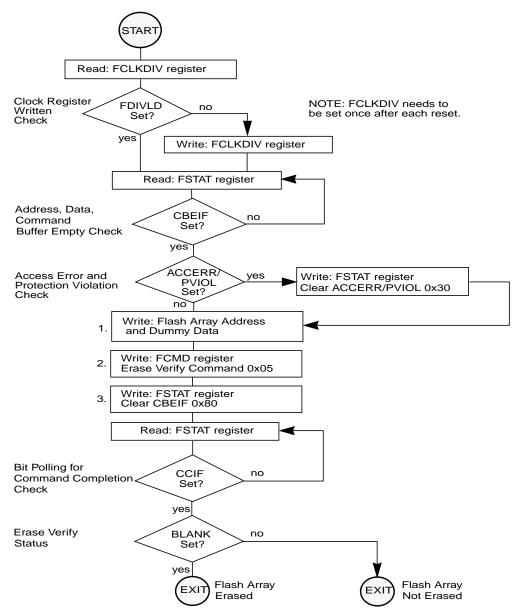
Figure 2-22. Example Erase Verify Command Flow
