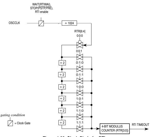
Figure 4-22. Clock Chain for RTI
