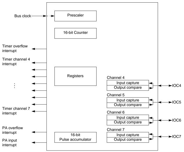
Figure 13-1. TIM16B4CV1 Block Diagram
