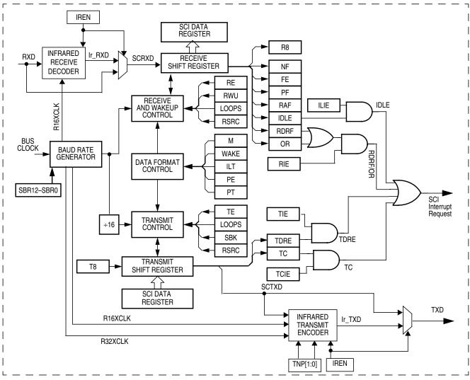
Figure 8-11. Detailed SCI Block Diagram
