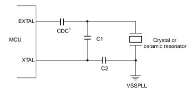
1. Due to the nature of a translated ground Colpitts oscillator a DC voltage bias is applied to the crystal. Please contact the crystal manufacturer for crystal DC
