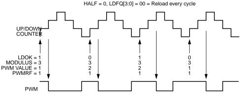
Figure 11-68. Full-Cycle Center-Aligned PWM Value Loading
