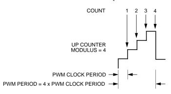
Figure 11-44. Edge-Aligned PWM Period
