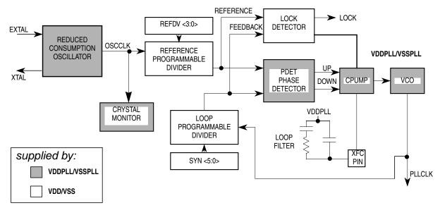
The VCO has a minimum operating frequency, which corresponds to the self-clock mode frequency f<sub>SCM</sub>.
