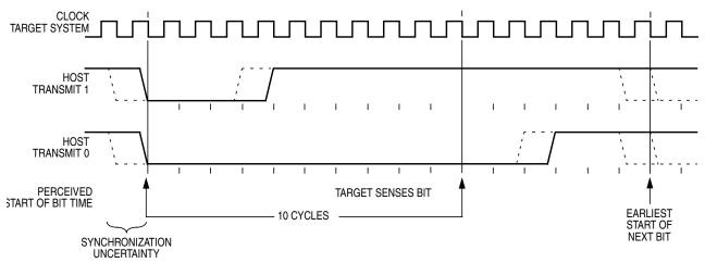
Figure 15-7. BDM Host-to-Target Serial Bit Timing
