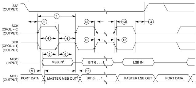
In Figure A-5 the timing diagram for master mode with transmission format CPHA=1 is depicted.
