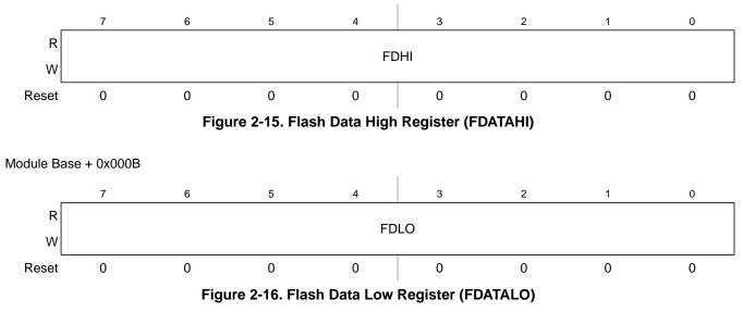
In normal modes, all FDATAHI and FDATALO bits read 0 and are not writable. In special modes, all FDATAHI and FDATALO bits are readable and writable when writing to an address within the Flash address range.
