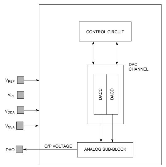
Figure 7-1. DAC8B1C Functional Block Diagram
