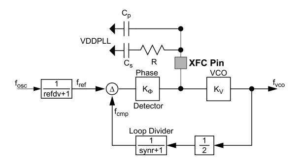
Figure A-2. Basic PLL functional diagram
