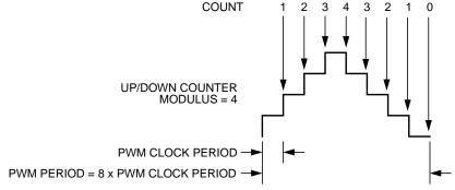
Figure 11-43. Center-Aligned PWM Period
