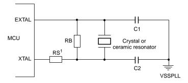
1. Rs can be zero (shorted) when use with higher frequency crystals. Refer to manufacturer's data.
