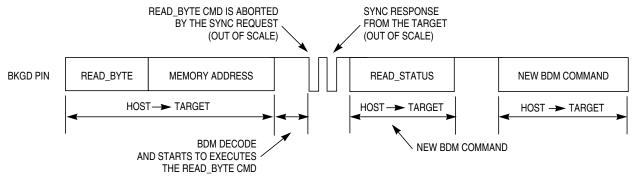
Figure 15-12. ACK Abort Procedure at the Command Level
