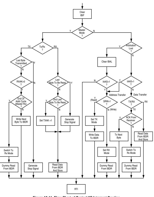
Figure 10-11. Flow-Chart of Typical IIC Interrupt Routine
