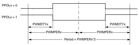
Figure 12-38. PWM Center Aligned Output Waveform
