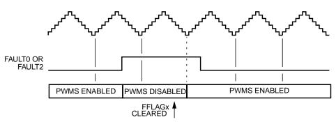
Figure 11-78. Manual Fault Clearing (Faults 0 & 2) - QSMP=01, 10, or 11
