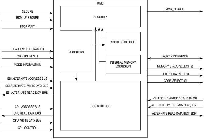
Figure 19-1. MMC Block Diagram
