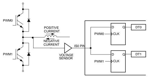
Figure 11-55. Current-Status Sense Scheme for Deadtime Correction
