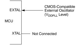
Figure 5-3. External Clock Connections (XCLKS = 1)
