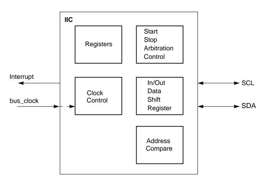
Figure 10-1. IIC Block Diagram
