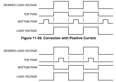
Figure 11-60. Correction with Negative Current
