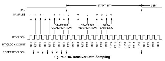
To verify the start bit and to detect noise, data recovery logic takes samples at RT3, RT5, and RT7. Table 8-14 summarizes the results of the start bit verification samples.
