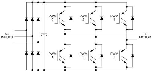
Figure 11-48. Typical 3 Phase AC Motor Drive
