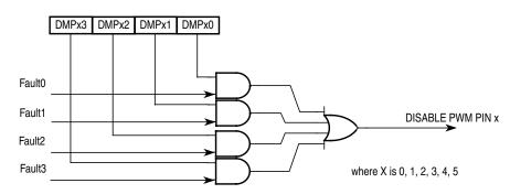
Figure 11-15. Fault Decoder
