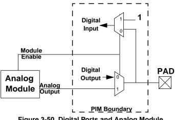
Figure 3-50. Digital Ports and Analog Module
