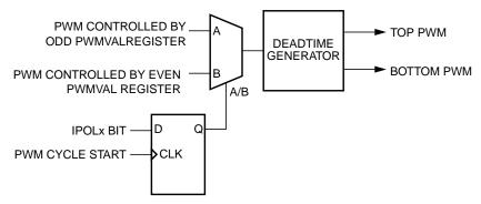
Figure 11-54. Internal Correction Logic when ISENS = 01
