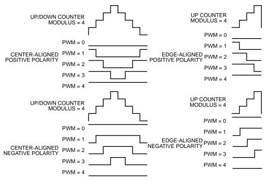
Figure 11-61. PWM Polarity
