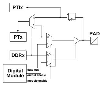
Figure 3-49. Illustration of I/O Pin Functionality
