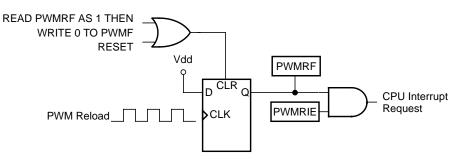
Figure 11-67. PWMRF Reload Interrupt Request
