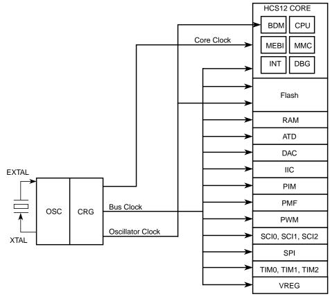
Figure 1-10. Clock Connections
