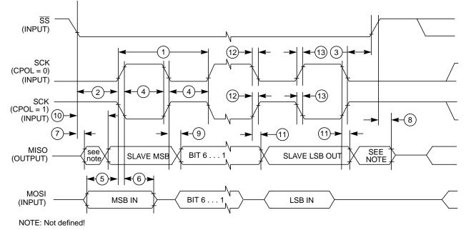
In Figure A-6 the timing diagram for slave mode with transmission format CPHA = 0 is depicted.
