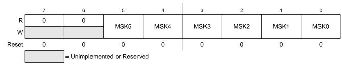
Figure 11-6. PMF Configure 2 Register (PMFCFG2)
