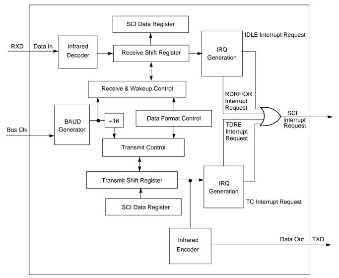
Figure 8-1. SCI Block Diagram
