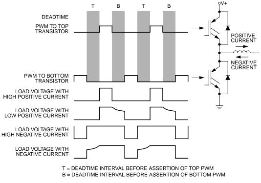
Figure 11-56. Output Voltage Waveforms
