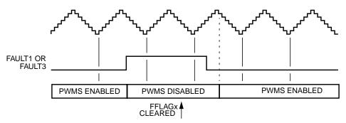
Figure 11-79. Manual Fault Clearing (Faults 1 & 3)
