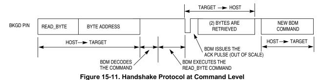
Differently from the normal bit transfer (where the host initiates the transmission), the serial interface ACK handshake pulse is initiated by the target MCU by issuing a falling edge in the BKGD pin. The hardware handshake protocol in Figure 15-10 specifies the timing when the BKGD pin is being driven, so the host
