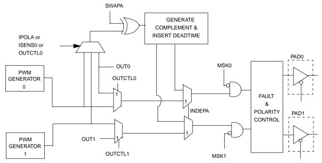
Figure 11-2. Detail of Mux, Swap, and Deadtime Functions
