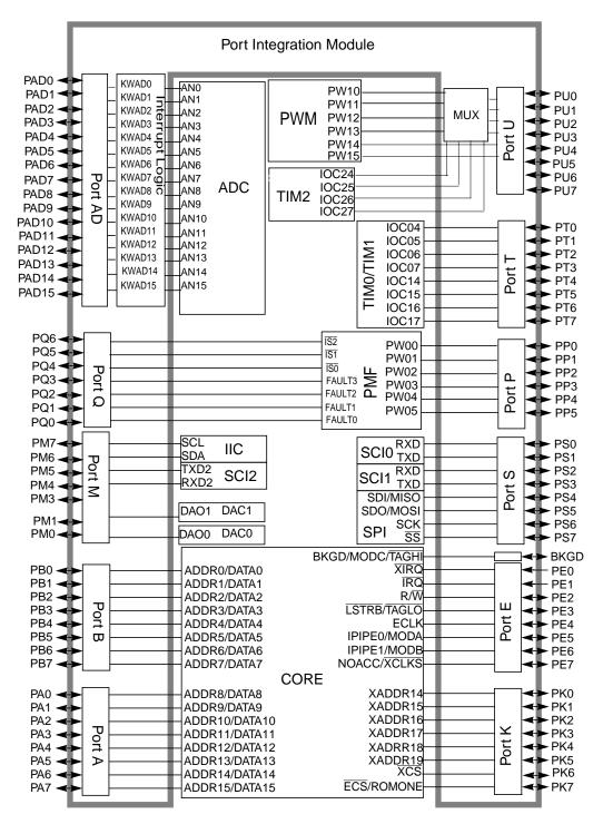
Figure 3-1. PIM9E128V1 Block Diagram
