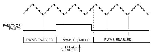
Figure 11-77. Manual Fault Clearing (Faults 0 & 2) — QSMP = 00
