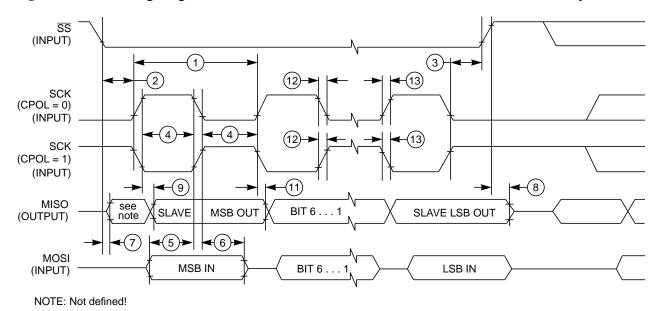
Figure A-7. SPI Slave Timing (CPHA = 1)
