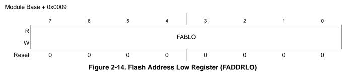
In normal modes, all FABHI and FABLO bits read 0 and are not writable. In special modes, the FABHI and FABLO bits are readable and writable. For sector erase, the MCU address bits [9:0] are ignored. For mass erase, any address within the Flash array is valid to start the command.
