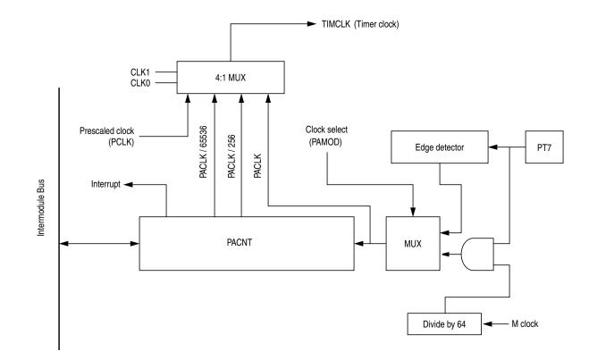
Figure 13-2. 16-Bit Pulse Accumulator Block Diagram
