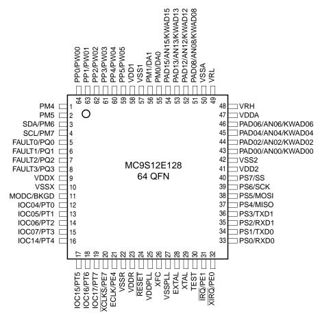
Figure 1-7. Pin Assignments for 64-QFN
