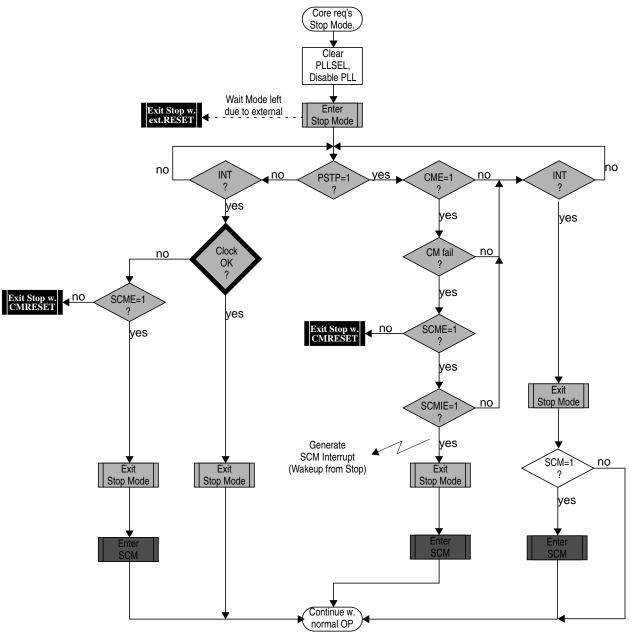
Figure 4-24. Stop Mode Entry/Exit Sequence
