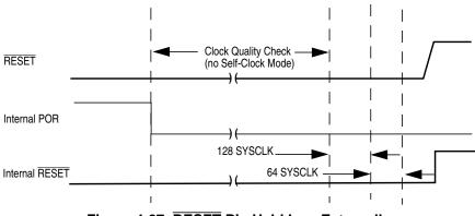
Figure 4-27. RESET Pin Held Low Externally
