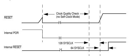
Figure 4-26. RESET Pin Tied to V<sub>DD</sub> (by a Pull-Up Resistor)
