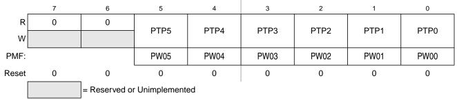
Figure 3-17. Port P I/O Register (PTP)
