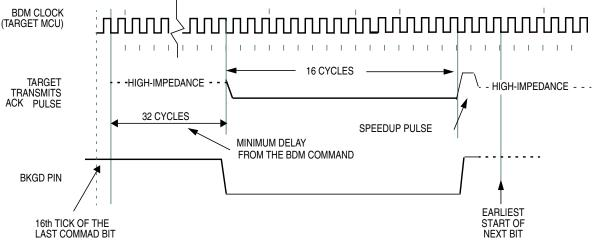
Figure 15-10. Target Acknowledge Pulse (ACK)
