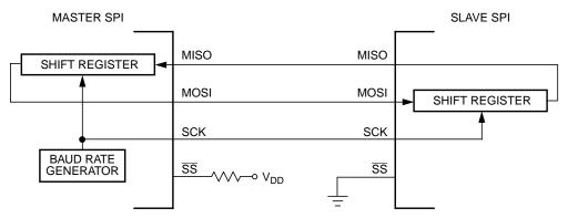
Figure 9-8. Master/Slave Transfer Block Diagram
