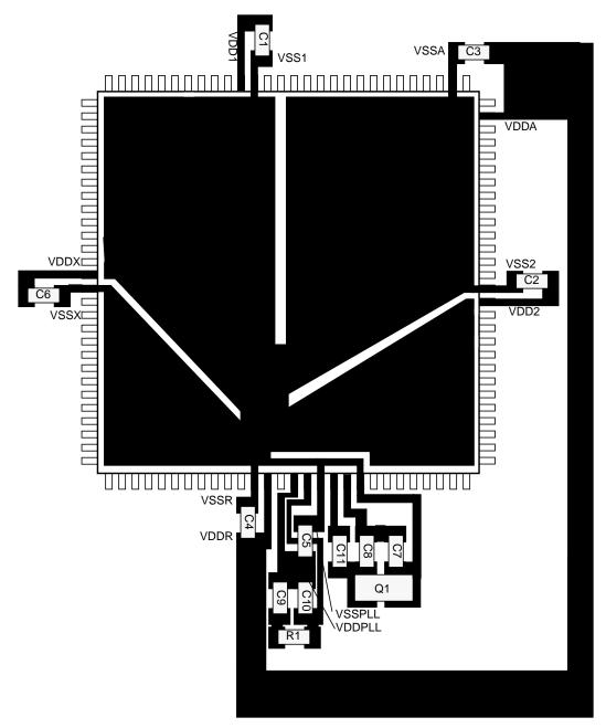
Figure 1-11. Recommended PCB Layout (112-LQFP)
