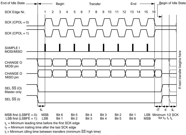
$t_L,\,t_T\!\!,$  and  $t_l$  are guaranteed for the master mode and required for the slave mode.
