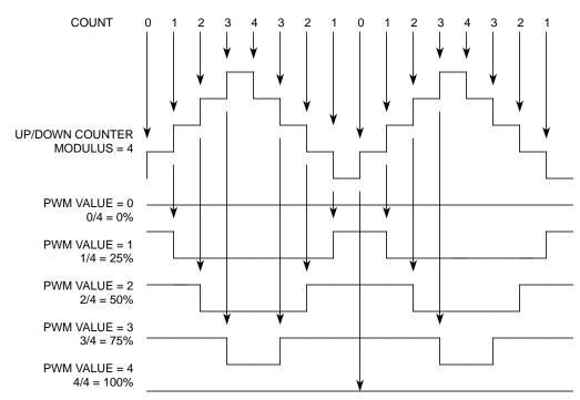
PWM pulse width = (PWM value)  $\times$  (PWM clock period)  $\times$  2
