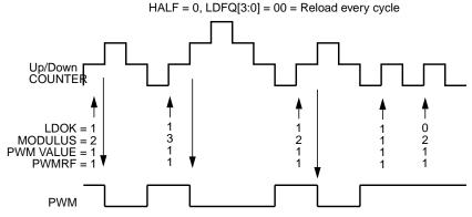
Figure 11-69. Full-Cycle Center-Aligned Modulus Loading
