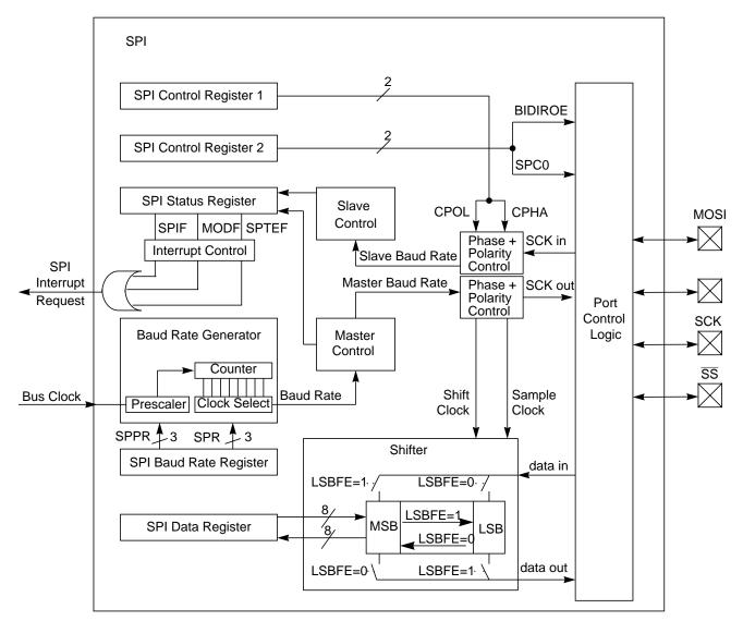
Figure 9-1. SPI Block Diagram
