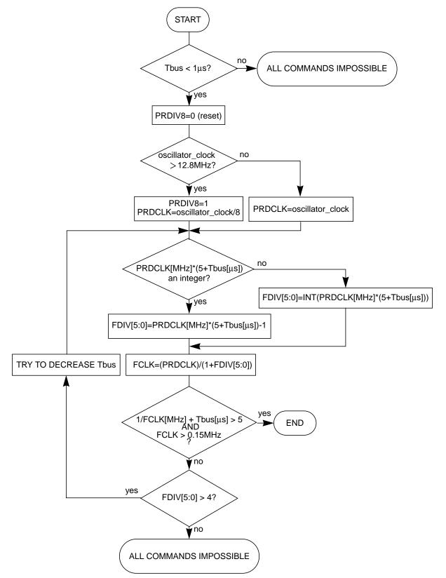
Figure 2-21. PRDIV8 and FDIV Bits Determination Procedure
