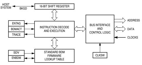
Figure 15-1. BDM Block Diagram
