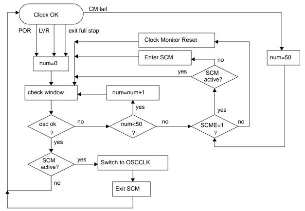
Figure 4-20. Sequence for Clock Quality Check
