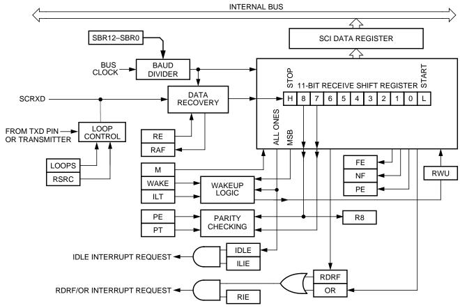
Figure 8-14. SCI Receiver Block Diagram
