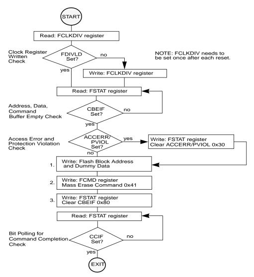
Figure 2-25. Example Mass Erase Command Flow
