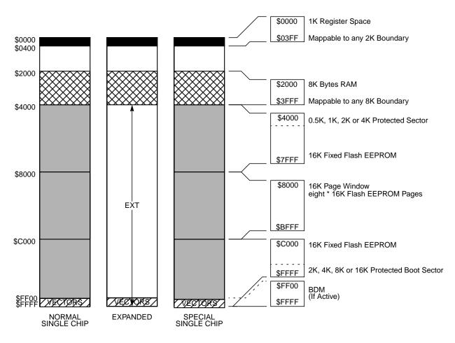
The figure shows a useful map, which is not the map out of reset. After reset the map is:
