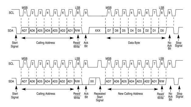
Figure 10-8. IIC-Bus Transmission Signals
