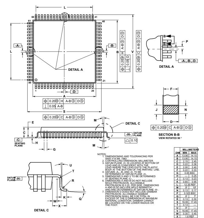
Figure B-2. 80-Pin QFP Mechanical Dimensions (Case no. 841B)
