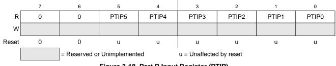
Figure 3-18. Port P Input Register (PTIP)
