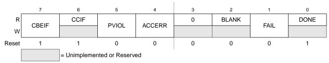
Figure 2-10. Flash Status Register (FSTAT)
