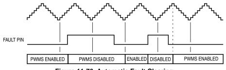
Figure 11-76. Automatic Fault Clearing
