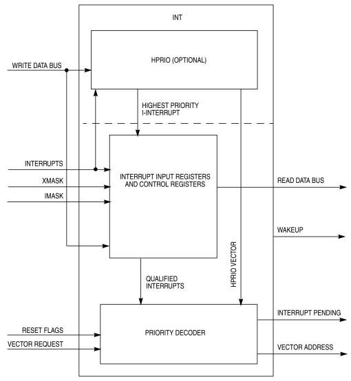
Figure 17-1. INTV1 Block Diagram
