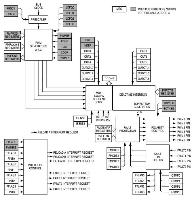
Figure 11-1. PMF Block Diagram
