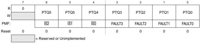
Figure 3-23. Port Q I/O Register (PTQ)
