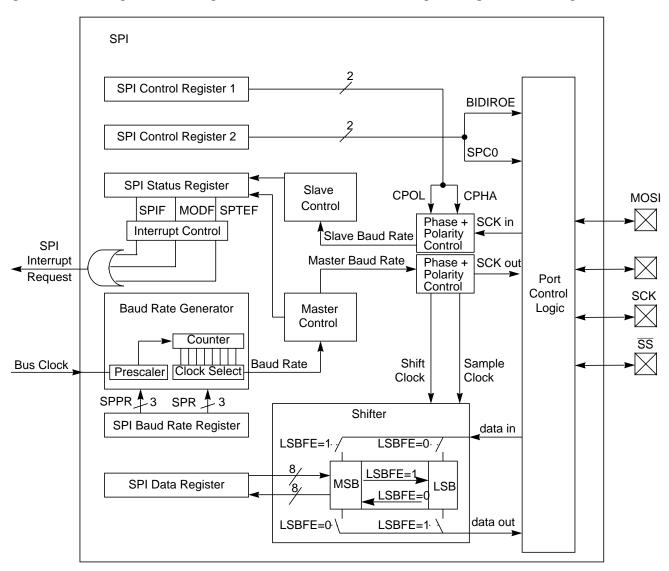
Figure 9-1. SPI Block Diagram
