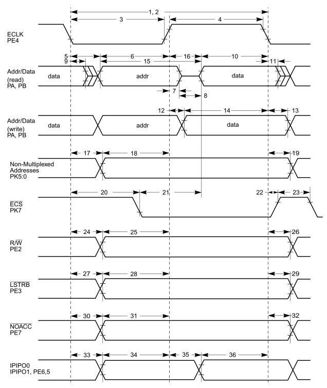
Figure A-10. General External Bus Timing
