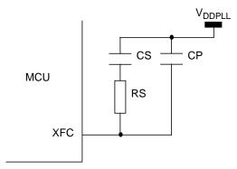
Figure 4-2. PLL Loop Filter Connections
