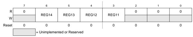
Figure 19-4. Initialization of Internal Registers Position Register (INITRG)
