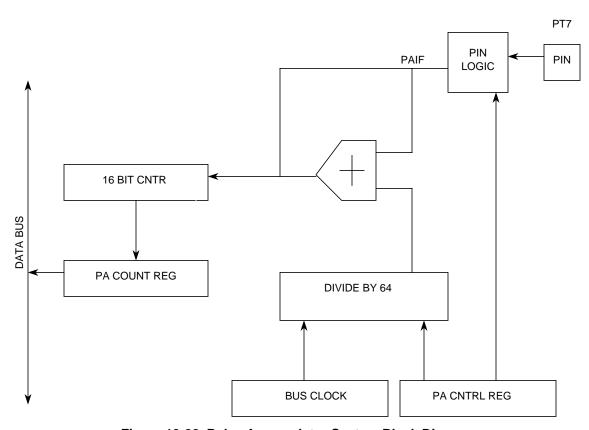
Figure 13-22. Pulse Accumulator System Block Diagram
