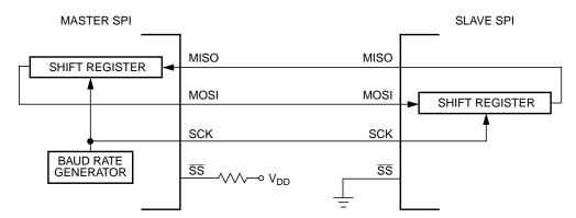
Figure 9-8. Master/Slave Transfer Block Diagram
