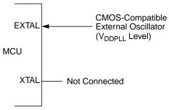
Figure 5-3. External Clock Connections (XCLKS = 1)
