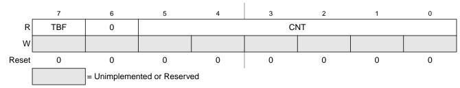
Figure 16-8. Debug Count Register (DBGCNT)
