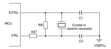
Rs can be zero (shorted) when use with higher frequency crystals.
