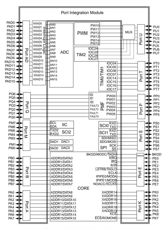
Figure 3-1. PIM9E256V1 Block Diagram
