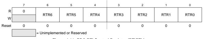
Figure 4-11. CRG RTI Control Register (RTICTL)
