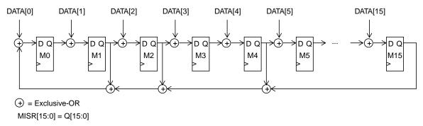
Figure 2-25. 16-Bit MISR Diagram
