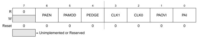
Figure 13-17. 16-Bit Pulse Accumulator Control Register (PACTL)
