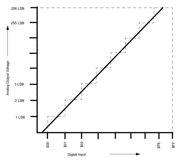
1 LSB = 21.5 mV when  $V_{DDA}$  = 5.5 V
