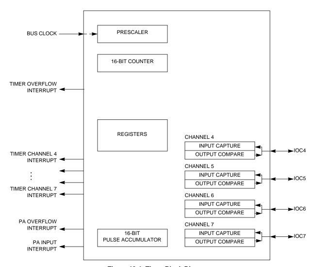
Figure 13-1. Timer Block Diagram
