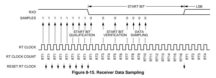
To verify the start bit and to detect noise, data recovery logic takes samples at RT3, RT5, and RT7. Table 8-15 summarizes the results of the start bit verification samples.
