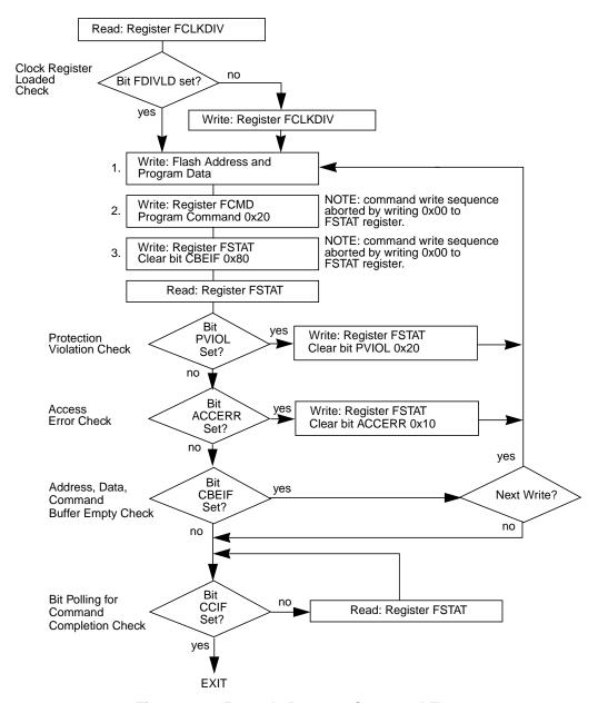
Figure 2-26. Example Program Command Flow
