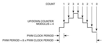
Figure 11-43. Center-Aligned PWM Period
