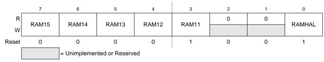
Figure 19-3. Initialization of Internal RAM Position Register (INITRM)
