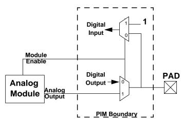
Figure 3-50. Digital Ports and Analog Module
