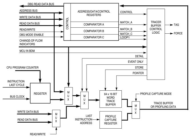
Figure 16-2. DBG Block Diagram in DBG Mode
