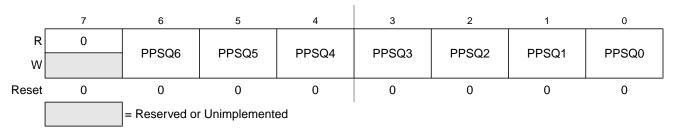
Figure 3-28. Port Q Polarity Select Register (PPSQ)
