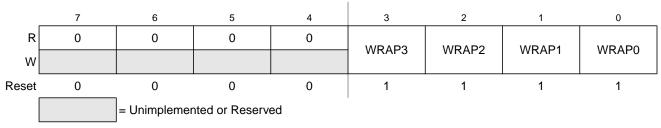
Figure 6-3. ATD Control Register 0 (ATDCTL0)
