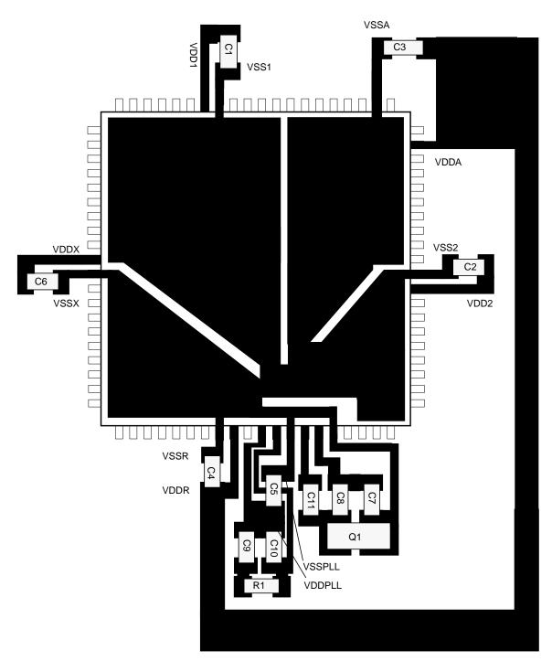
Figure 1-9. Recommended PCB Layout (80-QFP)
