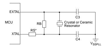
\* Rs can be zero (shorted) when used with higher frequency crystals. Refer to manufacturer's data.
