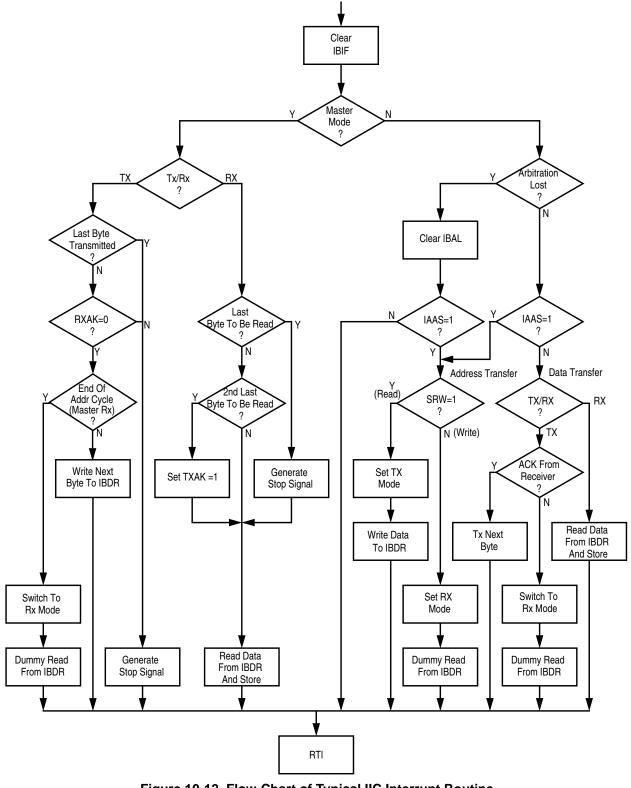
Figure 10-12. Flow-Chart of Typical IIC Interrupt Routine
