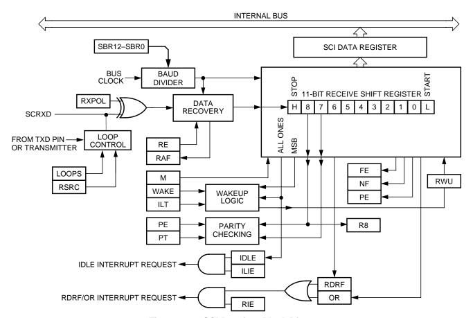
Figure 8-14. SCI Receiver Block Diagram
