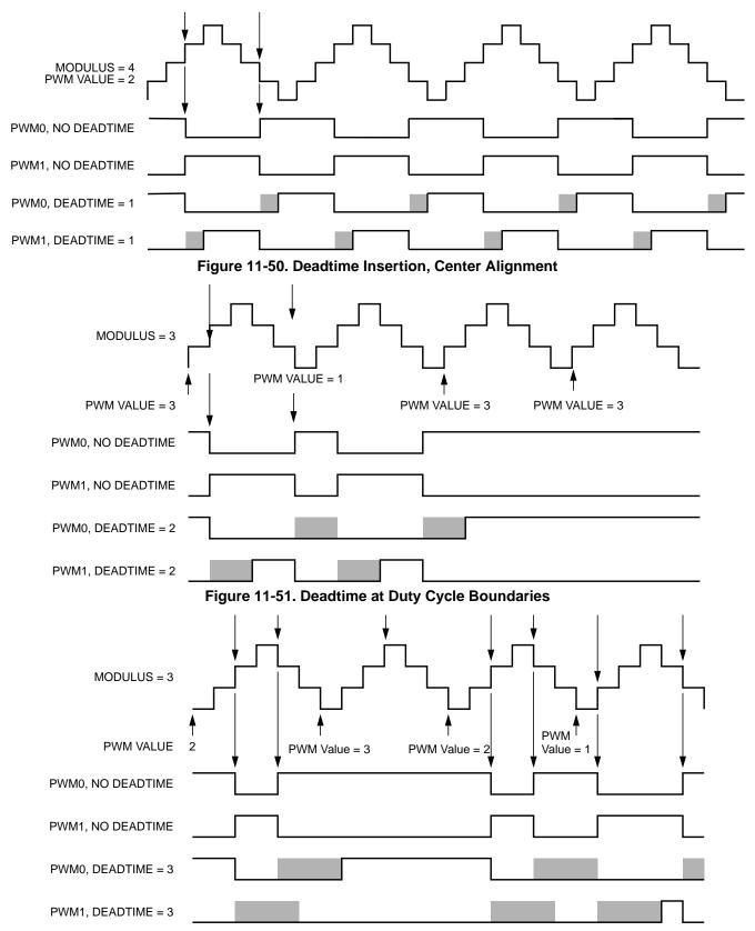
Figure 11-52. Deadtime and Small Pulse Widths
