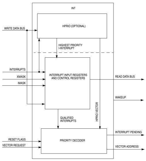
Figure 17-1. INTV1 Block Diagram
