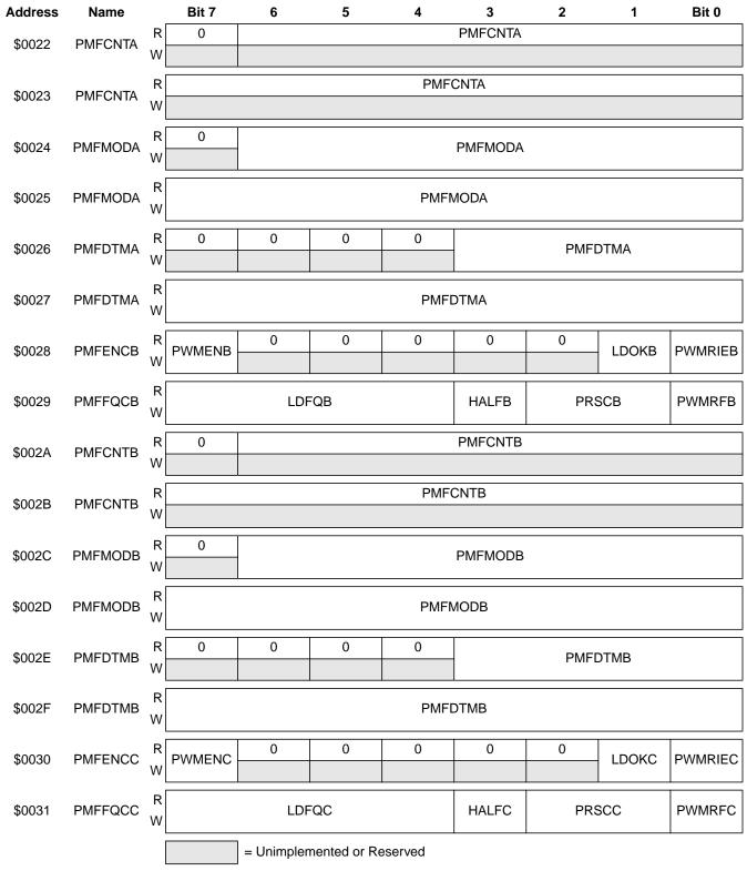
Figure 11-3. Quick Reference to PMF Registers (Sheet 3 of 4)
