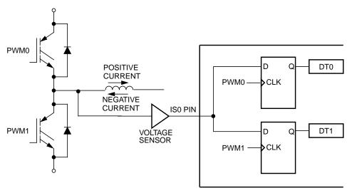
Figure 11-55. Current Status Sense Scheme for Deadtime Correction
