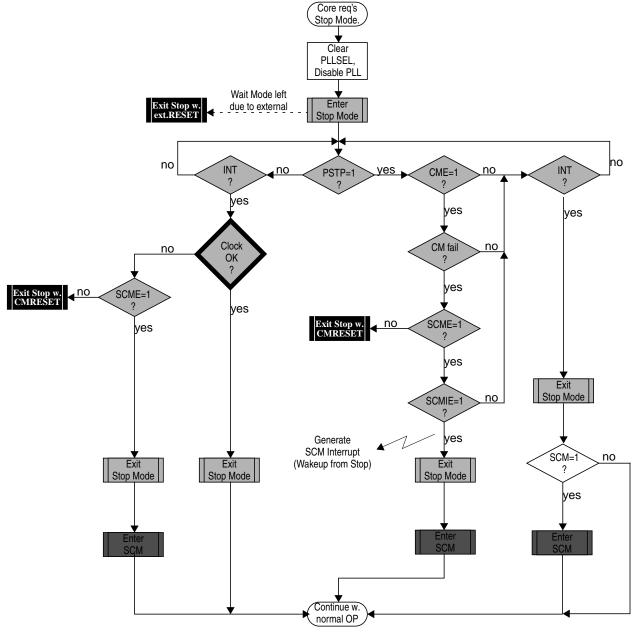
Figure 4-24. Stop Mode Entry/Exit Sequence
