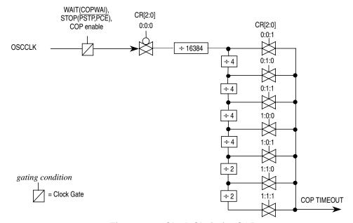
Figure 4-21. Clock Chain for COP
