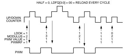
Figure 11-69. Full-Cycle Center-Aligned Modulus Loading
