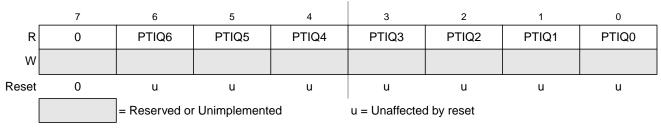
Figure 3-24. Port Q Input Register (PTIQ)
