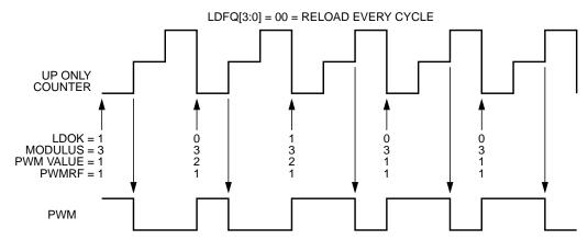
Figure 11-72. Edge-Aligned PWM Value Loading
