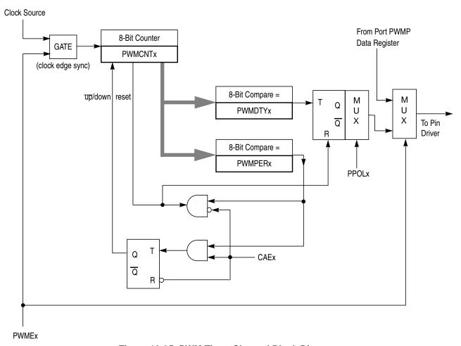
Figure 12-35. PWM Timer Channel Block Diagram
