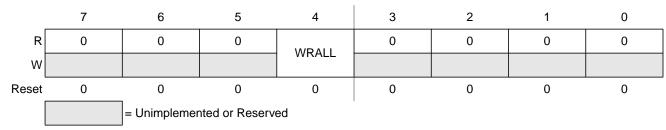
Figure 2-6. Flash Test Mode Register (FTSTMOD)
