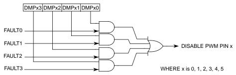
Figure 11-15. Fault Decoder
