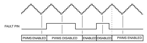
Figure 11-76. Automatic Fault Clearing
