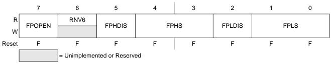
Figure 2-8. Flash Protection Register (FPROT)
