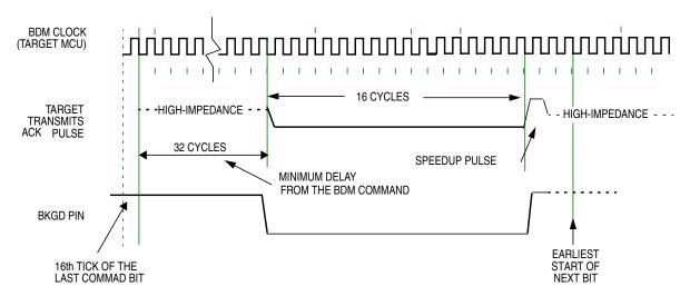
Figure 15-10. Target Acknowledge Pulse (ACK)
