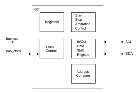
Figure 10-1. IIC Block Diagram
