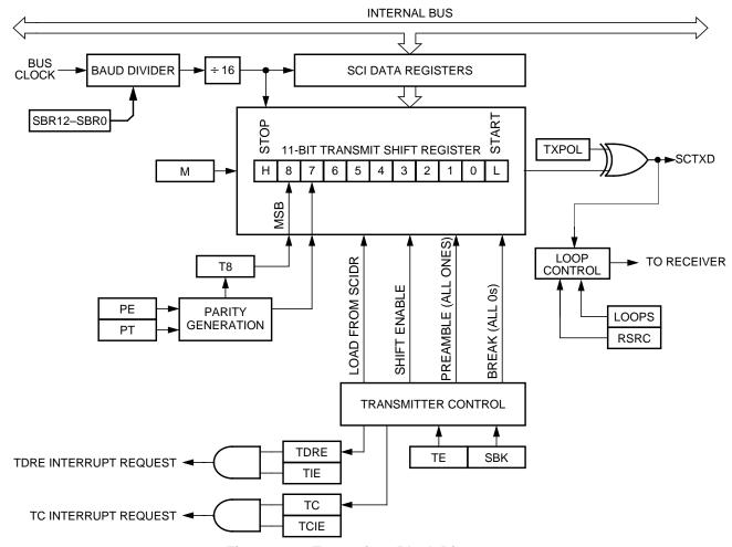
Figure 8-13. Transmitter Block Diagram
