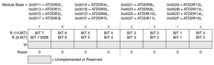
Figure 6-21. Right Justified, ATD Conversion Result Register x, Low Byte (ATDDRxL)
