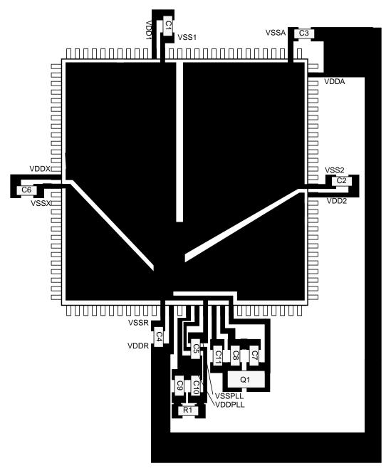
Figure 1-8. Recommended PCB Layout (112-LQFP)
