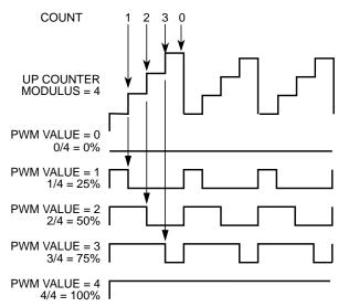
Figure 11-46. Edge-Aligned PWM Pulse Width
