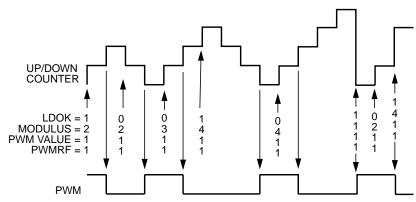
Figure 11-71. Half-Cycle Center-Aligned Modulus Loading
