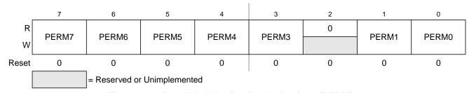
Figure 3-14. Port M Pull Device Enable Register (PERM)
