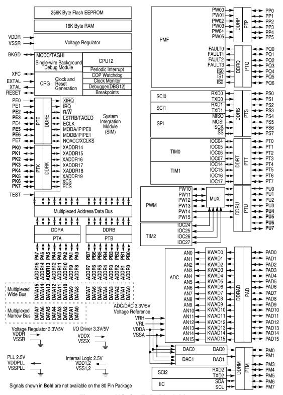
Figure 1-1. MC9S12E256 Block Diagram
