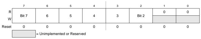
Figure 18-11. Data Direction Register E (DDRE)
