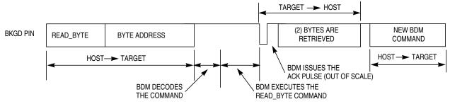
Figure 15-11. Handshake Protocol at Command Level
