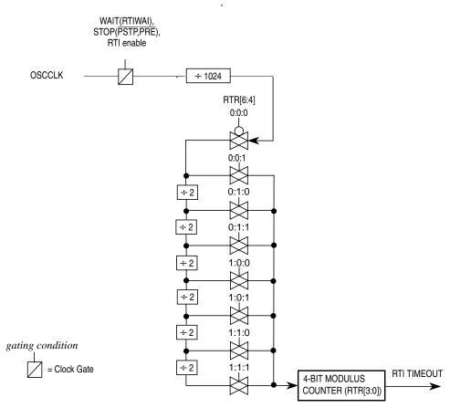
Figure 4-22. Clock Chain for RTI
