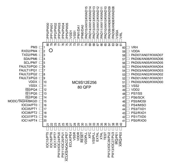
Figure 1-4. Pin Assignments for 80-QFP
