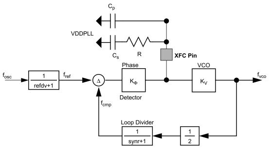
Figure A-2. Basic PLL Functional Diagram
