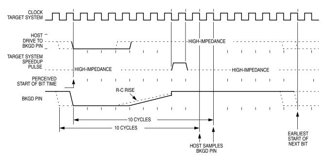
Figure 15-8. BDM Target-to-Host Serial Bit Timing (Logic 1)
