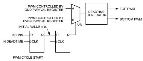
Figure 11-57. Internal Correction Logic when ISENS = 10
