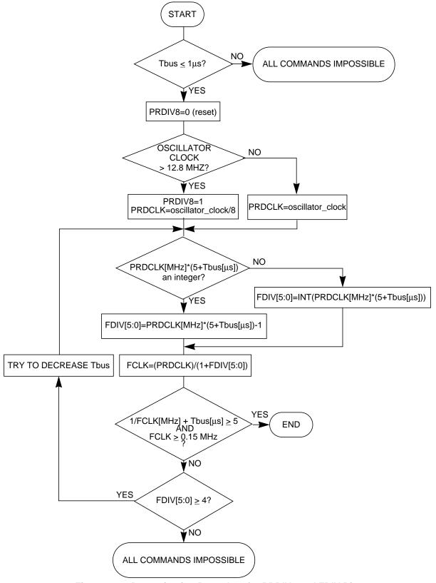
Figure 2-22. Determination Procedure for PRDIV8 and FDIV Bits
