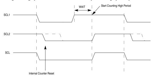
Figure 10-11. IIC-Bus Clock Synchronization
