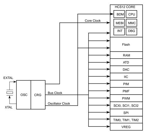
Figure 1-7. Clock Connections
