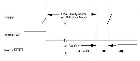
Figure 4-26. RESET Pin Tied to V<sub>DD</sub> (by a Pull-Up Resistor)
