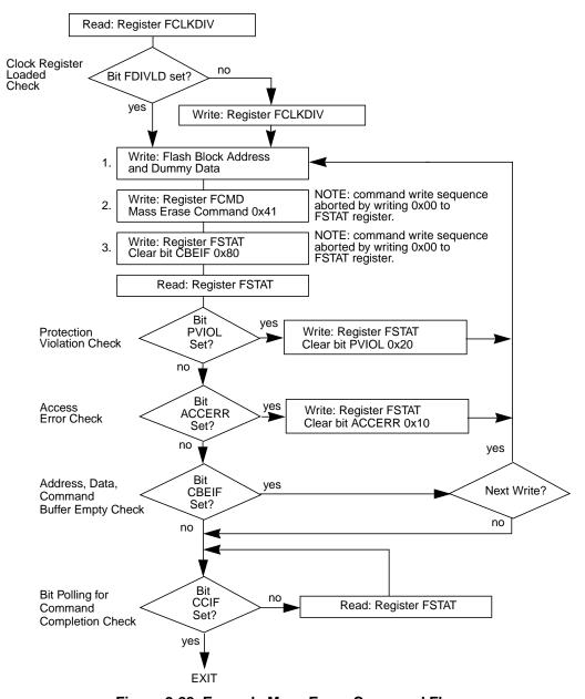
Figure 2-28. Example Mass Erase Command Flow
