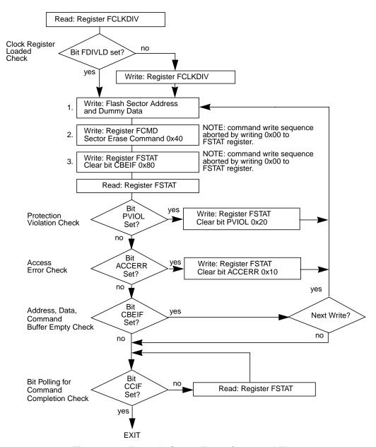
Figure 2-27. Example Sector Erase Command Flow
