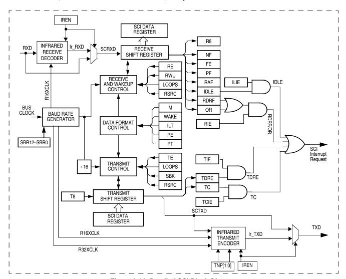
Figure 8-11. Detailed SCI Block Diagram
