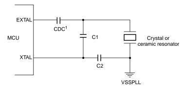
Due to the nature of a translated ground Colpitts oscillator a DC voltage bias is applied to the crystal. Please contact the crystal manufacturer for crystal DC
