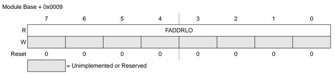
Figure 2-15. Flash Address Low Register (FADDRLO)
