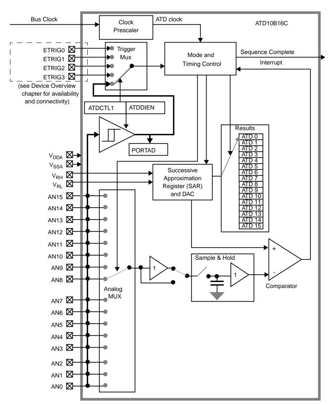
Figure 6-1. ATD10B16C Block Diagram
