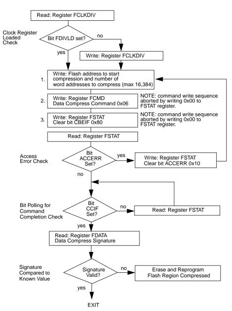
Figure 2-24. Example Data Compress Command Flow
