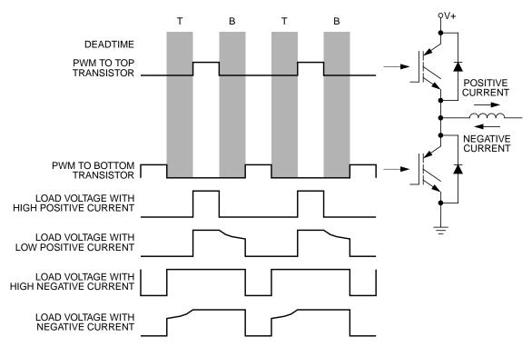
T = DEADTIME INTERVAL BEFORE ASSERTION OF TOP PWM B = DEADTIME INTERVAL BEFORE ASSERTION OF BOTTOM PWM
