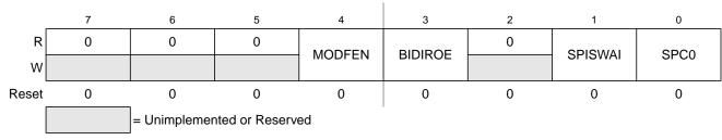
Figure 9-4. SPI Control Register 2 (SPICR2)
