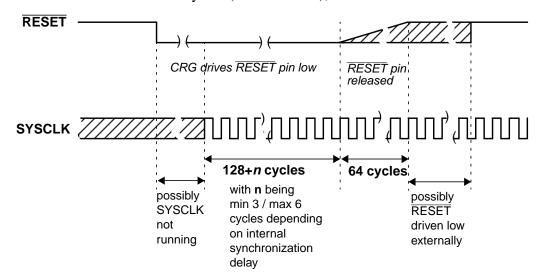
Figure 4-25. RESET Timing
