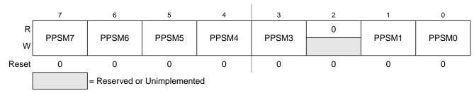
Figure 3-15. Port M Polarity Select Register (PPSM)
