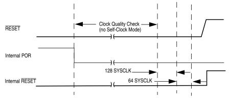
Figure 4-27. RESET Pin Held Low Externally
