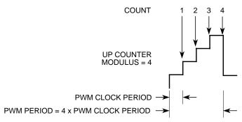
Figure 11-44. Edge-Aligned PWM Period
