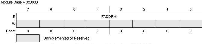
Figure 2-14. Flash Address High Register (FADDRHI)
