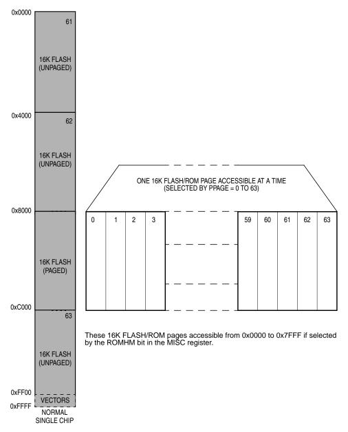
Figure 19-12. Memory Paging Example: 1M Byte On-Chip FLASH/ROM, 64K Allocation
