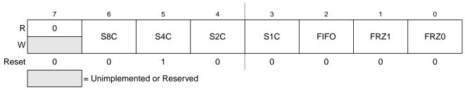
Figure 7-6. ATD Control Register 3 (ATDCTL3)
