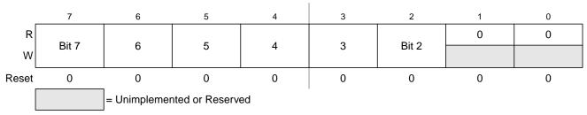
Figure 18-11. Data Direction Register E (DDRE)
