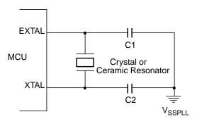
Figure 6-2. Loop Controlled Pierce Oscillator Connections (XCLKS = 0)
