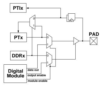
Figure 4-47. Illustration of I/O Pin Functionality
