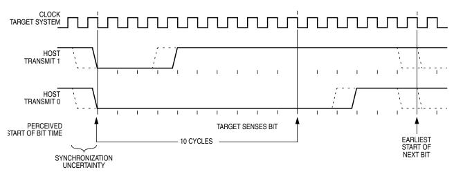
Figure 15-7. BDM Host-to-Target Serial Bit Timing
