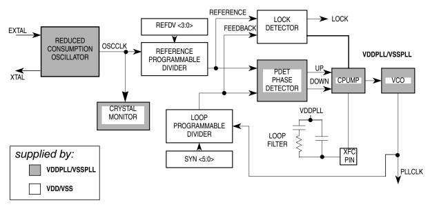
Figure 5-16. PLL Functional Diagram
