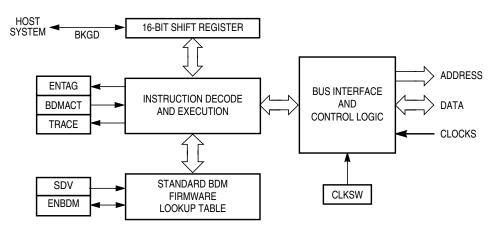
Figure 15-1. BDM Block Diagram
