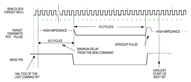
Figure 15-10. Target Acknowledge Pulse (ACK)
