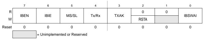
Figure 8-6. IIC Bus Control Register (IBCR)
