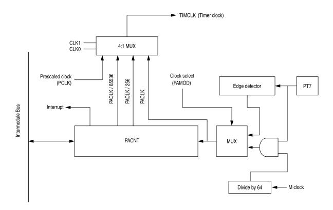
Figure 13-2. 16-Bit Pulse Accumulator Block Diagram
