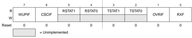
Figure 9-8. MSCAN Receiver Flag Register (CANRFLG)
