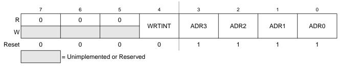
Figure 17-2. Interrupt Test Control Register (ITCR)
