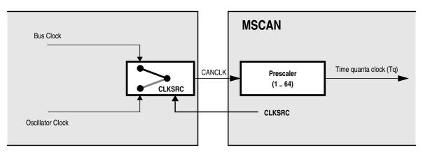
Figure 9-42. MSCAN Clocking Scheme
