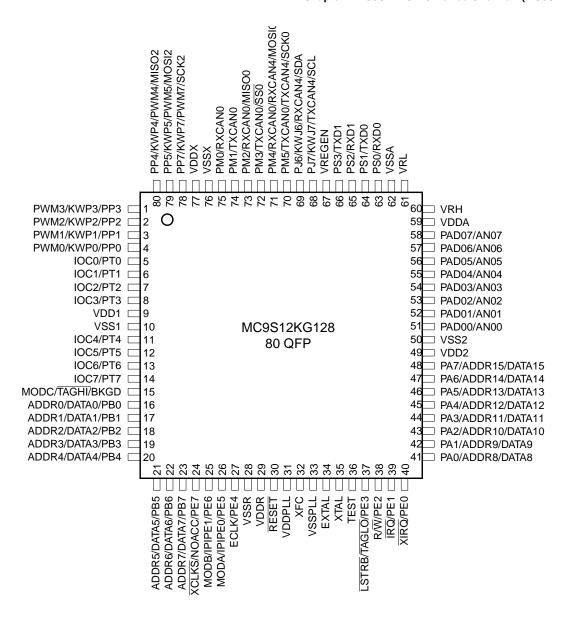
Figure 1-4. Pin Assignments for 80 QFP
