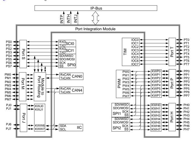
Figure 4-1. PIM9KG128 Block Diagram
