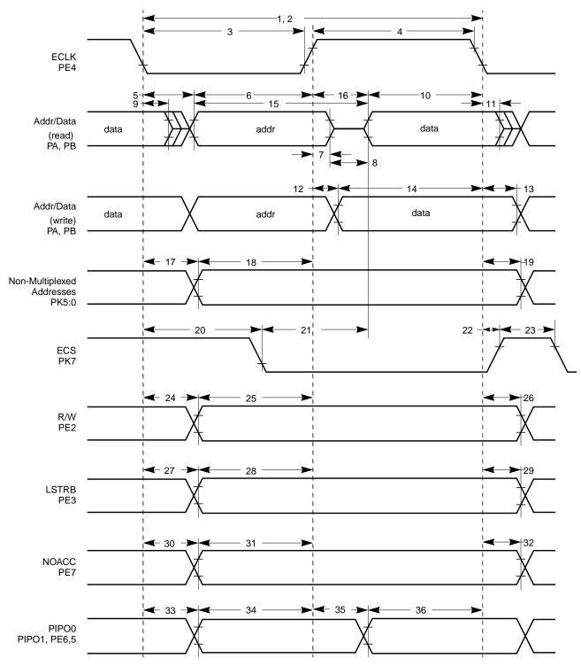
Figure A-9. General External Bus Timing
