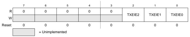
Figure 9-11. MSCAN Transmitter Interrupt Enable Register (CANTIER)
