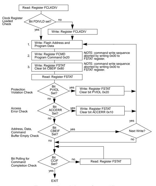
Figure 2-27. Example Program Command Flow
