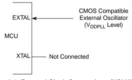
Figure 6-4. External Clock Connections (XCLKS = 1)
