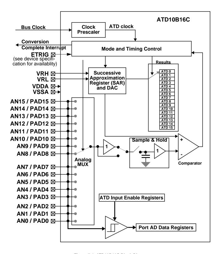
Figure 7-1. ATD10B16C Block Diagram
