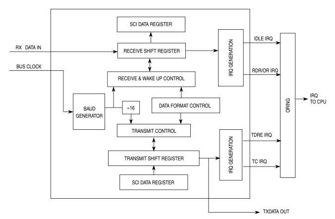
Figure 10-1. SCI Block Diagram
