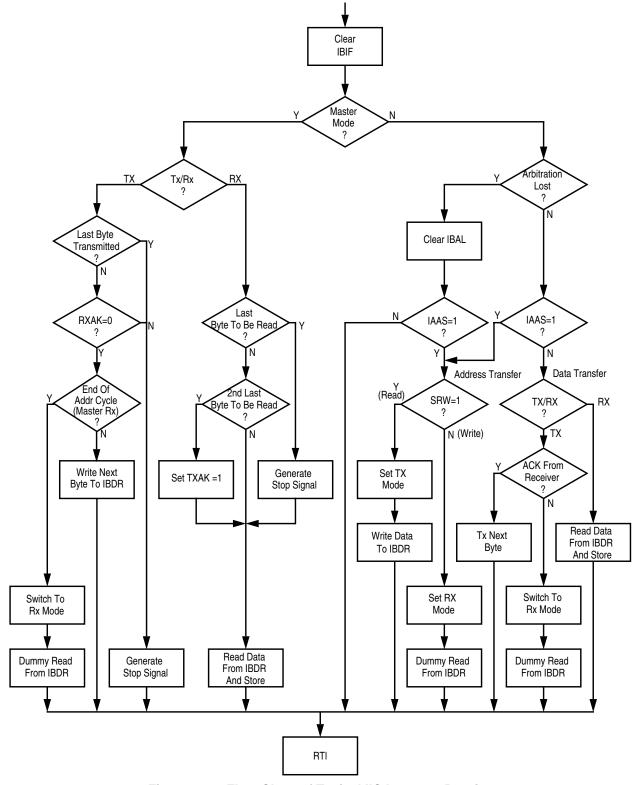
Figure 8-12. Flow-Chart of Typical IIC Interrupt Routine
