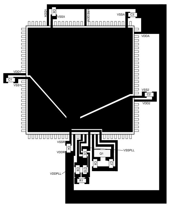
Figure B-1. Recommended PCB Layout for 112LQFP
