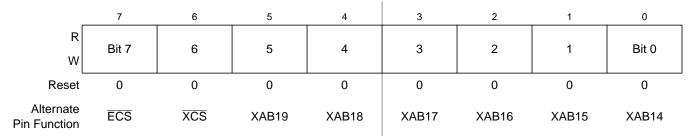
Figure 18-19. Port K Data Register (PORTK)
