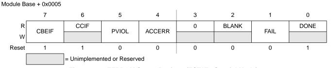
Figure 3-10. EEPROM Status Register (ESTAT - Special Mode)
