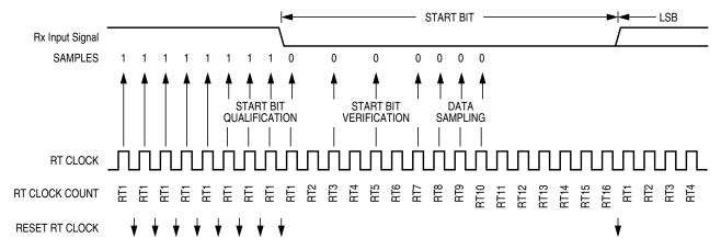
Figure 10-13. Receiver Data Sampling
