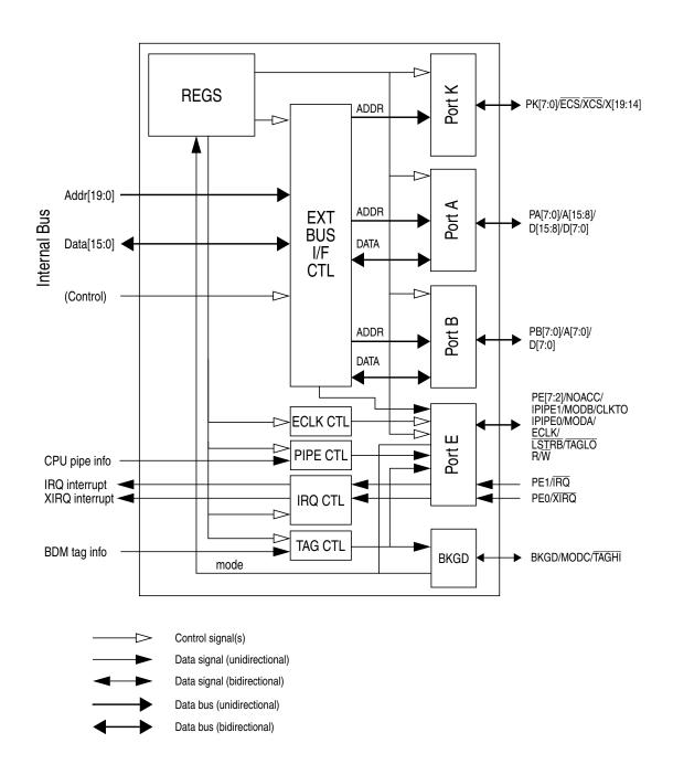
Figure 18-1. MEBI Block Diagram
