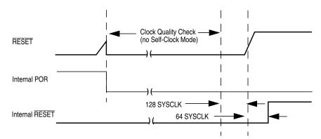
Figure 5-26. RESET Pin Tied to V<sub>DD</sub> (by a Pull-Up Resistor)
