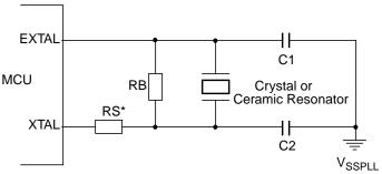
$<sup>^{\</sup>ast}$  R  $_{\!S}$  can be zero (shorted) when use with higher frequency crystals. Refer to manufacturer's data.
