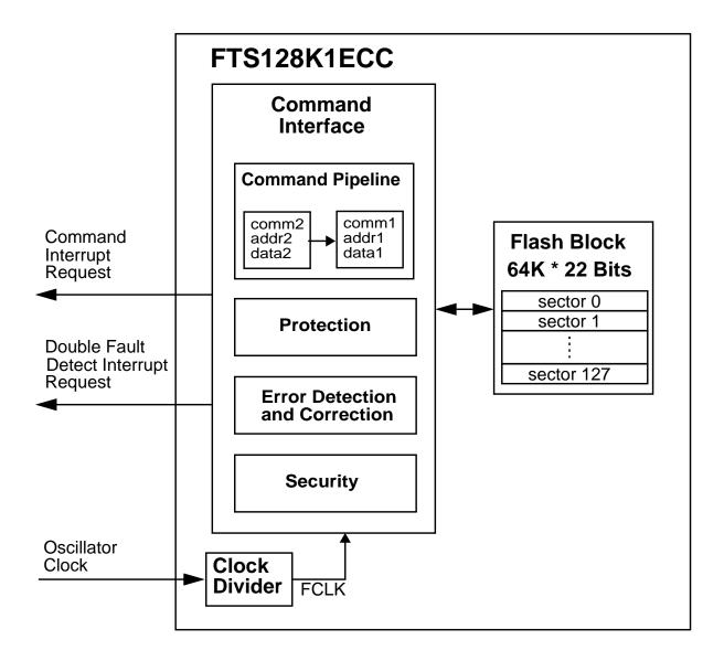
Figure 2-1. FTS128K1ECC Block Diagram
