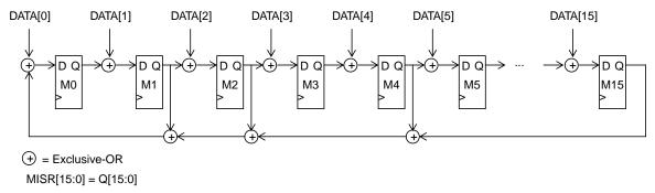
Figure 2-26. 16-Bit MISR Diagram
