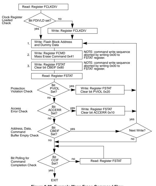
Figure 2-29. Example Mass Erase Command Flow
