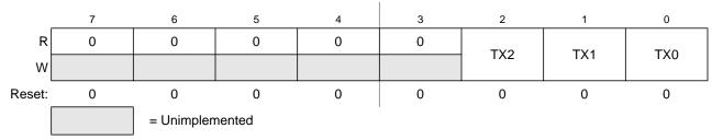
Figure 9-14. MSCAN Transmit Buffer Selection Register (CANTBSEL)
