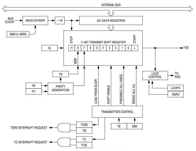
Figure 10-11. Transmitter Block Diagram
