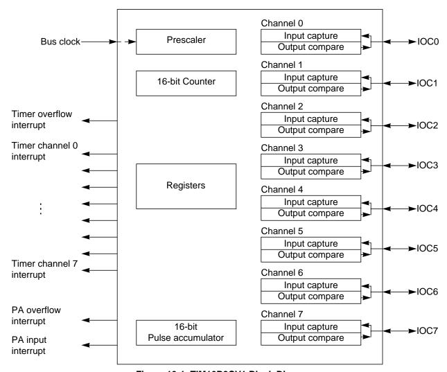
Figure 13-1. TIM16B8CV1 Block Diagram
