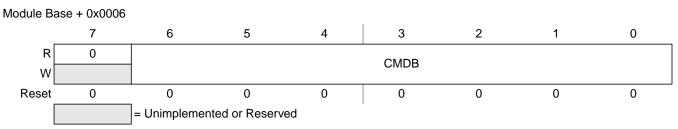
Figure 2-11. Flash Command Register (FCMD - NVM User Mode)
