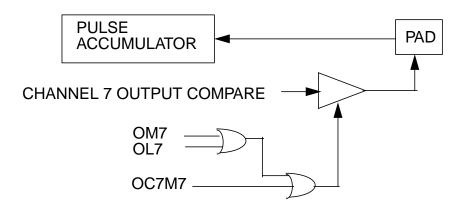
Figure 13-4. Channel 7 Output Compare/Pulse Accumulator Logic
