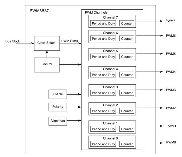
Figure 12-1. PWM Block Diagram
