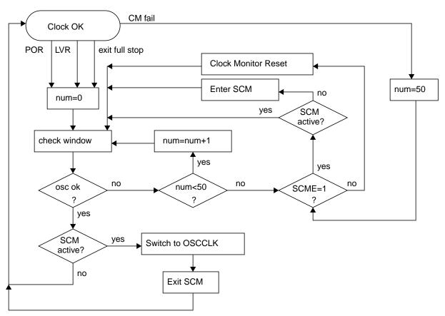
Figure 5-20. Sequence for Clock Quality Check
