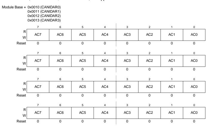
Figure 9-19. MSCAN Identifier Acceptance Registers (First Bank) — CANIDAR0-CANIDAR3
