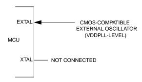
Figure 1-8. External Clock Connections (PE7 = 0)
