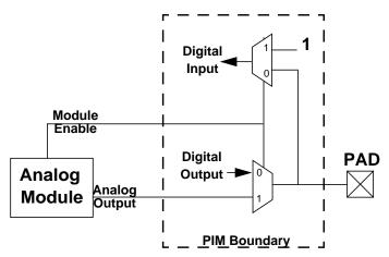
Figure 4-48. Digital Ports and Analog Module
