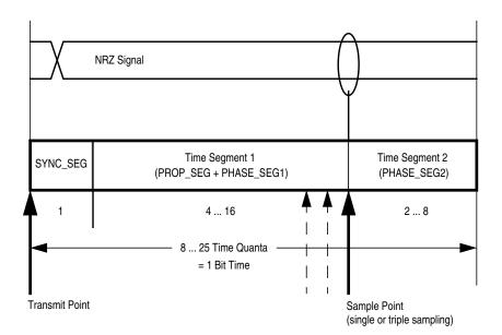
Figure 9-43. Segments within the Bit Time
