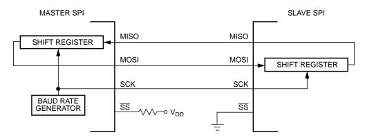
Figure 11-8. Master/Slave Transfer Block Diagram
