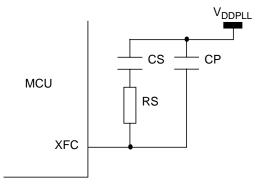
Figure 5-2. PLL Loop Filter Connections
