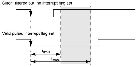
Figure 4-50. Interrupt Glitch Filter (PPS = 0)
