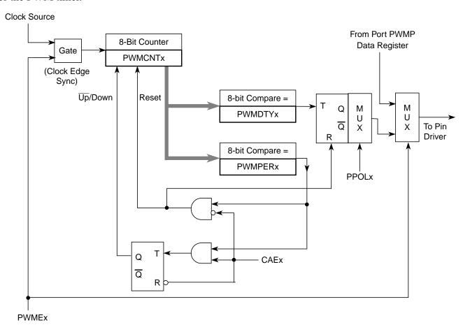
Figure 12-19. PWM Timer Channel Block Diagram
