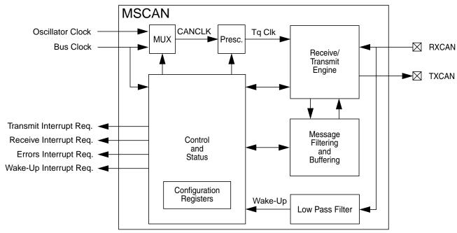
Figure 9-1. MSCAN Block Diagram
