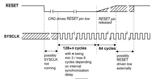
Figure 5-25. RESET Timing
