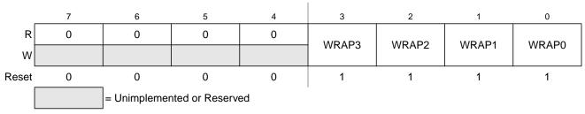
Figure 7-3. ATD Control Register 0 (ATDCTL0)
