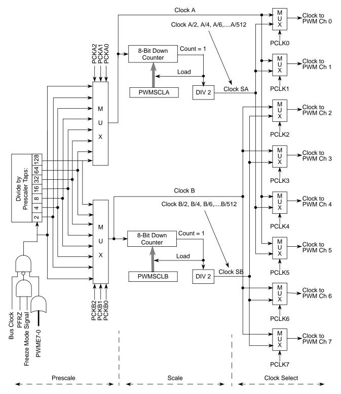
Figure 12-18. PWM Clock Select Block Diagram
