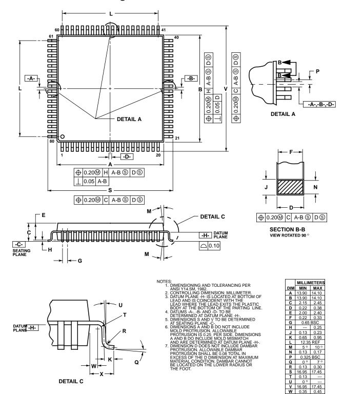
Figure C-2. 80-Pin QFP Mechanical Dimensions (Case no. 841B)
