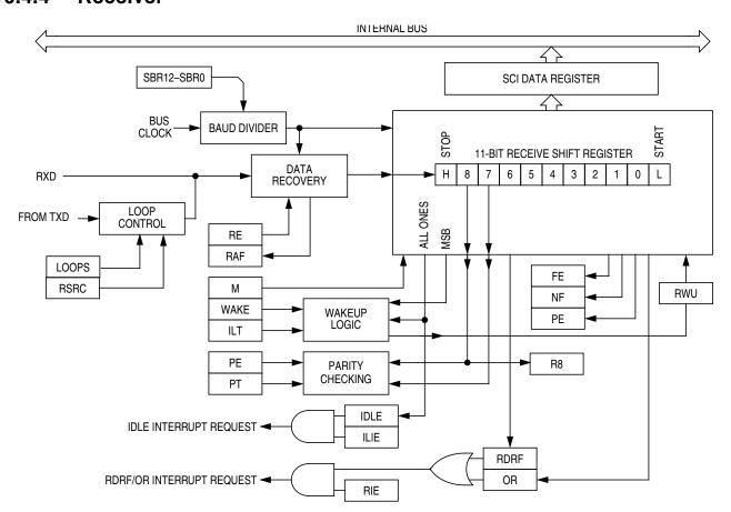
Figure 10-12. SCI Receiver Block Diagram
