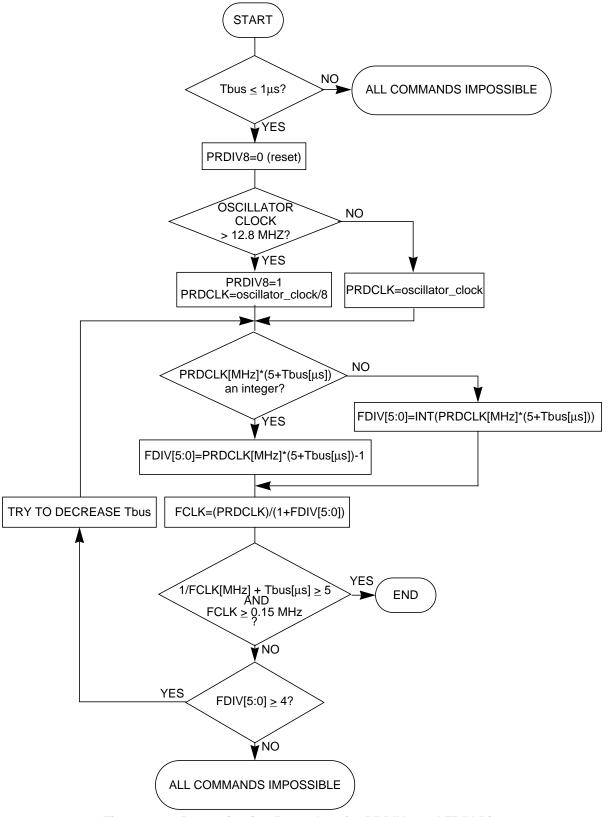
Figure 2-23. Determination Procedure for PRDIV8 and FDIV Bits
