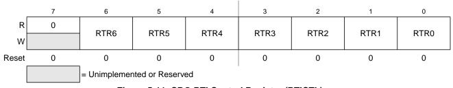
Figure 5-11. CRG RTI Control Register (RTICTL)
