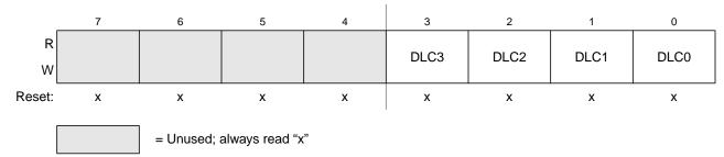
Figure 9-34. Data Length Register (DLR) — Extended Identifier Mapping
