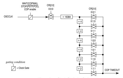
Figure 5-21. Clock Chain for COP
