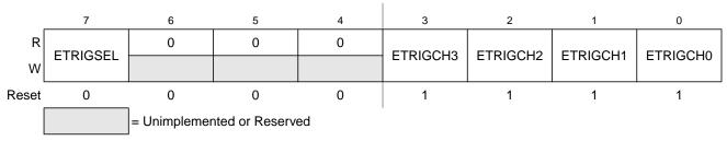
Figure 7-4. ATD Control Register 1 (ATDCTL1)
