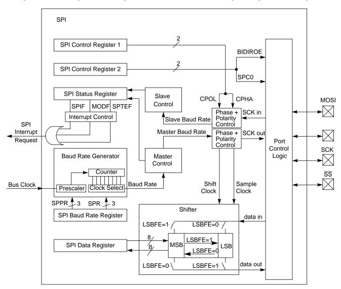
Figure 11-1. SPI Block Diagram
