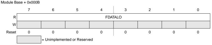
Figure 2-18. Flash Data Low Register (FDATALO)
