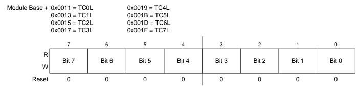
Figure 13-23. Timer Input Capture/Output Compare Register x Low (TCxL)
