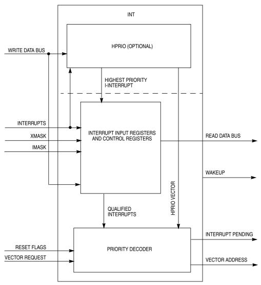
Figure 17-1. INTV1 Block Diagram
