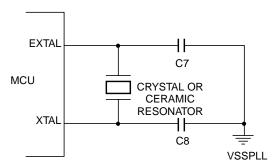
Figure 1-6. Loop Controlled Pierce Oscillator Connections (PE7 = 1)
