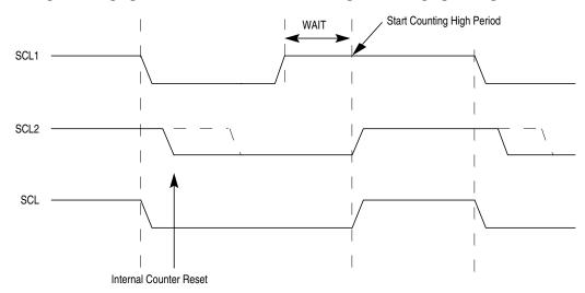
Figure 8-11. IIC-Bus Clock Synchronization
