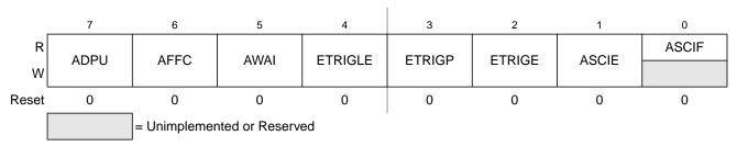
Figure 7-5. ATD Control Register 2 (ATDCTL2)
