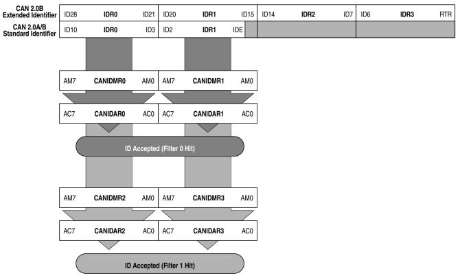
Figure 9-40. 16-bit Maskable Identifier Acceptance Filters
