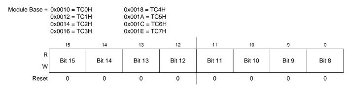
Figure 13-22. Timer Input Capture/Output Compare Register x High (TCxH)
