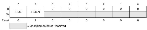
Figure 18-18. IRQ Control Register (IRQCR)
