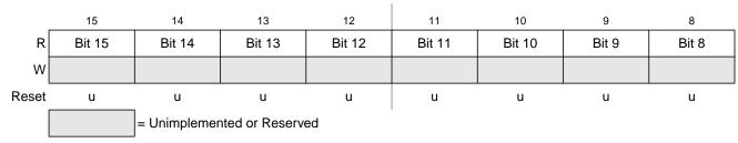
Figure 16-6. Debug Trace Buffer Register High (DBGTBH)
