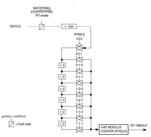
Figure 5-22. Clock Chain for RTI
