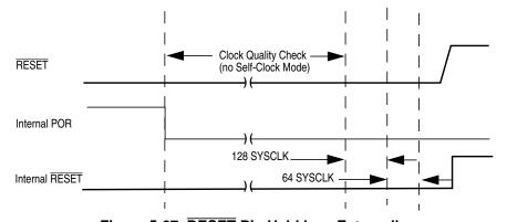
Figure 5-27. RESET Pin Held Low Externally
