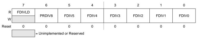
Figure 2-4. Flash Clock Divider Register (FCLKDIV)
