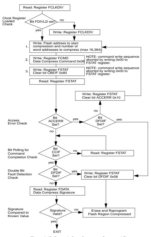
Figure 2-25. Example Data Compress Command Flow
