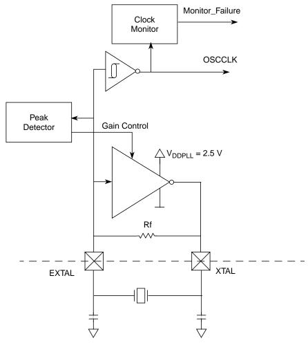
Figure 6-1. XOSC Block Diagram
