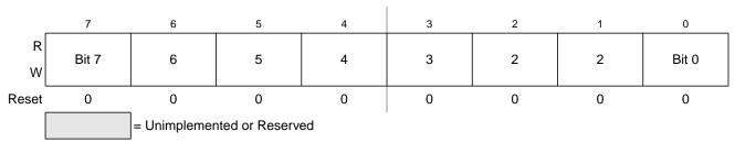
Figure 11-7. SPI Data Register (SPIDR)
