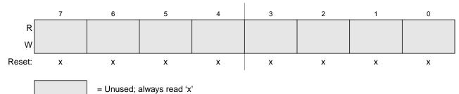
Figure 9-31. Identifier Register 2 — Standard Mapping
