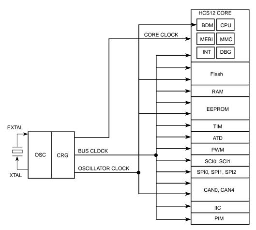
Figure 1-12. Clock Connections
