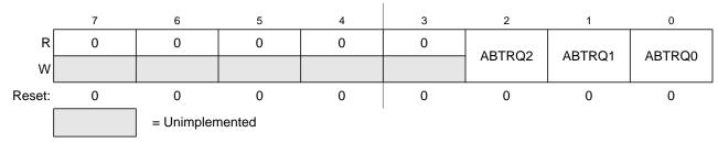
Figure 9-12. MSCAN Transmitter Message Abort Request Register (CANTARQ)
