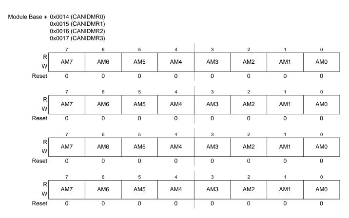
Figure 9-21. MSCAN Identifier Mask Registers (First Bank) — CANIDMR0-CANIDMR3
