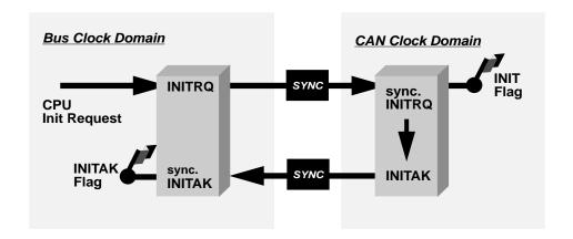
Figure 9-46. Initialization Request/Acknowledge Cycle
