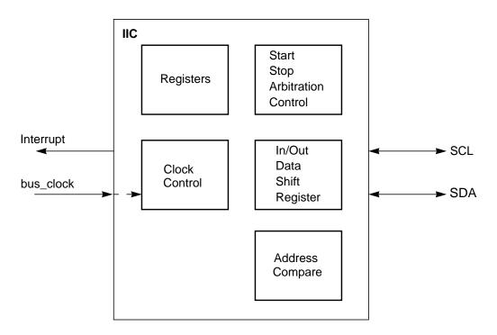
Figure 8-1. IIC Block Diagram
