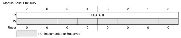
Figure 2-17. Flash Data High Register (FDATAHI)
