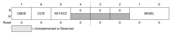
Figure 2-7. Flash Configuration Register (FCNFG)
