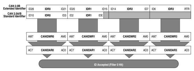
Figure 9-39. 32-bit Maskable Identifier Acceptance Filter
