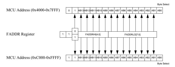
Figure 2-16. FADDR to MCU Address Mapping (Unpaged)
