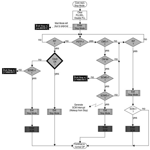
Figure 5-24. Stop Mode Entry/Exit Sequence
