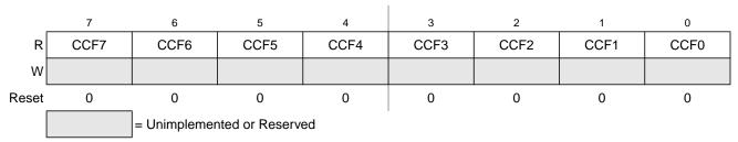
Figure 7-13. ATD Status Register 1 (ATDSTAT1)
