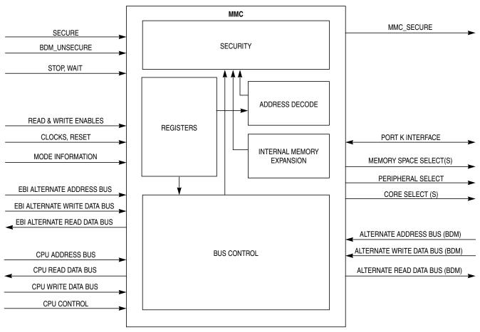
Figure 19-1. MMC Block Diagram
