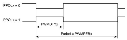
Figure 12-20. PWM Left Aligned Output Waveform
