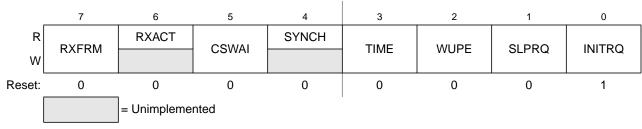
Figure 9-4. MSCAN Control Register 0 (CANCTL0)
