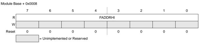
Figure 2-13. Flash Address High Register (FADDRHI)
