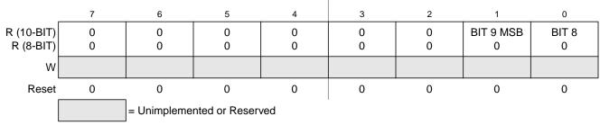
Figure 7-20. Right Justified, ATD Conversion Result Register x, High Byte (ATDDRxH)
