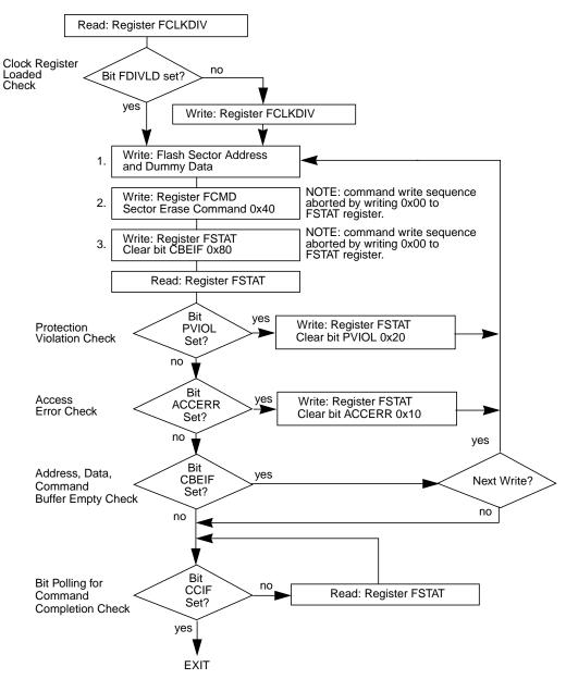
Figure 2-28. Example Sector Erase Command Flow
