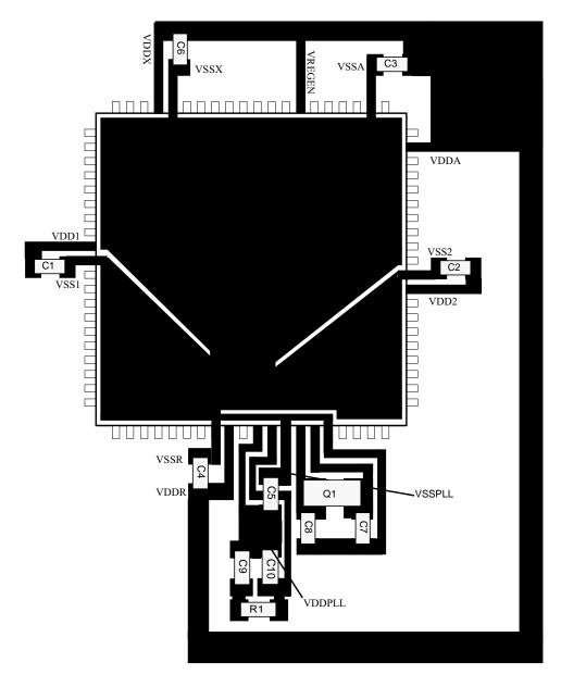
Figure B-2. Recommended PCB Layout for 80QFP
