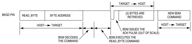
Figure 15-11. Handshake Protocol at Command Level
