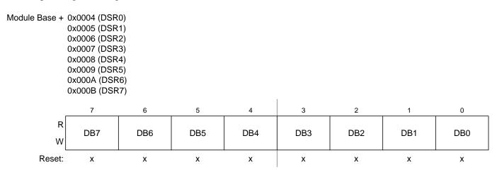
Figure 9-33. Data Segment Registers (DSR0-DSR7) — Extended Identifier Mapping
