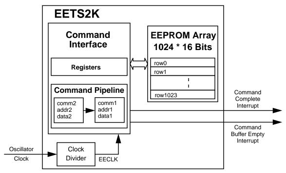
Figure 3-1. EETS2K Block Diagram
