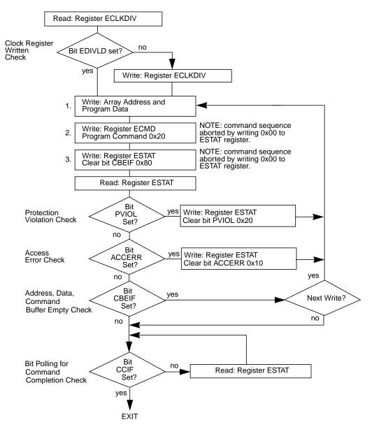
Figure 3-18. Example Program Command Flow
