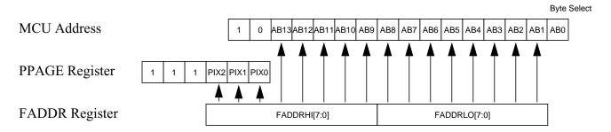
Figure 2-15. FADDR to MCU Address Mapping (Paged)
