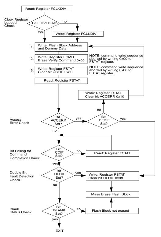
Figure 2-24. Example Erase Verify Command Flow
