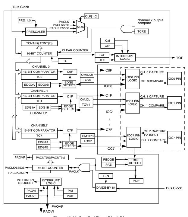
Figure 13-28. Detailed Timer Block Diagram
