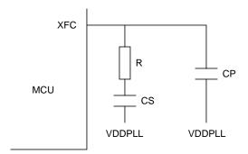
Figure 1-5. PLL Loop Filter Connections
