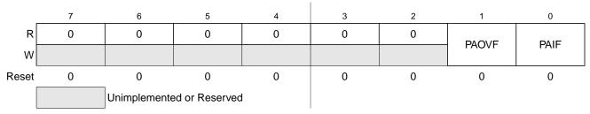
Figure 13-25. Pulse Accumulator Flag Register (PAFLG)
