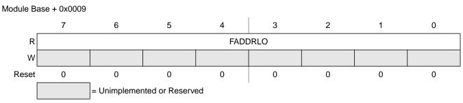
Figure 2-14. Flash Address Low Register (FADDRLO)
