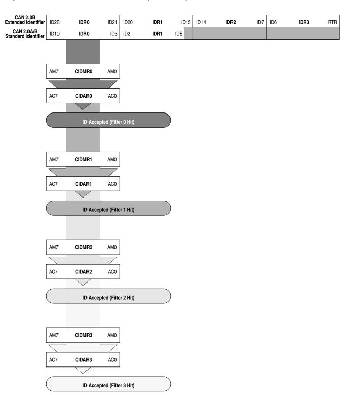
Figure 9-41. 8-bit Maskable Identifier Acceptance Filters
