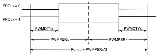
Figure 12-22. PWM Center Aligned Output Waveform
