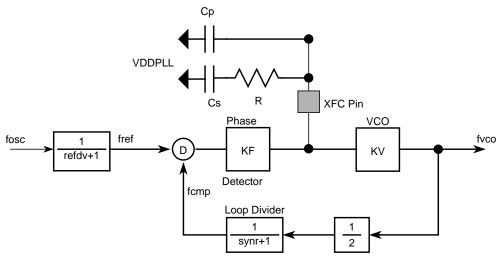
Figure A-3. Basic PLL Functional Diagram
