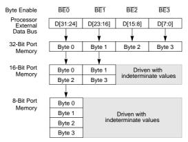
Figure 18-2. Connections for External Memory Port Sizes
