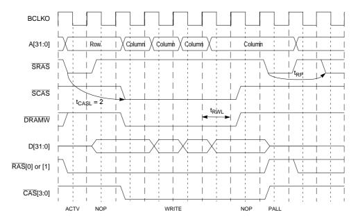
Figure 11-19. Burst Write SDRAM Access
