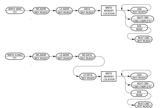
Figure 5-25. WRITE Command Sequence
