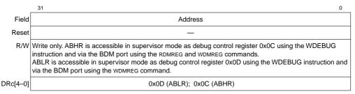
Figure 5-6. Address Breakpoint Registers (ABLR, ABHR)
