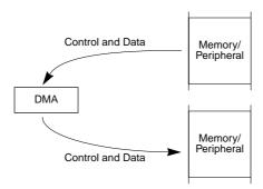
Figure 12-2. Dual-Address Transfer
