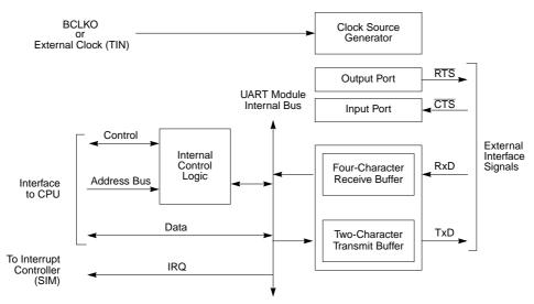
Figure 14-17. UART Block Diagram Showing External and Internal Interface Signals
