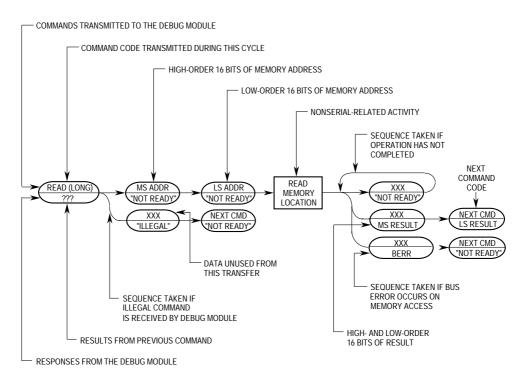
Figure 5-17. Command Sequence Diagram
