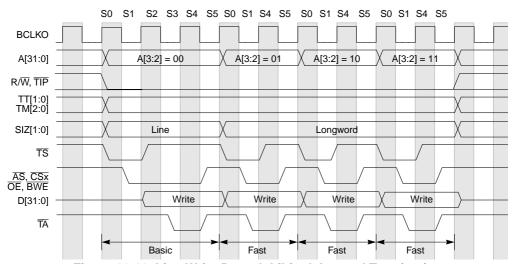
Figure 18-18. Line Write Burst-Inhibited, Internal Termination
