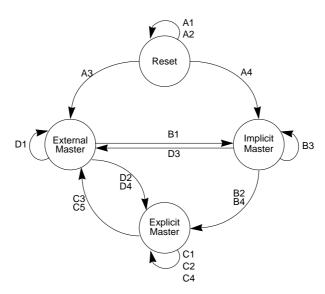
Figure 18-32. Three-Wire Bus Arbitration Protocol State Diagram
