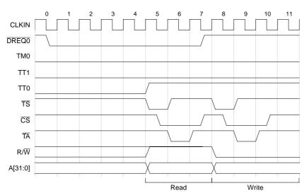
Figure 12-11. DREQ Timing Constraints, Dual-Address DMA Transfer
