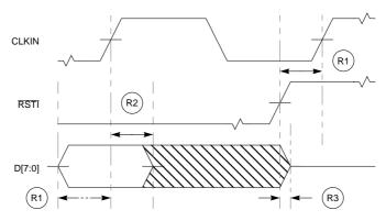
Note: Mode selects are registered on the rising CLKIN edge before the cycle in which  $\overline{\text{RSTI}}$  is recognized as being negated.
