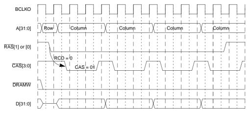
Figure 11-8. Burst Page-Mode Write Operation (4-3-3-3)
