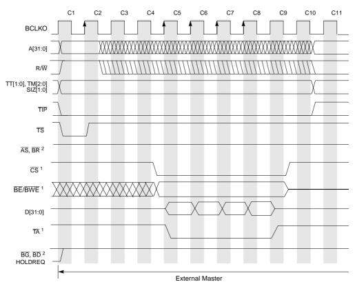
$<sup>^1</sup>$  Depending on programming, these signals may or may not be driven by the processor.  $^2$  These signals are driven by the processor for an external master transfer.
