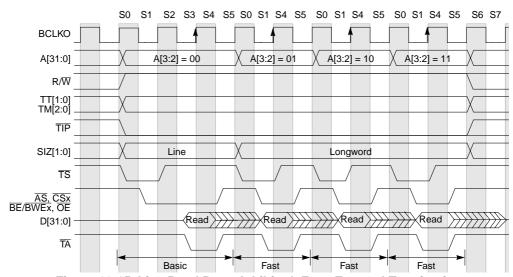
Figure 18-15. Line Read Burst-Inhibited, Fast, External Termination
