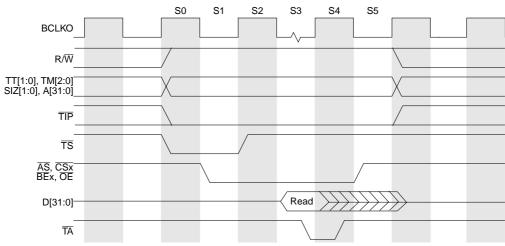
Figure 18-6. Basic Read Bus Cycle
