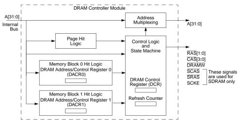
Figure 11-1. Asynchronous/Synchronous DRAM Controller Block Diagram
