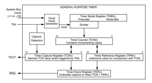
Figure 13-1. Timer Block Diagram
