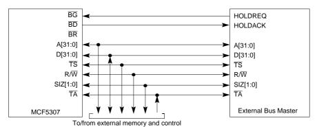
Figure 18-26. MCF5307 Two-Wire Mode Bus Arbitration Interface
