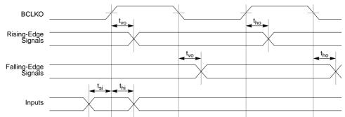
t<sub>vo</sub>=Propagation delay of signal relative to BCLKO edge
