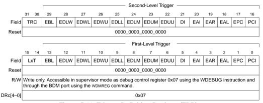
Figure 5-12. Trigger Definition Register (TDR)
