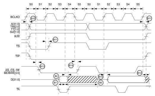
Figure 20-3. AC Timings—Normal Read and Write Bus Cycles
