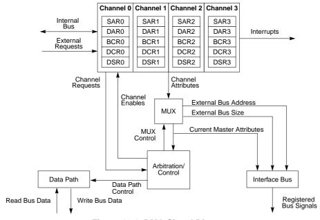
Figure 12-1. DMA Signal Diagram
