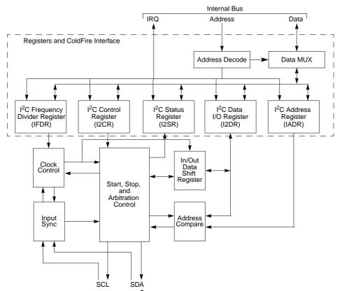
Figure 8-1. I<sup>2</sup>C Module Block Diagram
