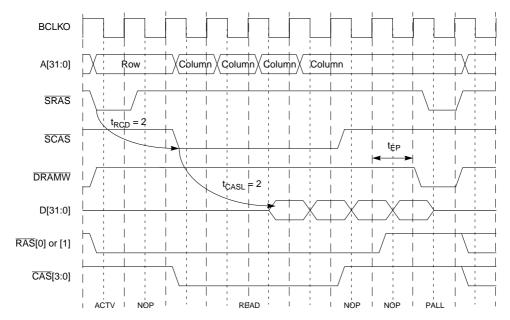
Figure 11-18. Burst Read SDRAM Access
