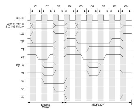
Figure 18-31. Three-Wire Bus Arbitration
