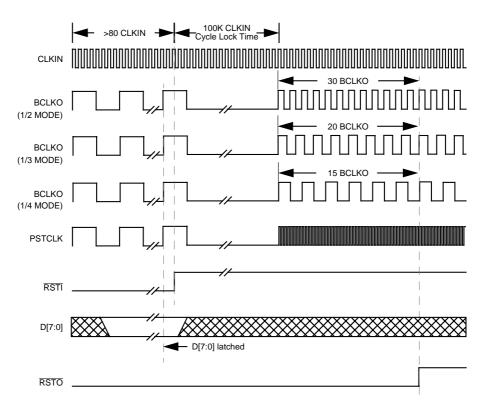
Figure 18-34. Software Watchdog Reset Timing
