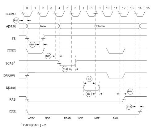
Figure 20-8. SDRAM Read Cycle with EDGESEL Tied Low
