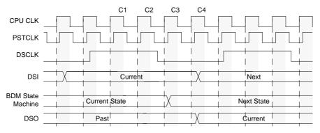
Figure 5-13. BDM Serial Interface Timing
