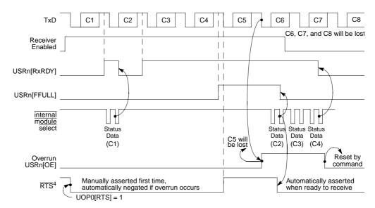
Figure 14-22. Receiver Timing
