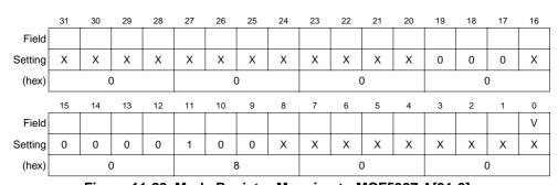
Figure 11-29. Mode Register Mapping to MCF5307 A[31:0]
