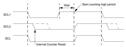
Figure 8-4. Synchronized Clock SCL
