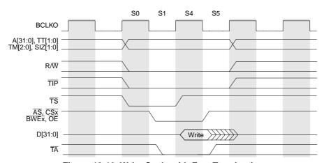
Figure 18-10. Write Cycle with Fast Termination
