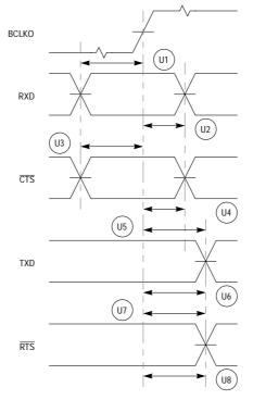
Figure 20-16. UART0/1 Module AC Timing—UART Mode
