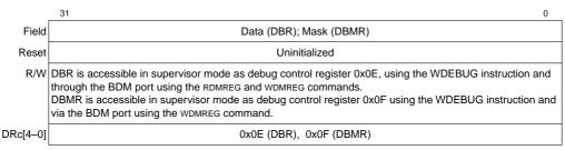
Figure 5-9. Data Breakpoint/Mask Registers (DBR and DBMR)
