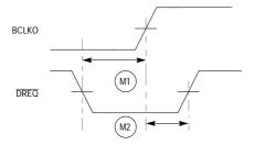
Figure 20-18. DMA Timing
