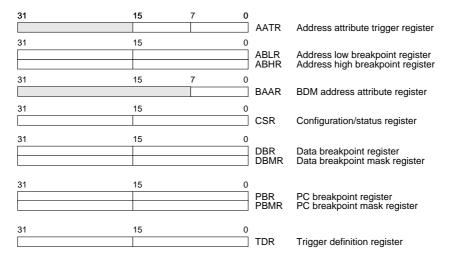
Note: Each debug register is accessed as a 32-bit register; shaded fields above are not used (don't care). All debug control registers are writable from the external development system or the CPU via the WDEBUG instruction.
