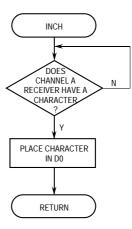
Figure 14-27. UART Mode Programming Flowchart (Sheet 4 of 5)
