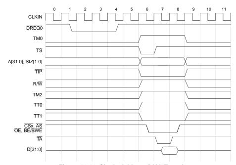
Figure 12-13. Single-Address DMA Transfer
