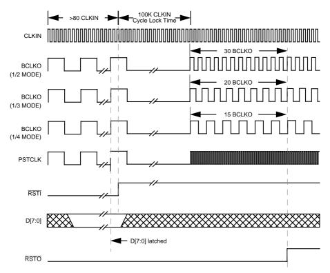
Figure 7-4. Reset and Initialization Timing
