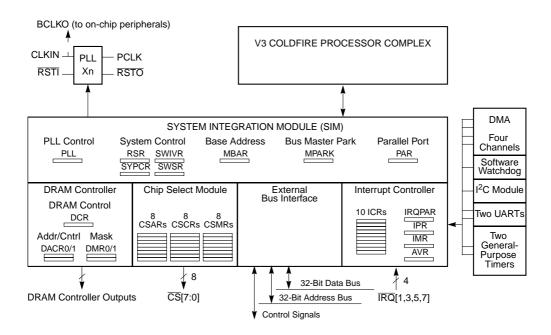
Figure 6-1. SIM Block Diagram
