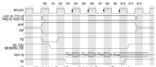
Figure 18-12. Line Read Burst (2-1-1-1), External Termination
