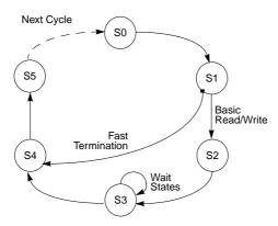
Figure 18-4. Data Transfer State Transition Diagram
