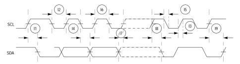
Figure 20-15. I<sup>2</sup>C Input/Output Timings
