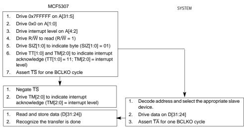
Figure 18-23. Interrupt-Acknowledge Cycle Flowchart
