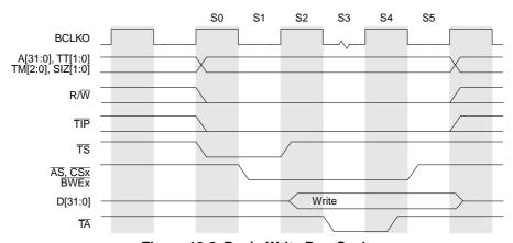
Figure 18-8. Basic Write Bus Cycle
