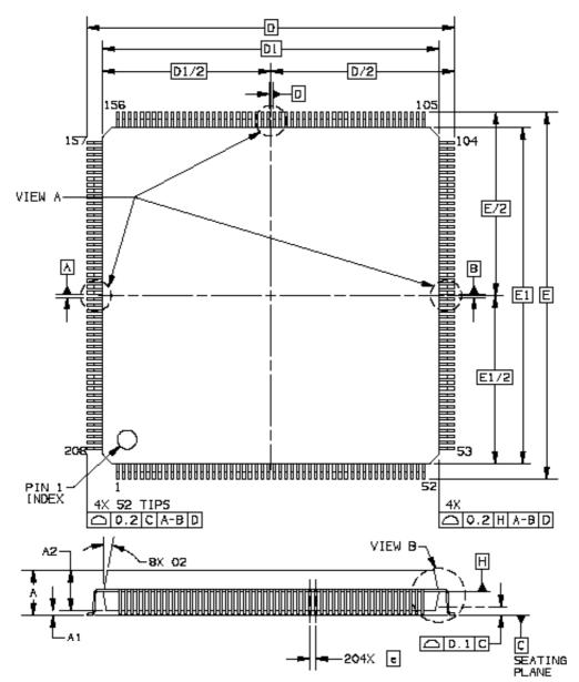
Figure 16-2. MCF5307 Case Drawing (General View)
