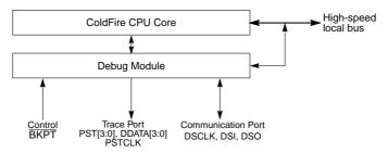
Figure 5-1. Processor/Debug Module Interface
