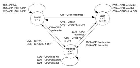
Figure 4-11. Cache Line State Diagram—Copyback Mode
