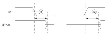
Figure 20-10. AC Output Timing—High Impedance
