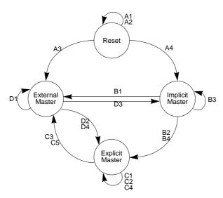
Figure 18-29. MCF5307 Two-Wire Bus Arbitration Protocol State Diagram
