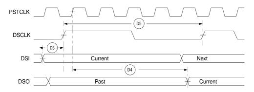
Figure 20-13. BDM Serial Port AC Timing
