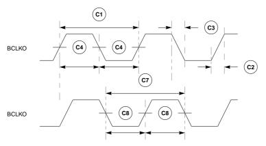
Note: Input and output AC timing specifications are measured to BCLKO with a 50-pF load capacitance (not including pin capacitance).
