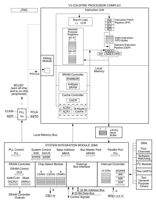
Figure 1-1. MCF5307 Block Diagram
