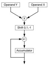
Figure 2-2. ColdFire Multiply-Accumulate Functionality Diagram
