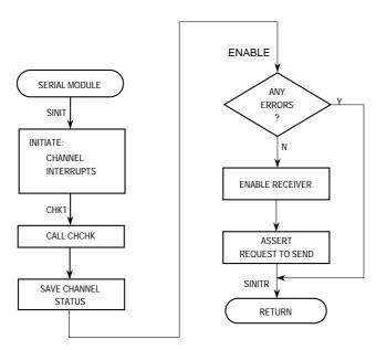
Figure 14-27. UART Mode Programming Flowchart (Sheet 1 of 5)
