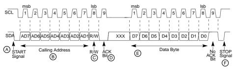
Figure 8-2. I<sup>2</sup>C Standard Communication Protocol
