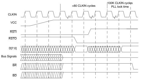
Figure 18-33. Master Reset Timing
