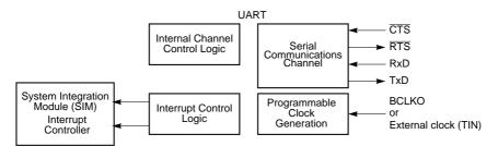
Figure 14-1. Simplified Block Diagram
