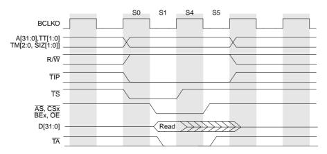
Figure 18-9. Read Cycle with Fast Termination
