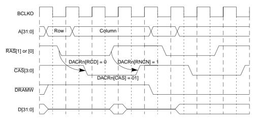
Figure 11-5. Basic Non-Page-Mode Operation RCD = 0, RNCN = 1 (4-4-4-4)
