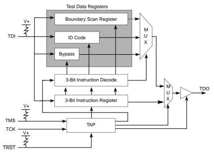
Figure 19-1. JTAG Test Logic Block Diagram
