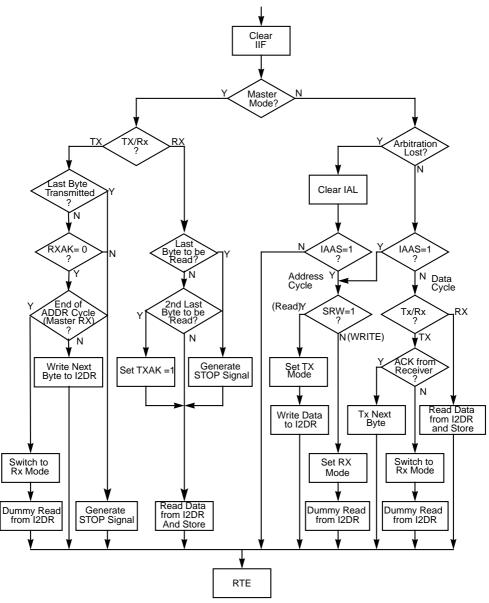
Figure 8-10. Flow-Chart of Typical I<sup>2</sup>C Interrupt Routine
