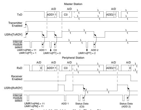
Figure 14-26. Multidrop Mode Timing Diagram
