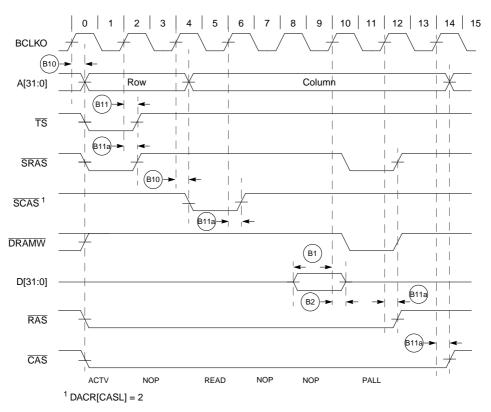
Figure 20-6. SDRAM Read Cycle with EDGESEL Tied High
