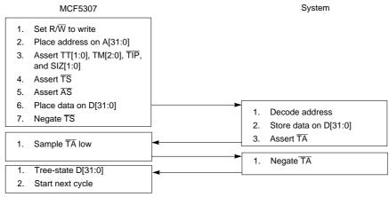
Figure 18-7. Write Cycle Flowchart
