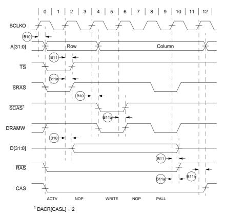
Figure 20-7. SDRAM Write Cycle with EDGESEL Tied High
