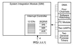
Figure 9-1. Interrupt Controller Block Diagram
