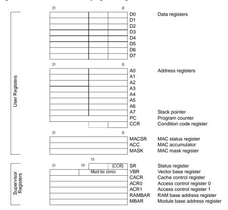
Figure 1-4. ColdFire MCF5307 Programming Model
