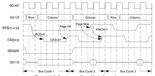
Figure 11-9. Continuous Page-Mode Operation
