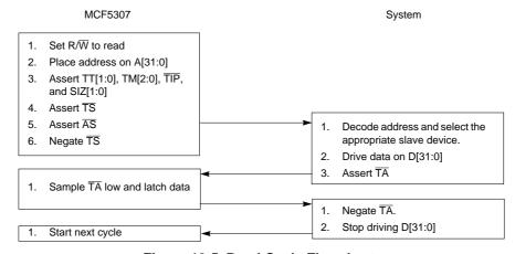
Figure 18-5. Read Cycle Flowchart
