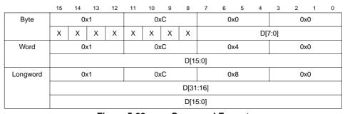
Figure 5-28. FILL Command Format
