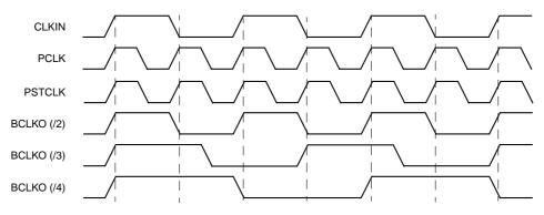
NOTE: The clock signals are shown with edges aligned to show frequency relationships only. Actual signal edges have some skew between them.
