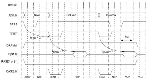
Figure 11-20. Synchronous, Continuous Page-Mode Access—Consecutive Reads
