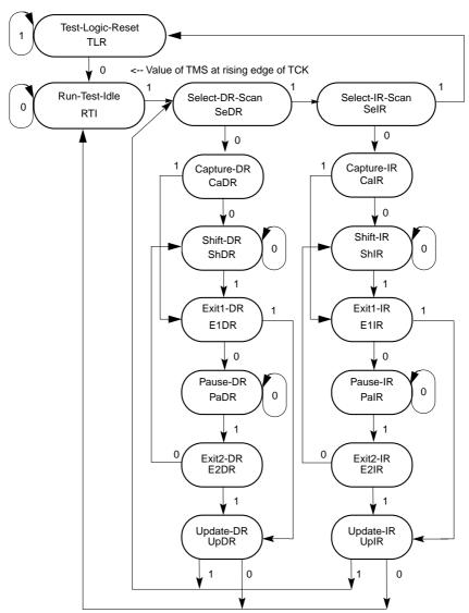
Figure 19-2. JTAG TAP Controller State Machine
