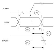
Figure 20-17. General-Purpose I/O Timing
