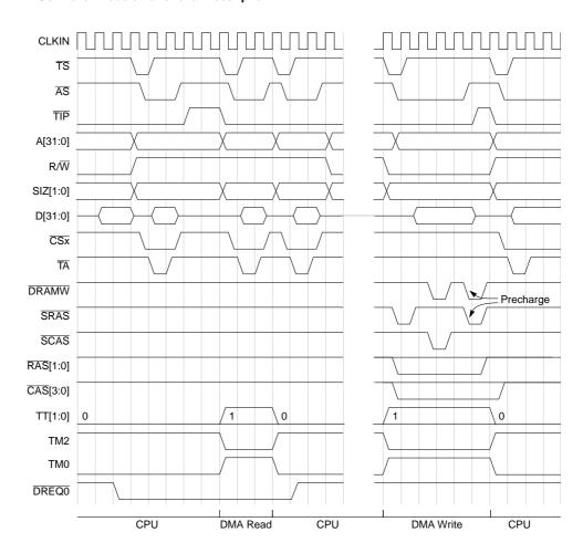
Figure 12-12. Dual-Address, Peripheral-to-SDRAM, Lower-Priority DMA Transfer
