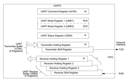
Figure 14-20. Transmitter and Receiver Functional Diagram
