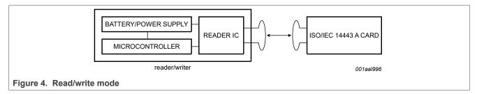
A typical system using the MFRC630 is using a microcontroller to implement the higher levels of the contactless communication protocol and a power supply (battery or external supply).
