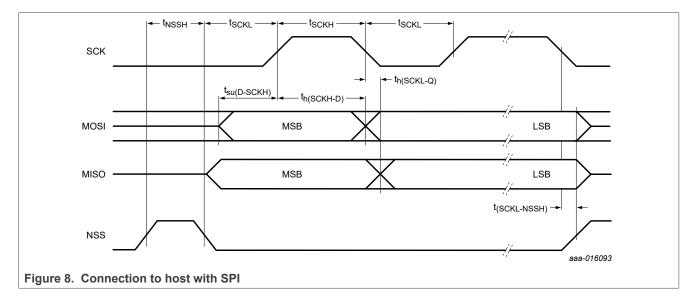
**Remark:** To send more bytes in one data stream the NSS signal must be LOW during the send process. To send more than one data stream the NSS signal must be HIGH between each data stream.
