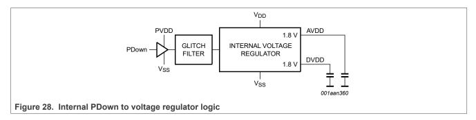
When the MFRC630 has finished the reset phase and the oscillator has entered a stable working condition the IC is ready to be used. A typical duration before the IC is ready to receive commands after the reset had been released is 2.5ms.
