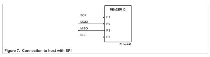
The MFRC630 acts as a slave during the SPI communication. The SPI clock SCK has to be generated by the master. Data communication from the master to the slave uses the Line MOSI. Line MISO is used to send data back from the MFRC630 to the master.
