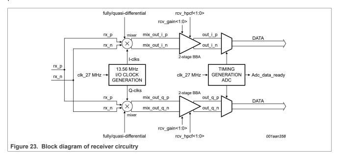
The receiver can also be operated in a single ended mode. In this case the Rcv\_RX\_single bit has to be set. In the single ended mode, the two receiver pins RXP and RXN need to be connected together and will provide a single ended signal to the receiver circuitry.
