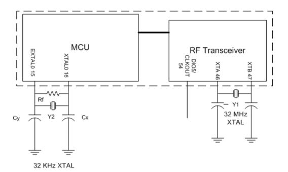
Figure 4. MKW01 Two Crystal System Clock Connection
