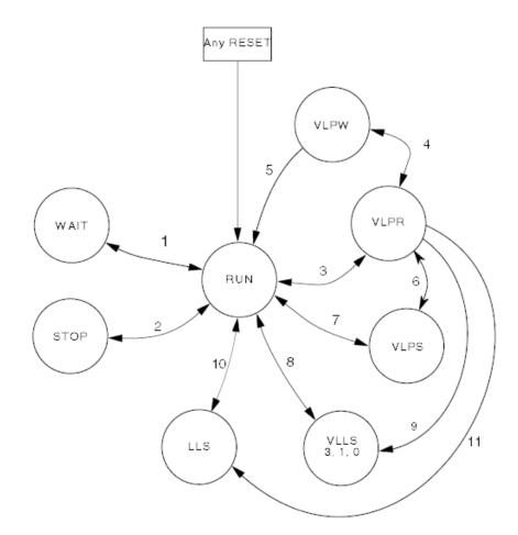
Figure 6. Power mode state transition diagram
