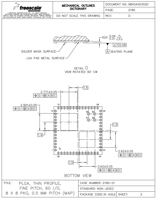
Figure 9. Mechanical Drawing (2 of 2)
