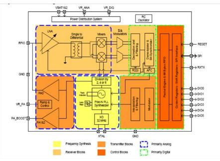
Figure 2. MKW01 Transceiver Block Diagram
