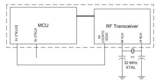
Figure 3. MKW01 Single Crystal System Clock Connection
