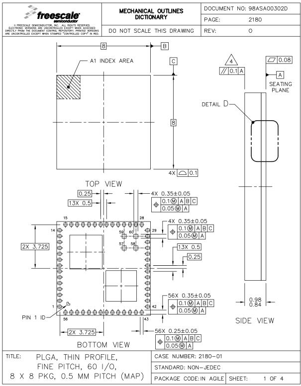
Figure 8. Mechanical Drawing (1 of 2)
