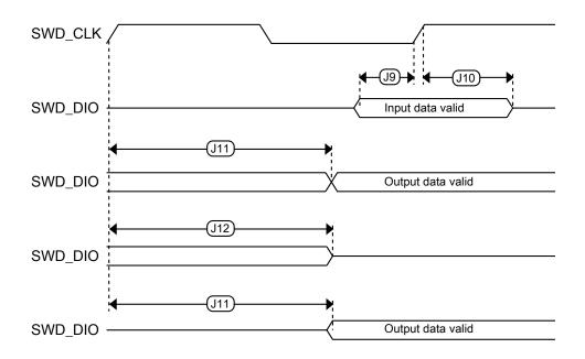
Figure 4. Serial wire data timing
