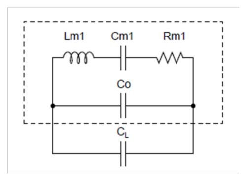
Figure 7. Crystal Electrical Block Diagram
