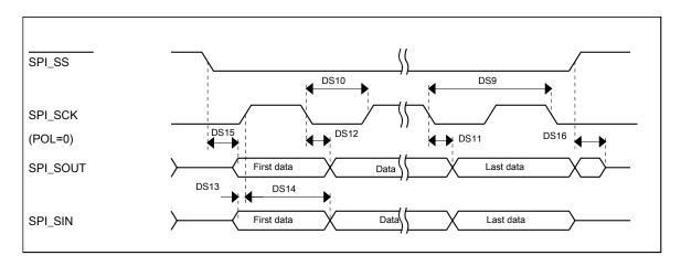
Figure 14. DSPI classic SPI timing — slave mode
