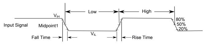
The midpoint is V<sub>IL</sub> + (V<sub>IH</sub> - V<sub>IL</sub>) / 2
