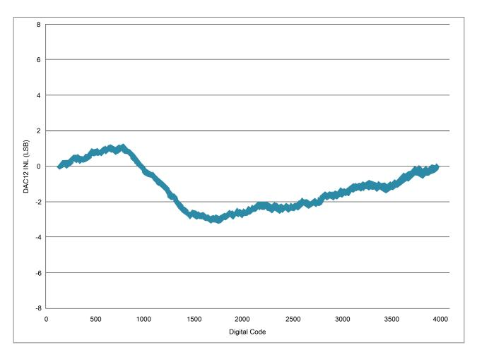
Figure 11. Typical INL error vs. digital code
