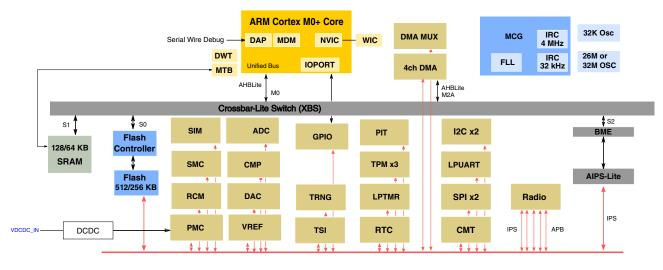
Figure 1. KW41Z Detailed Block Diagram
