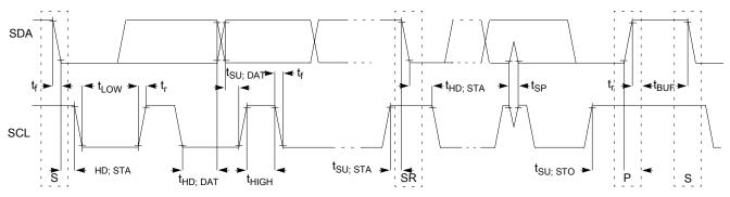
Figure 17. Timing definition for fast and standard mode devices on the I<sup>2</sup>C bus
