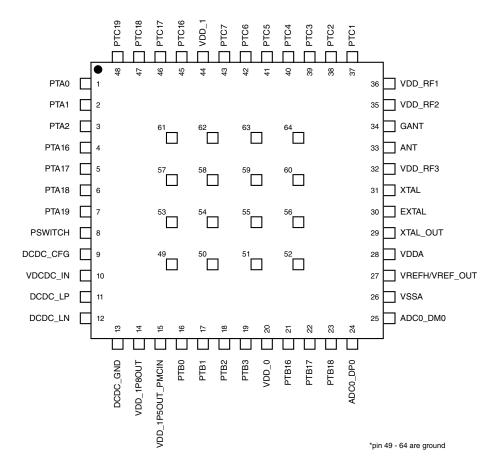
Figure 18. 48-pin Laminate QFN pinout diagram
