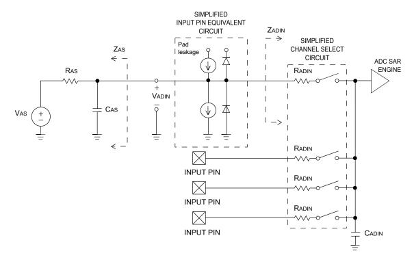
Figure 8. ADC input impedance equivalency diagram
