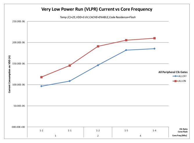
Figure 4. VLPR mode current vs. core frequency
