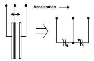
Figure 3. Transducer Physical Model
