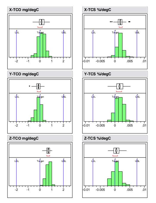
Figure 7. MMA7331LC (4g only) Temperature Coefficient of Offset (TCO) and Temperature Coefficient of Sensitivity (TCS) Distribution Charts
