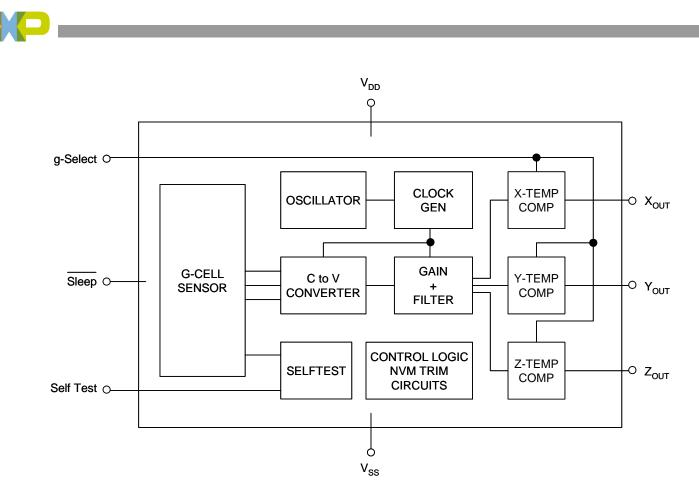
Figure 2. Simplified Accelerometer Functional Block Diagram
