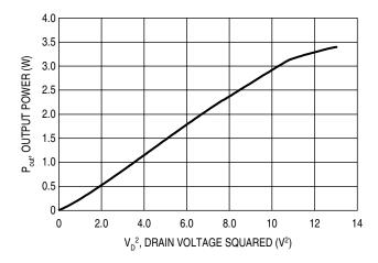
Figure 21. Output Power versus Drain Voltage
