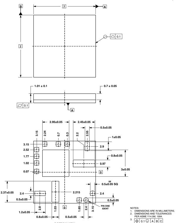
Figure 31. Outline Dimensions for 7x7 mm Module (Case 1383-02, Issue A)
