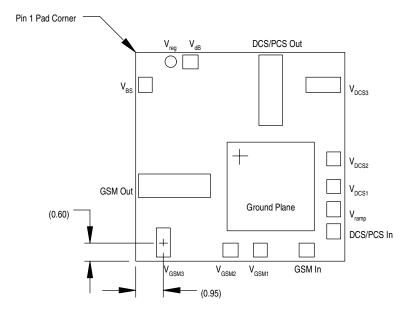
**NOTE:** For optimum performance  $V_{GSM1}$  and  $V_{GSM2}$ , as well as  $V_{DCS1}$  and  $V_{DCS2}$ , must be strapped together on the application demobard.
