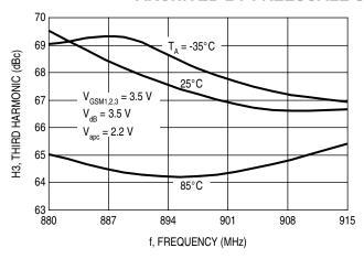
Figure 11. Third Harmonic Output versus Frequency
