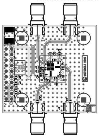
Figure 28. PA Evaluation Circuit PCB
