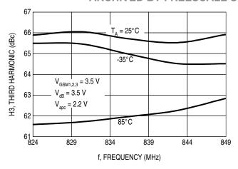
Figure 6. Third Harmonic Outputversus Frequency
