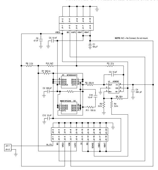
Figure 27. Power Amplifier Control Loop
