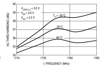
Figure 15. Third Harmonic Output versus Frequency
