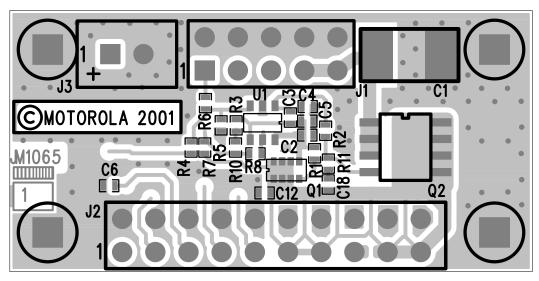
Figure 29. Power Amplifier Control Loop PCB
