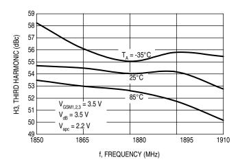
Figure 19. Third Harmonic Output versus Frequency
