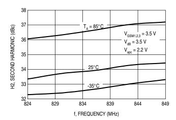
Figure 5. Second Harmonic Output versus Frequency
