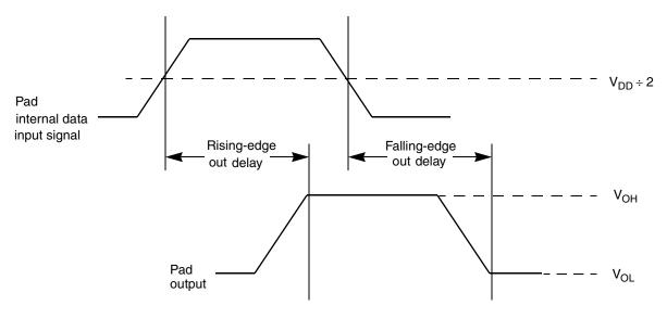
Figure 4. Pad Output Delay
