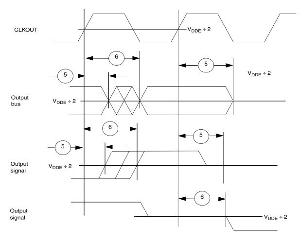
Figure 13. Synchronous Output Timing
