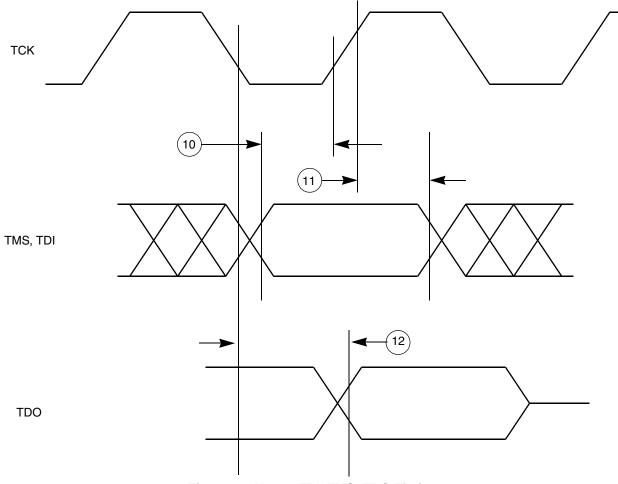
Figure 11. Nexus TDI, TMS, TDO Timing
