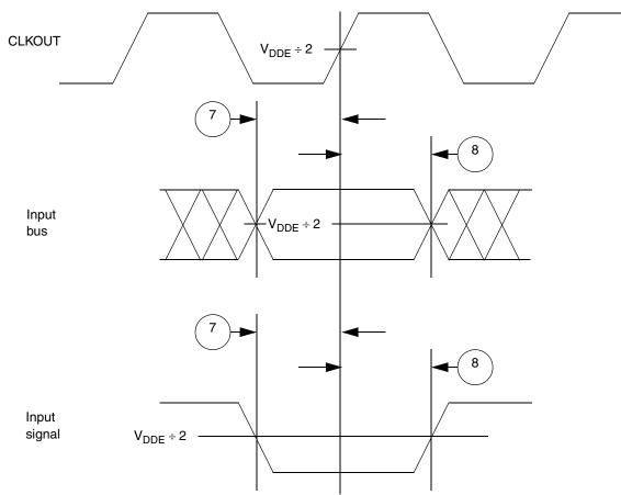
Figure 14. Synchronous Input Timing
