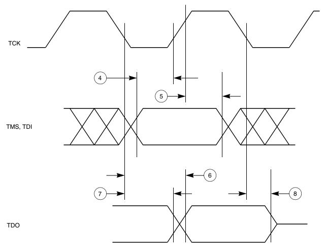
Figure 7. JTAG Test Access Port Timing
