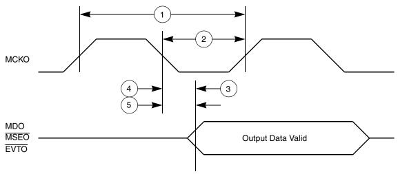
Figure 10. Nexus Output Timing
