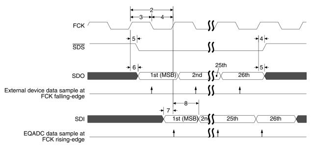
Figure 27. EQADC SSI Timing
