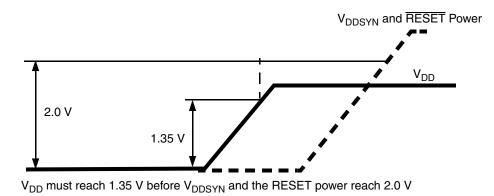
Figure 3. Power-Up Sequence (V<sub>RC33</sub> Grounded)
