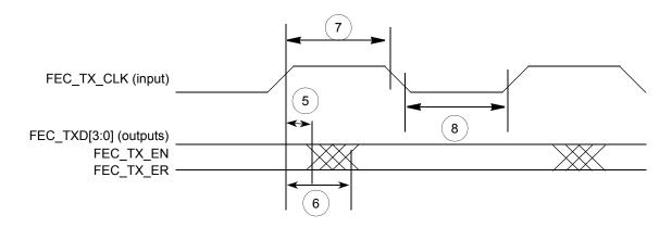
Figure 29. MII FEC Transmit Signal Timing Diagram
