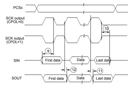
Figure 19. DSPI Classic SPI Timing—Master, CPHA = 1
