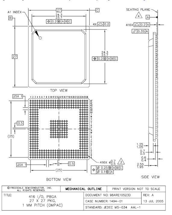
Figure 38. MPC5567 416 TEPBGA Package
