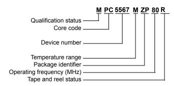
Temperature Range  $M = -40^{\circ} C$  to  $125^{\circ} C$
