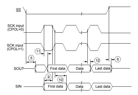
Figure 25. DSPI Modified Transfer Format Timing—Slave, CPHA = 1
