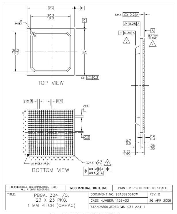
Figure 37. MPC5567 324 TEPBGA Package
