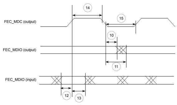
Figure 31. MII FEC Serial Management Channel Timing Diagram
