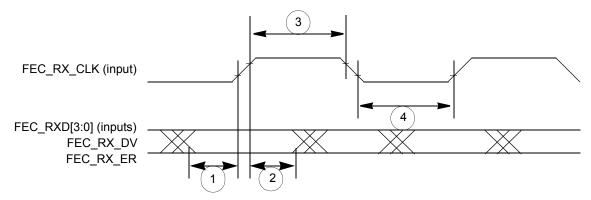
Figure 28. MII FEC Receive Signal Timing Diagram
