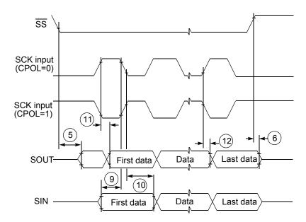
Figure 21. DSPI Classic SPI Timing—Slave, CPHA = 1
