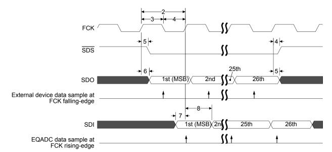
Figure 27. EQADC SSI Timing
