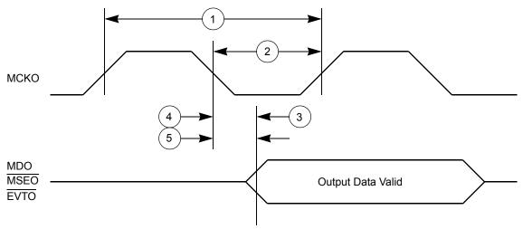
Figure 10. Nexus Output Timing
