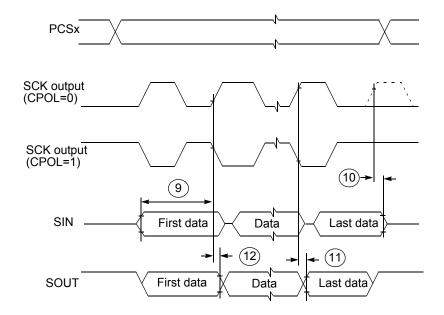
Figure 23. DSPI Modified Transfer Format Timing—Master, CPHA = 1
