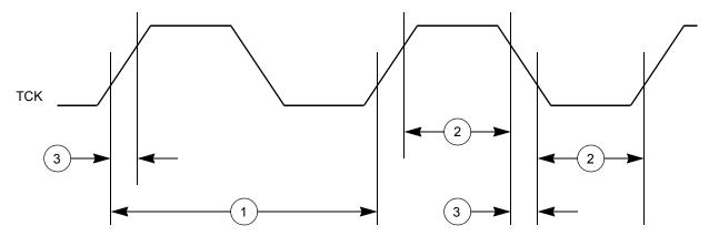
Figure 6. JTAG Test Clock Input Timing
