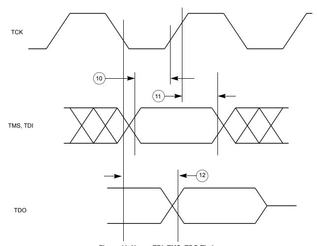
Figure 11. Nexus TDI, TMS, TDO Timing
