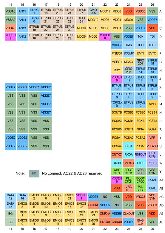
Figure 35. MPC5567 416 Package Right Side (view 2 of 2)
