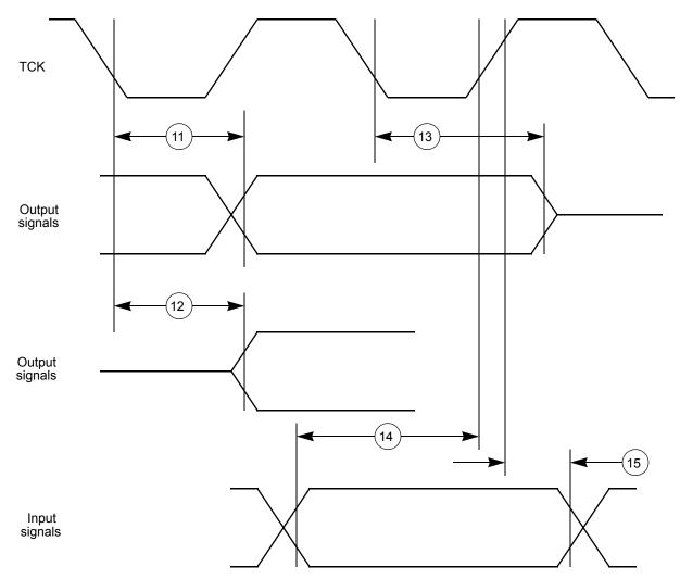
Figure 9. JTAG Boundary Scan Timing
