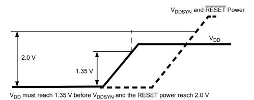
Figure 3. Power-Up Sequence (V<sub>RC33</sub> Grounded)
