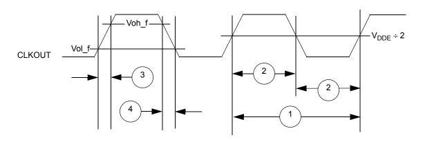
Figure 12. CLKOUT Timing
