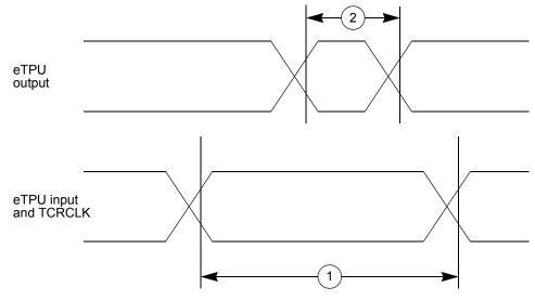
Figure 16. eTPU Timing
