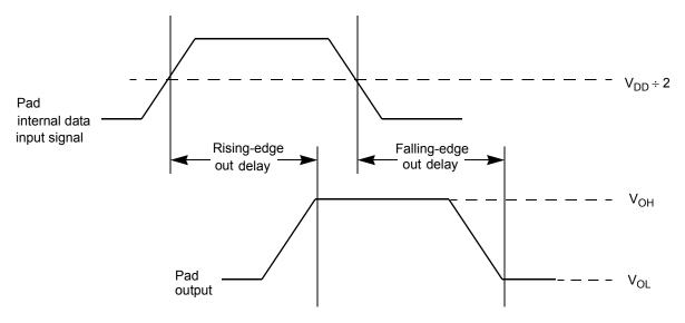
Figure 4. Pad Output Delay
