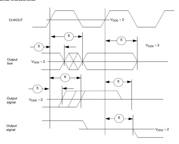
Figure 13. Synchronous Output Timing
