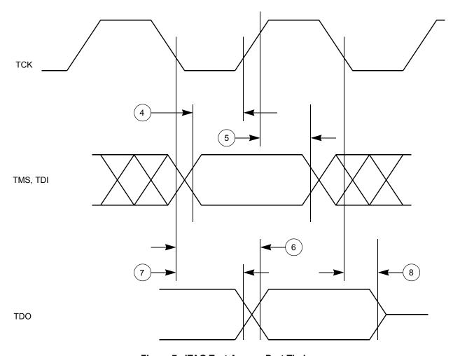
Figure 7. JTAG Test Access Port Timing
