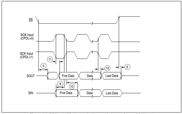
Figure 31. DSPI modified transfer format timing — Slave, CPHA = 1
