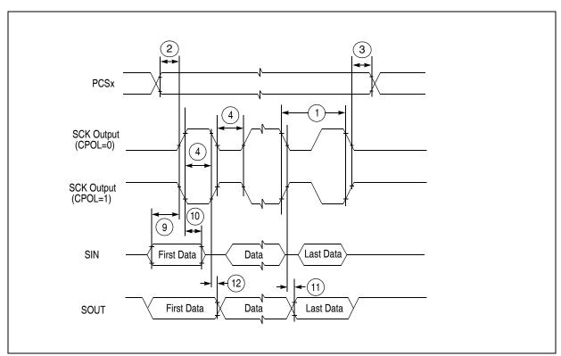
Figure 24. DSPI classic SPI timing — Master, CPHA = 0
