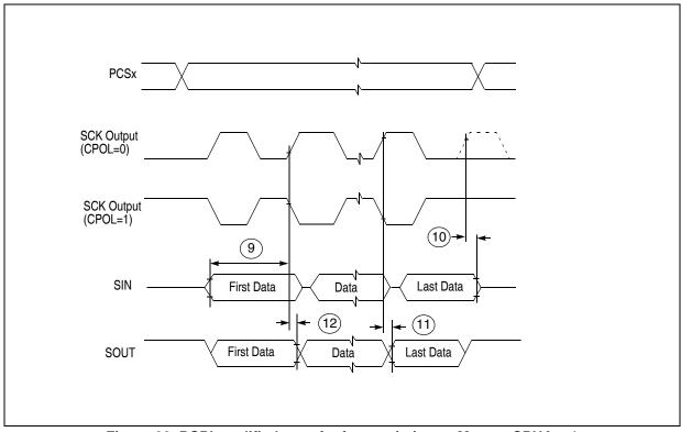
Figure 29. DSPI modified transfer format timing — Master, CPHA = 1
