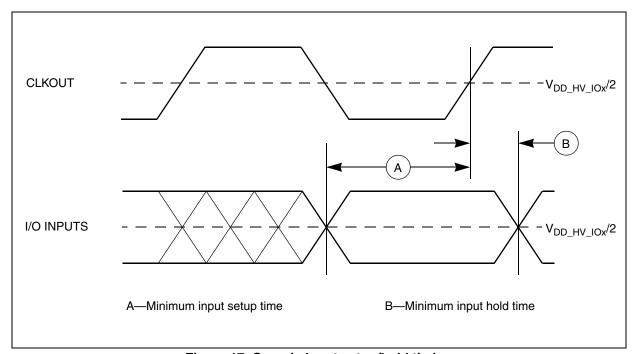
Figure 17. Generic Input setup/hold timing
