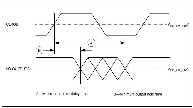
Figure 16. Generic output delay/hold timing
