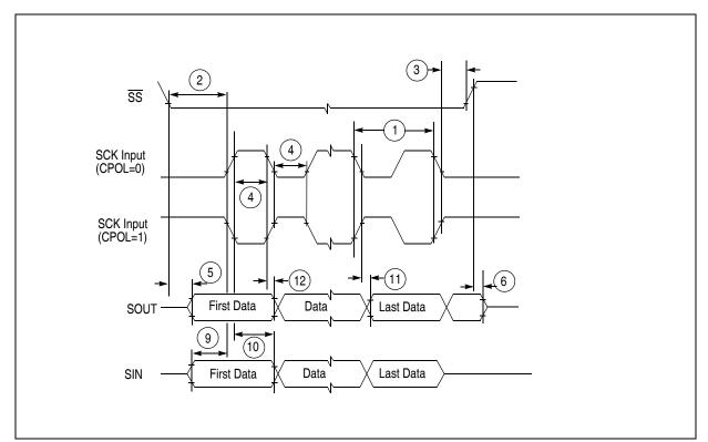
Figure 26. DSPI classic SPI timing — Slave, CPHA = 0
