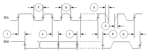
Figure 38. I<sup>2</sup>C input/output timing
