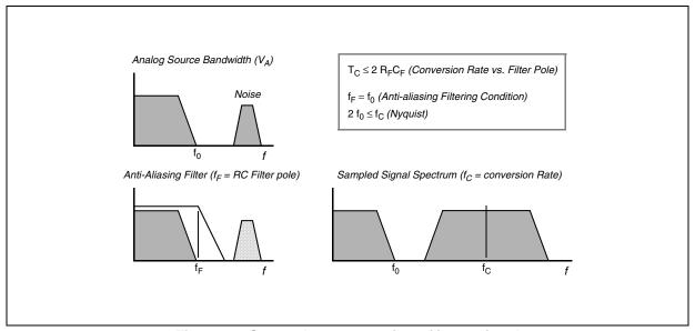
Figure 14. Spectral representation of input signal
