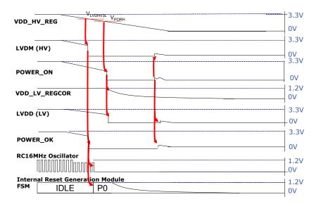
Figure 10. Power-down typical sequence
