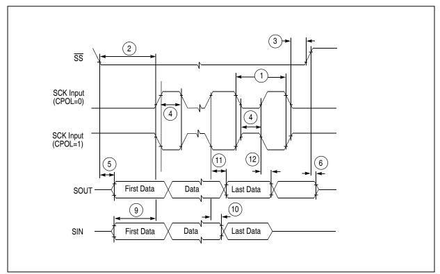
Figure 30. DSPI modified transfer format timing — Slave, CPHA = 0
