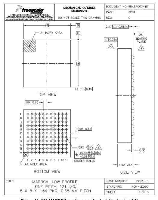
Figure 41. 121 MAPBGA package mechanical drawing (part 1)
