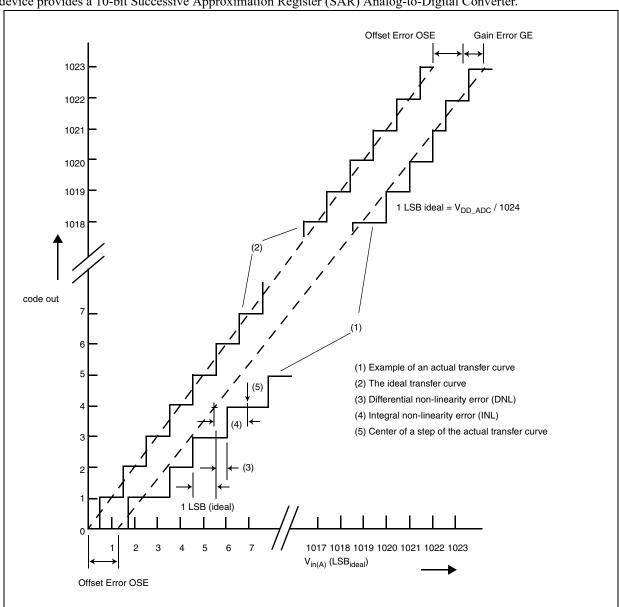
Figure 11. ADC characteristics and error definitions
