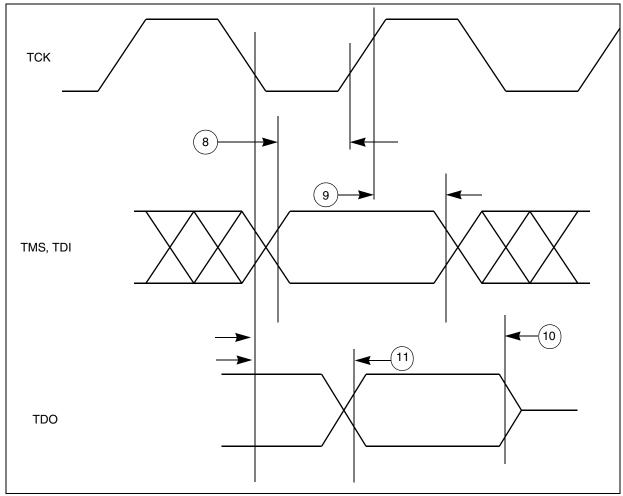
Figure 22. Nexus TDI, TMS, TDO Timing
