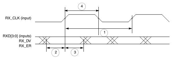
Figure 34. MII receive signal timing diagram
