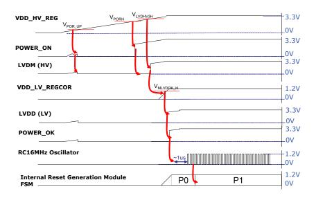
Figure 9. Power-up typical sequence
