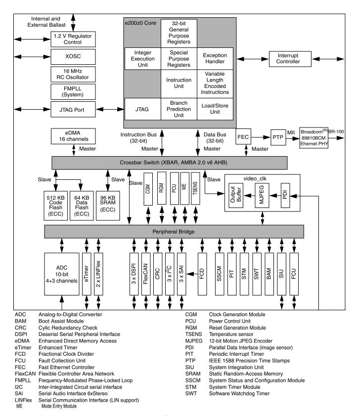
Figure 1. MPC5606E block diagram
