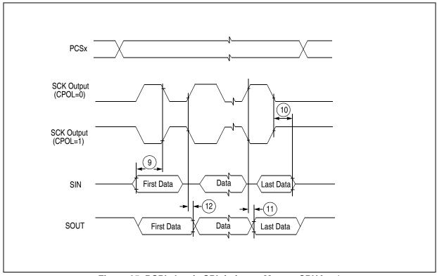
Figure 25. DSPI classic SPI timing — Master, CPHA = 1
