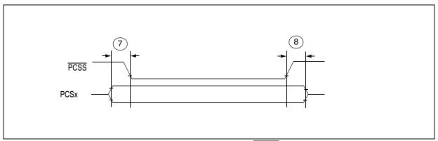
Figure 32. DSPI PCS Strobe (PCSS) timing
