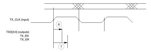
Figure 35. MII transmit signal timing diagram
