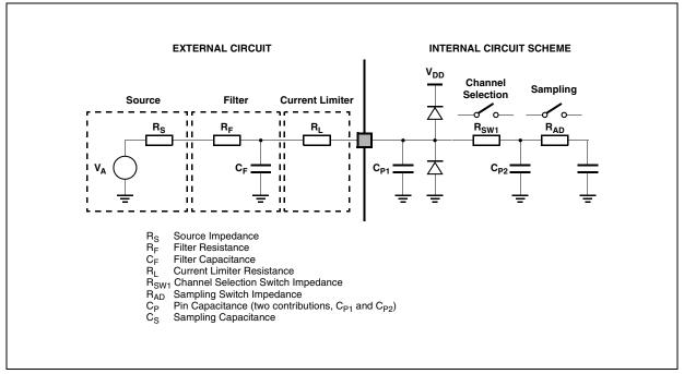
Figure 12. Input equivalent circuit
