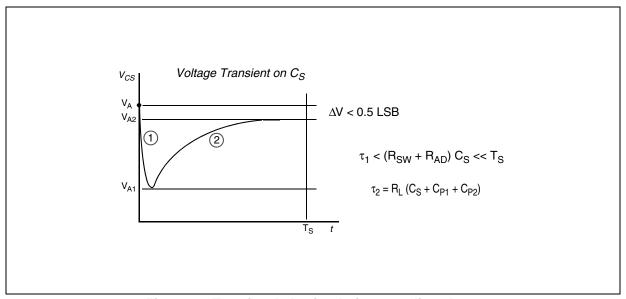
Figure 13. Transient behavior during sampling phase
