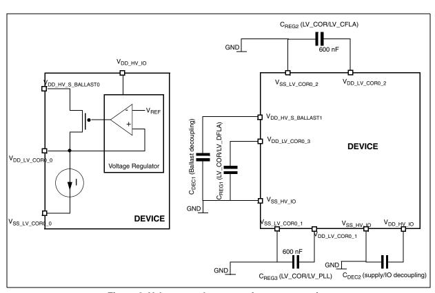
Figure 8. Voltage regulator capacitance connection
