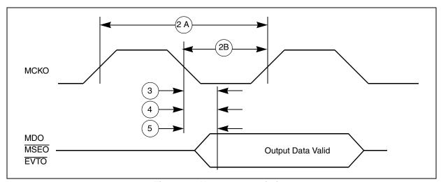
Figure 20. Nexus output timing
