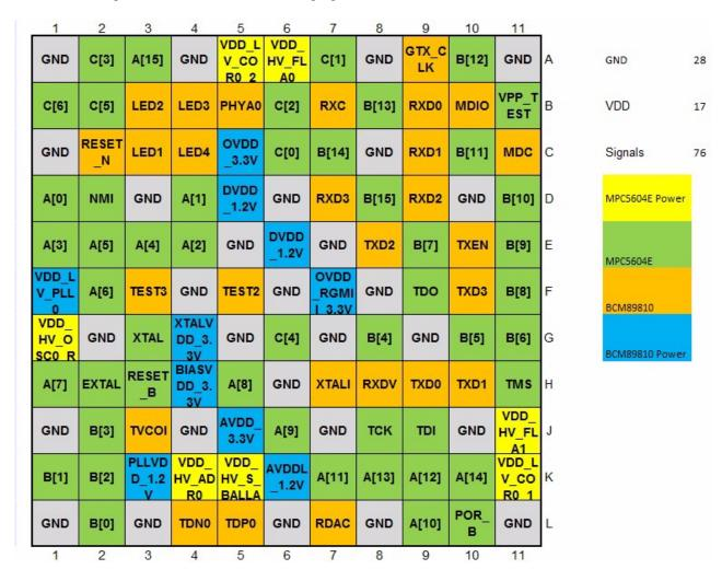
Figure 2. 121 MAPBGA pinout(top view)
