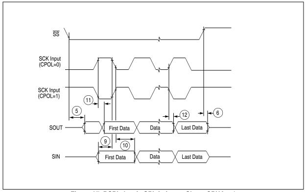
Figure 27. DSPI classic SPI timing — Slave, CPHA = 1
