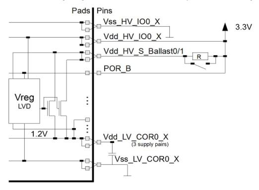
Figure 6. Internal Regulation Mode
