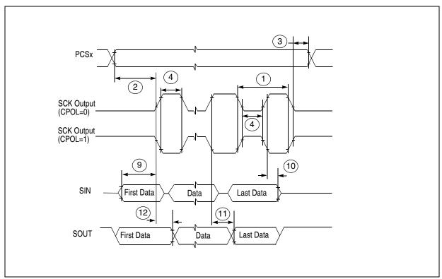
Figure 28. DSPI modified transfer format timing — Master, CPHA = 0
