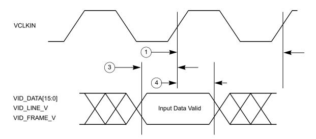
Figure 33. Video interface timing
