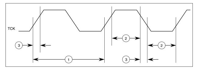
Figure 19. JTAG test clock input timing
