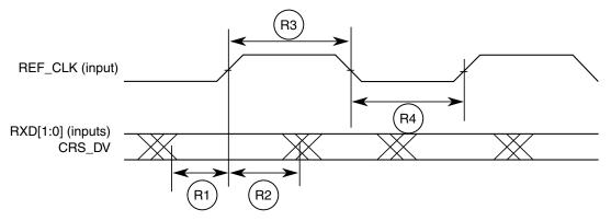
Figure 47. RMII receive signal timing diagram
