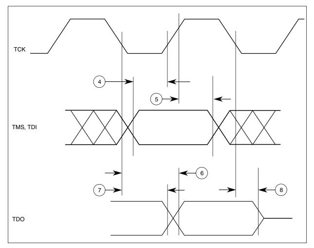
Figure 20. JTAG test access port timing
