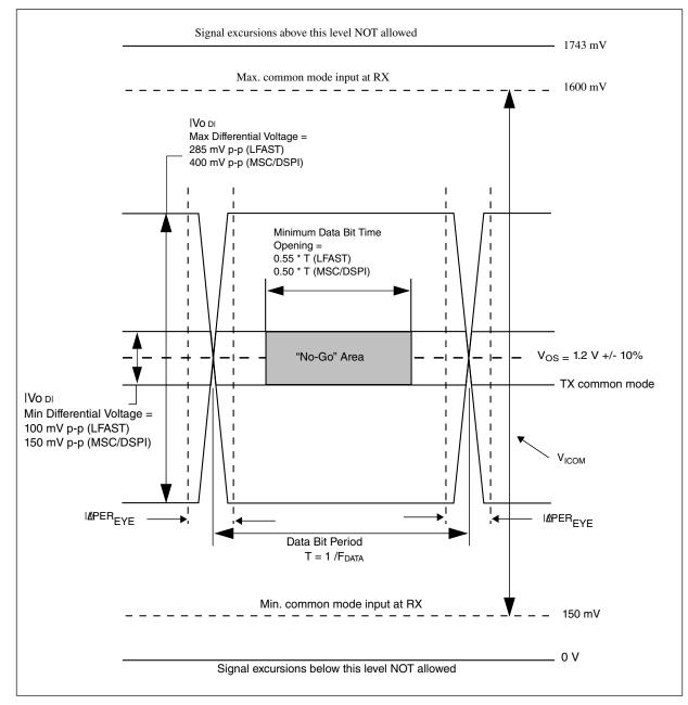
Figure 8. LFAST and MSC/DSPI LVDS timing definition
