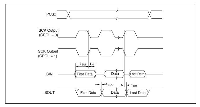
Figure 33. DSPI CMOS master mode – classic timing, CPHA = 1
