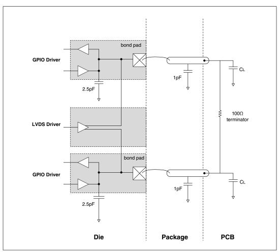
Figure 11. LVDS pad external load diagram
