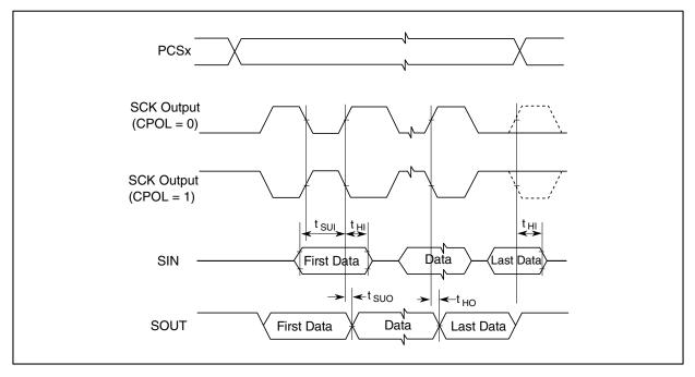
Figure 36. DSPI CMOS master mode – modified timing, CPHA = 1
