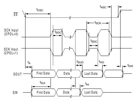
Figure 41. DSPI Slave Mode - Modified transfer format timing (MFTE = 0/1) — CPHA = 0
