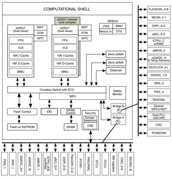
Figure 1. MPC5777C block diagram
