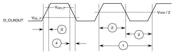
Figure 25. D\_CLKOUT timing
