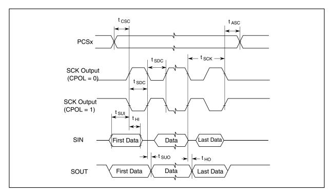
Figure 35. DSPI CMOS master mode – modified timing, CPHA = 0
