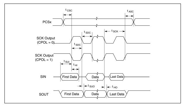
Figure 38. DSPI LVDS master mode – modified timing, CPHA = 0
