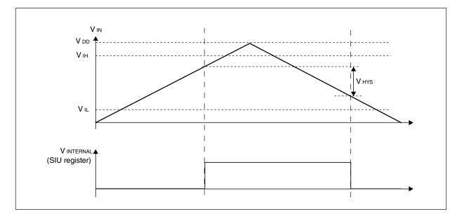
Figure 4. I/O input DC electrical characteristics definition
