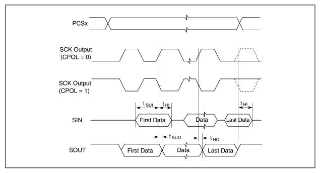
Figure 39. DSPI LVDS master mode – modified timing, CPHA = 1
