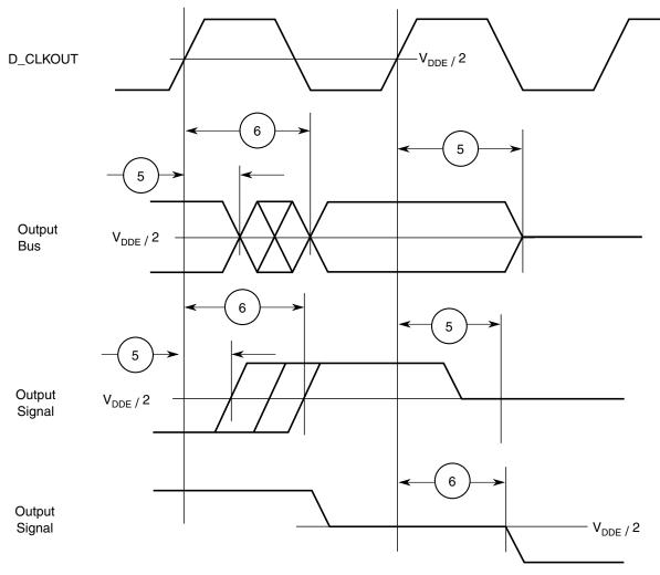
Figure 26. Synchronous output timing
