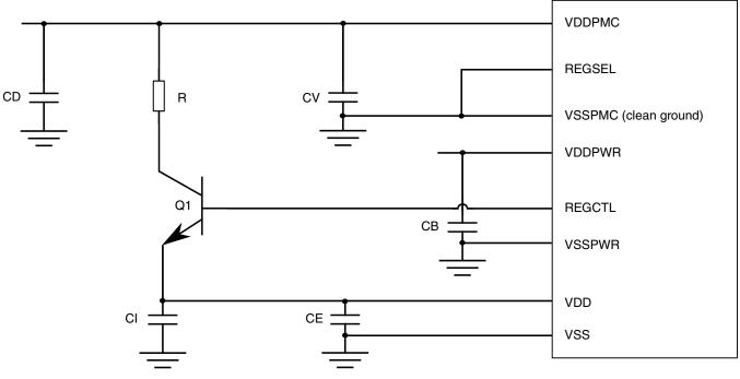
Figure 12. VRC 1.2 V LDO configuration
