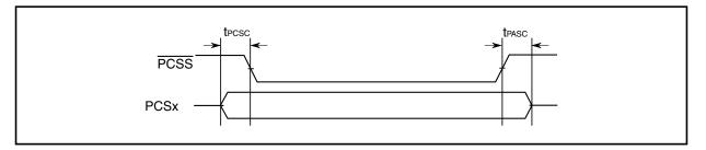
Figure 34. DSPI PCS strobe (PCSS) timing (master mode)
