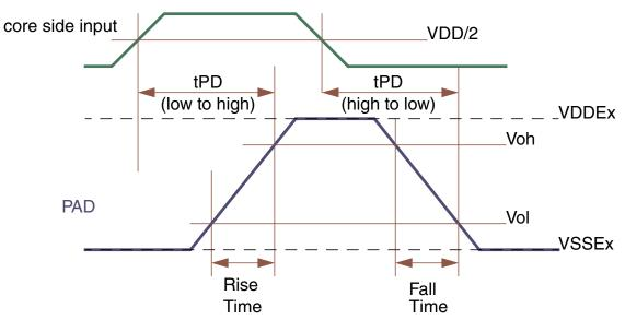
Figure 5. I/O output DC electrical characteristics definition
