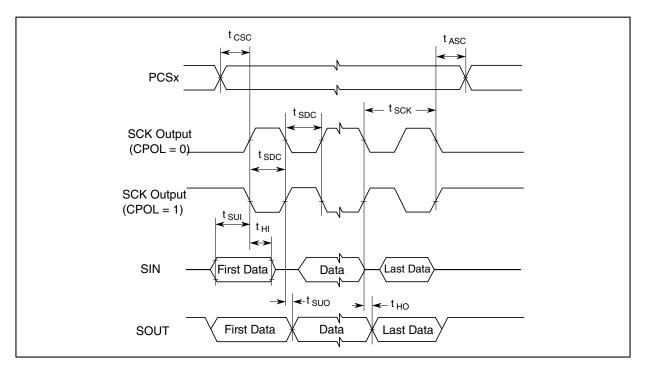
Figure 32. DSPI CMOS master mode – classic timing, CPHA = 0
