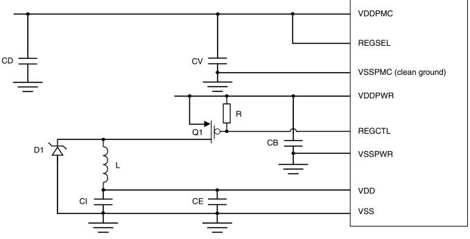
Figure 13. SMPS configuration
