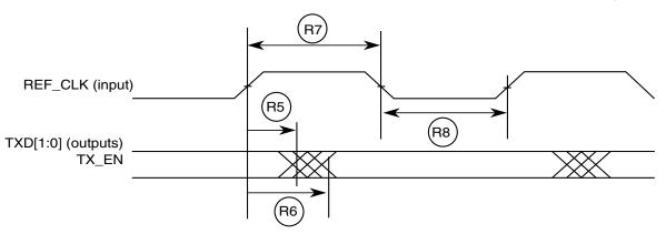
Figure 48. RMII transmit signal timing diagram
