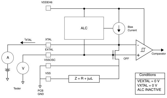
Figure 7. Test circuit
