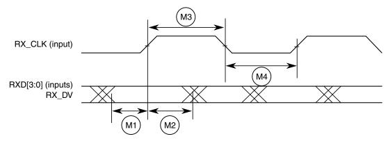
Figure 43. MII receive signal timing diagram
