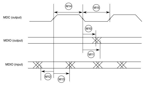
Figure 46. MII serial management channel timing diagram
