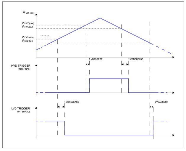
Figure 15. Voltage monitor threshold definition
