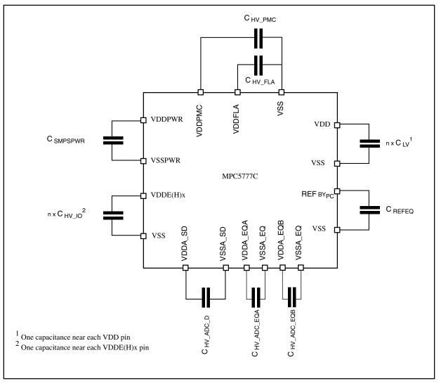
Figure 14. Recommended supply pin circuits
