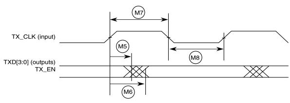
Figure 44. MII transmit signal timing diagram
