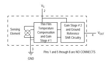
Figure 1. Fully Integrated Pressure Sensor Schematic
