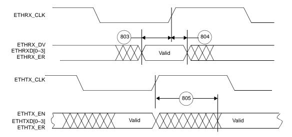
Figure 24. MII Mode Signal Timing
