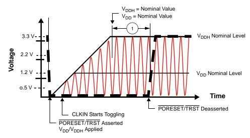
Figure 6. Start-Up Sequence:  $V_{DD}$  and  $V_{DDH}$  Raised Together
