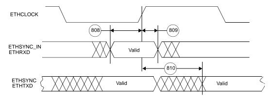
Figure 26. SMII Mode Signal Timing
