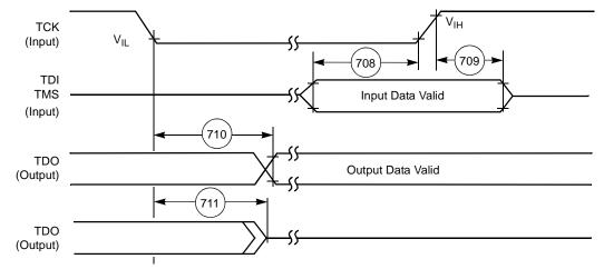
Figure 31. Test Access Port Timing Diagram
