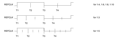
Figure 10. Internal Tick Spacing for Memory Controller Signals
