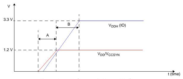
Figure 8. Power-Up Sequence for V<sub>DDH</sub> and V<sub>DD</sub>/V<sub>CCSYN</sub>
