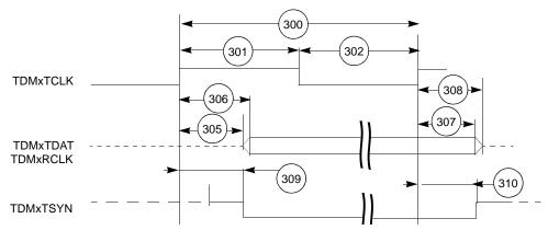
Figure 19. TDM Output Signals
