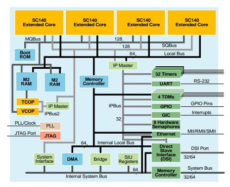
Figure 1. MSC8126 Block Diagram
