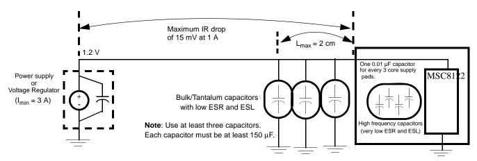
Figure 33. Core Power Supply Decoupling
