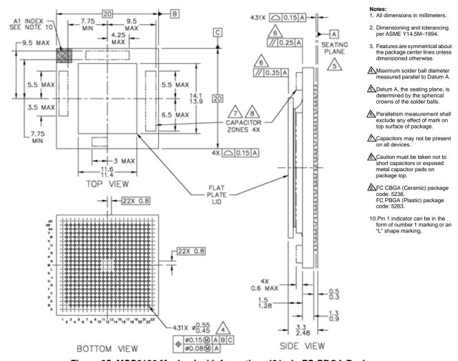
Figure 35. MSC8126 Mechanical Information, 431-pin FC-PBGA Package
