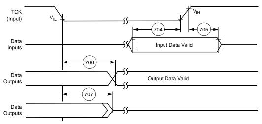
Figure 30. Boundary Scan (JTAG) Timing Diagram
