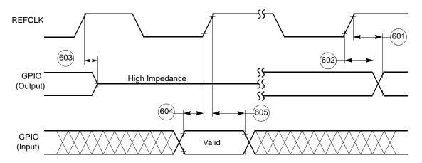
Figure 27. GPIO Timing
