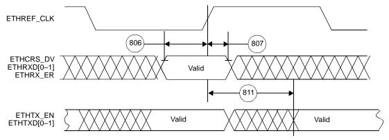
Figure 25. RMII Mode Signal Timing
