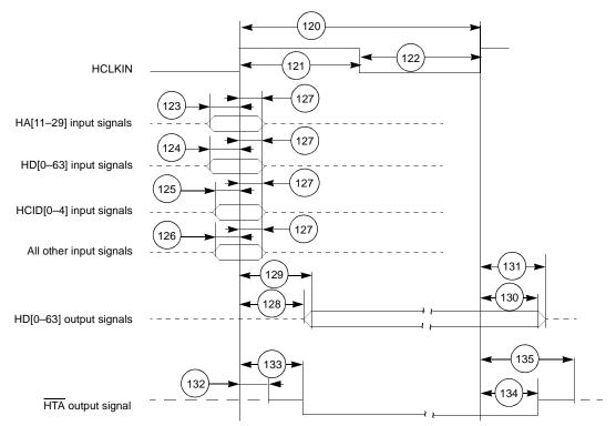
Figure 17. DSI Synchronous Mode Signals Timing Diagram
