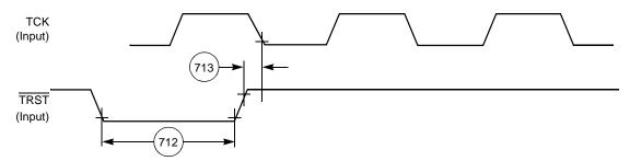
Figure 32. TRST Timing Diagram
