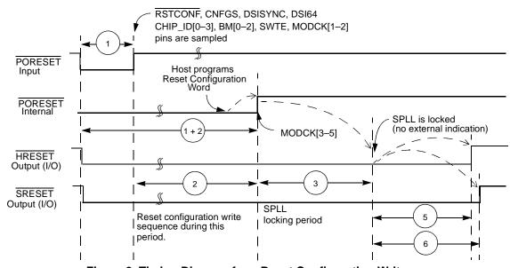
Figure 9. Timing Diagram for a Reset Configuration Write
