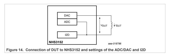
Apply the desired bias voltage to the first terminal (preferably as high as possible), and sequentially measure the voltage and current on the second terminal. The resistance is found by dividing the measured voltage drop with the measured current through the DUT.
