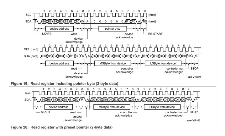
I3C, I<sup>2</sup>C-bus interface, 1 °C accuracy, digital temperature sensor
