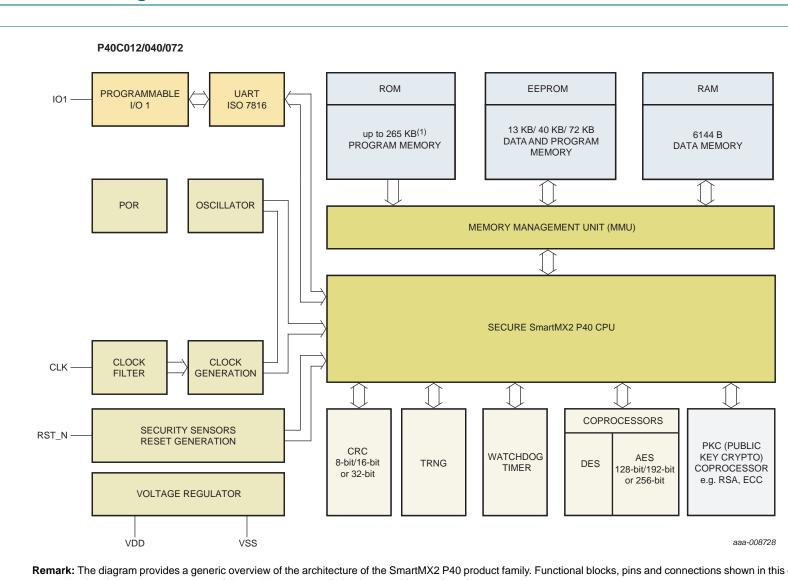
Remark: The diagram provides a generic overview of the architecture of the SmartMX2 P40 product family. Functional blocks, pins and connections shown in this diagram are optional and represent a super-set of those elements actually implemented in a real product.
