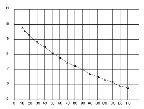
Figure 3-8 Typical Relaxation Oscillator Frequency vs. Trim Value @ 25°C
