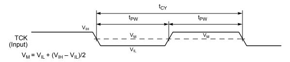
**Figure 3-14 Test Clock Input Timing Diagram**
