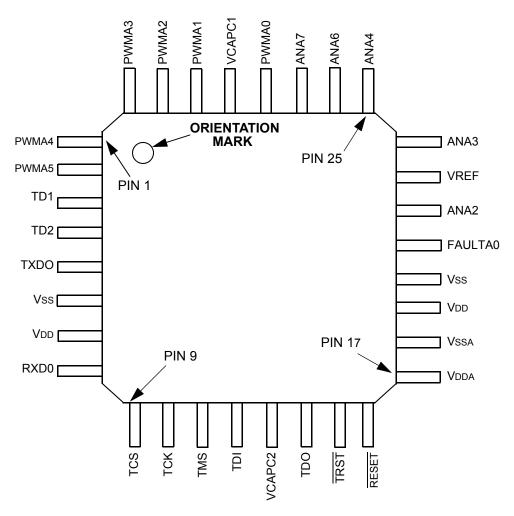
Figure 4-1 Top View, 56F802 32-pin LQFP Package
