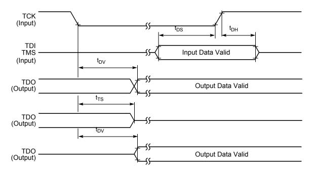
Figure 3-15 Test Access Port Timing Diagram
