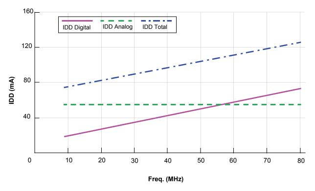
Figure 3-1 Maximum Run IDD vs. Frequency (see Note 6. in Table 3-4)
