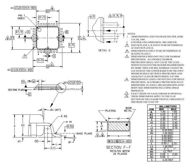
Figure 4-2 32-pin LQFP Mechanical Information (Case 873A)
