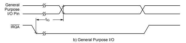
Figure 3-9 External Level-Sensitive Interrupt Timing
