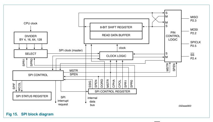
The SPI interface has four pins: SPICLK, MOSI, MISO and SS:
