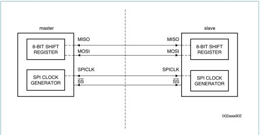
Fig 17. SPI dual device configuration, where either can be a master or a slave
