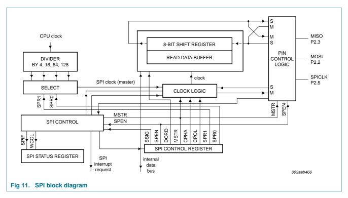
The SPI interface has three pins: SPICLK, MOSI, MISO and SS:
