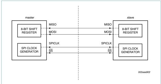
Fig 16. SPI dual device configuration, where either can be a master or a slave
