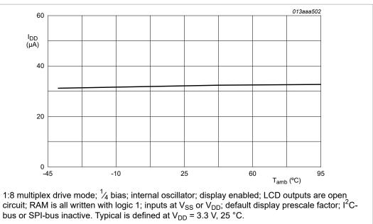
Figure 43. Typical I<sub>DD</sub> with respect to temperature
