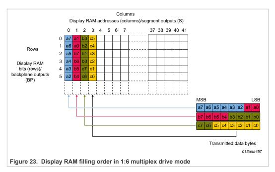
The remaining bits are wrapped over into the next column. In order to fill the whole RAM, 31 and a half bytes need to be sent to the PCA8536. After the last byte sent, the data pointer must be reset before the next RAM content update. Additional data bytes sent and any data bits that spill over the RAM will be discarded. Depending on the start address of the data pointer, there are three possible boundary conditions. See Figure 24.
