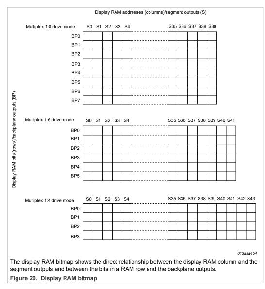
Logic 1 in the RAM bit map indicates the on-state ( $V_{on(RMS)}$ ) of the corresponding LCD element; similarly, logic 0 indicates the off-state ( $V_{off(RMS)}$ ). For more information on  $V_{on(RMS)}$  and  $V_{off(RMS)}$ , see Section 7.4.
