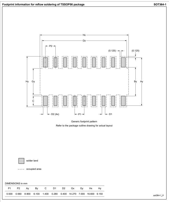
Figure 53. Footprint information for reflow soldering of SOT364-1 (TSSOP56) package
