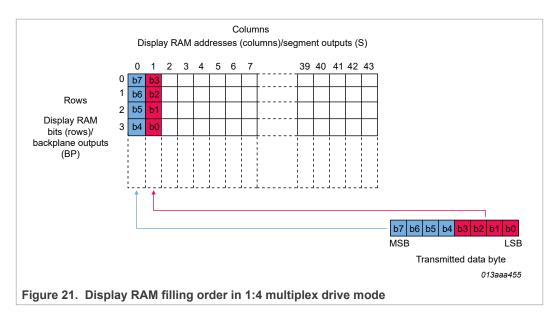
Depending on the start address of the data pointer, there is the possibility for a boundary condition. This will occur when more data bits are sent than fit into the remaining RAM. The additional data bits are discarded. See <u>Figure 22</u>.
