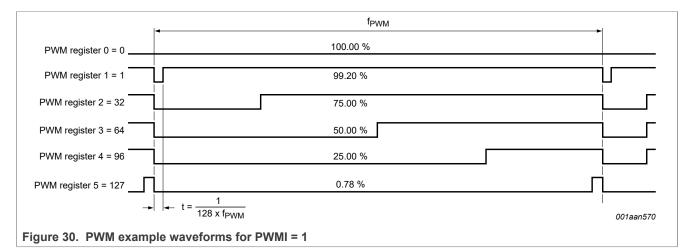
When PWM inversion mode is used, the PWM duty cycle can be calculated with:
