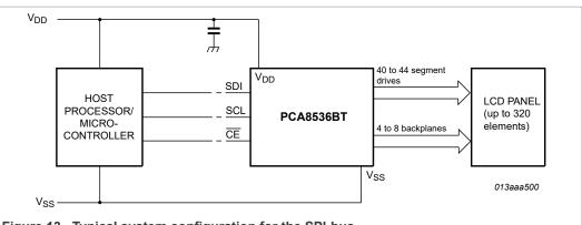
Figure 13. Typical system configuration for the SPI-bus
