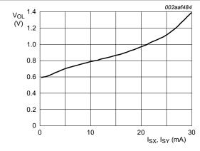
Figure 11. Typical SX/SY current versus LOW-level output voltage
