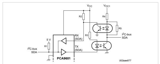
This simple example may be limited, if using lowest-cost couplers, to speeds as low as 5 kHz. Refer to application notes for schematics suitable for operation to 400 kHz or higher.
