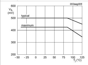
$V_{\text{IL}}$  at SX changes over temperature range.
