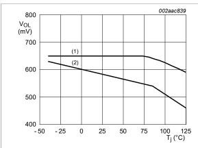
V<sub>OL</sub> at SX typical and limits over temperature.
