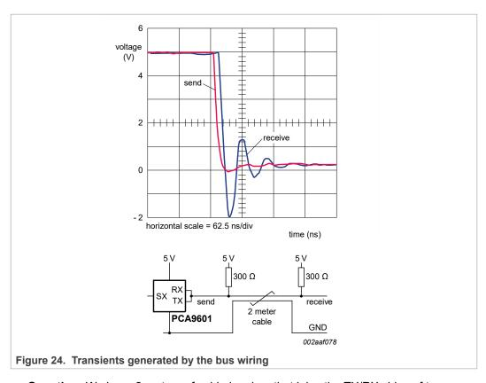
**Question:** We have 2 meters of cable in a bus that joins the TX/RX sides of two PCA9601 devices. When one TX drives LOW the other PCA9601 TX/RX is driven to -0.8 V for over 50 ns. What is the expected value and the theoretically allowed value of undershoot?
