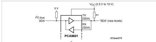
Figure 12. Interfacing a standard 3 mA I<sup>2</sup>C-bus or one with TTL levels (e.g. SMBus) to higher voltage or higher current sink (e.g. Fast-mode Plus) devices
