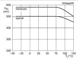
$V_{\text{IH}}$  at SX changes over temperature range.
