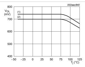
V<sub>OL</sub> at SX typical and limits over temperature.
