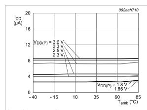
$I_{DD} = I_{DD(I2C-bus)} + I_{DD(P)}$
