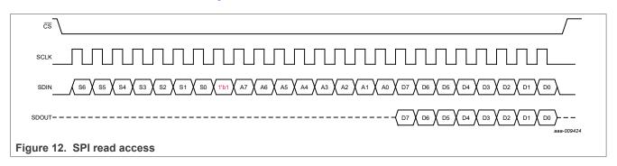
The SDOUT pin is high-impedance for the first 16 cycles of the read cycle. The SDOUT pin is driven only if a valid register address has been specified. The dummy data on the SDIN for the last 8 clock pulses is not clocked into the register.
