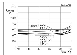
Figure 24. Standby supply current versus ambient temperature
