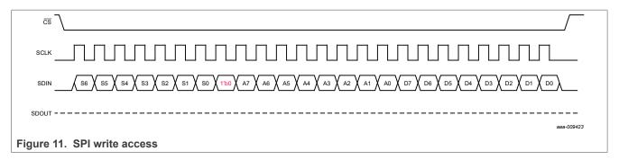
If more than 24 bits of data are transferred, that is, there are more than 24 clock pulses before deasserting the  $\overline{\text{CS}}$ , the register address is auto incremented. Auto Increment is discussed in Section 6.10.1.3.
