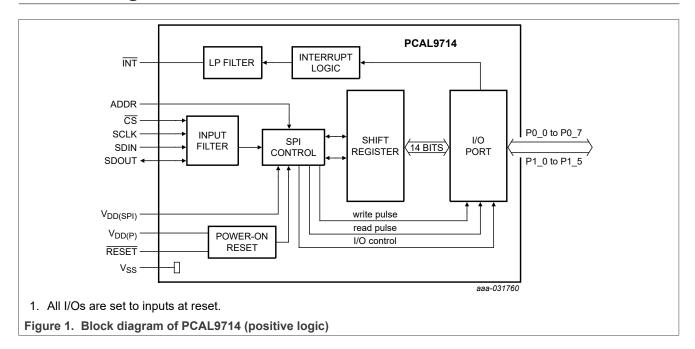
Ultra low-voltage translating 14-bit SPI I/O expander with Agile I/O features, interrupt output, and
