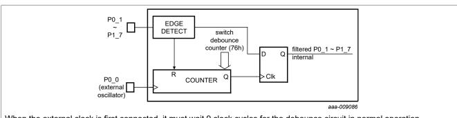
When the external clock is first connected, it must wait 9 clock cycles for the debounce circuit in normal operation.
