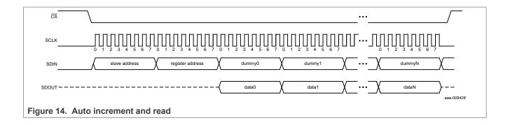
Ultra low-voltage translating 14-bit SPI I/O expander with Agile I/O features, interrupt output, and
