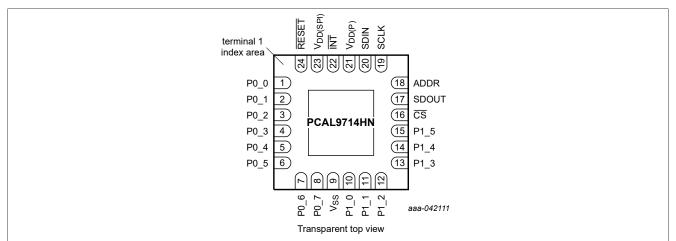
1. The exposed center pad, if used, must be connected only as a secondary ground or must be left electrically open.
