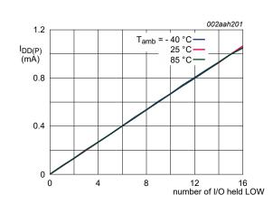
Figure 26. Supply current versus number of I/O held I OW
