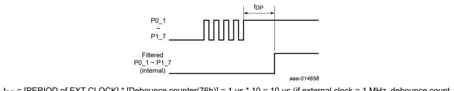
$t_{DP}$  = [PERIOD of EXT CLOCK] \* [Debounce counter(76h)] = 1  $\mu$ s \* 10 = 10  $\mu$ s (if external clock = 1 MHz, debounce count register (76h) = 0Ah)
