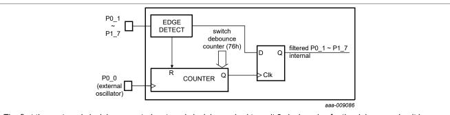
The first time external clock is connected, external clock is required to wait 9 clock cycles for the debounce circuit in normal operation.
