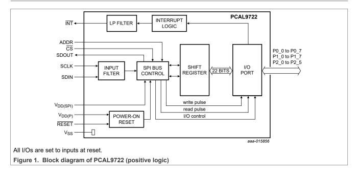
Ultra low-voltage translating 22-bit SPI I/O expander with Agile I/O features, interrupt output and
