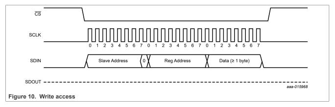
If more than 24 bits of data are transferred i.e. there are more than 24 clock pulses before de-asserting the CS, the register address is auto incremented. Auto Increment is discussed in a section below.
