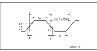
Figure 4. SDRAM Output clock
