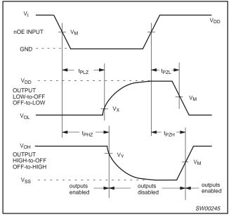
Figure 2. 3-State enable and disable times
