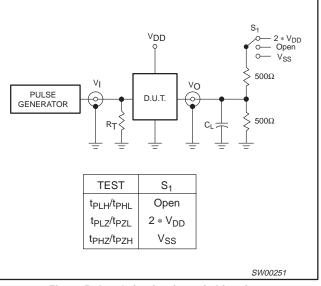
Figure 5. Load circuitry for switching times
