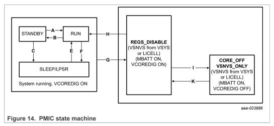
In the "System On" modes, some or all of the PMIC regulators are powered and in general the system processor is powered.
