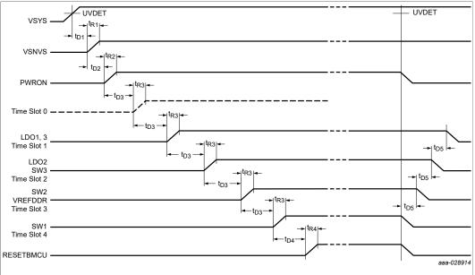
Figure 15. A4 startup and power down sequence
