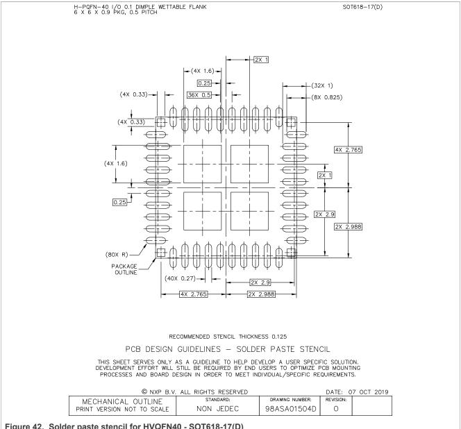
Figure 42. Solder paste stencil for HVQFN40 - SOT618-17(D)
