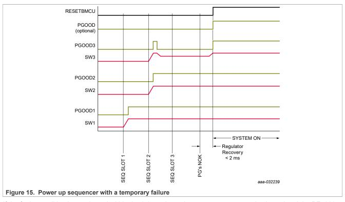
If the faulty condition is not cleared within the 2.0 ms timer, the power up sequence is aborted and the PF5023 turns off all voltage regulators enabled so far as shown in <u>Figure 16</u>.
