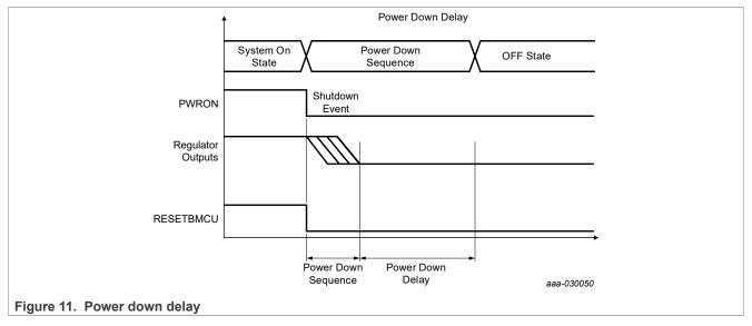
The default value of the OTP\_PD\_SEQ\_DLY[1:0] bits on an unprogrammed OTP device shall be 00.
