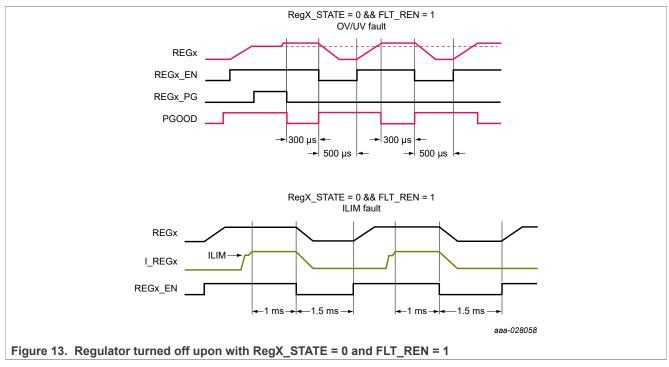
When any of the regulators is controlled by hardware using the ENx pins and programmed to turn off upon an OV, UV or ILIM fault, the \_FLT\_REN bit still controls whether the regulator returns to its previous state or not regardless the state of the ENx pin.
