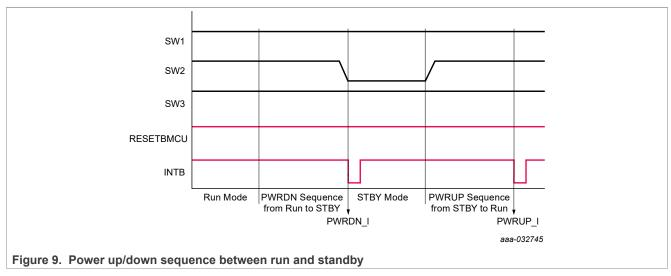
The PWRUP\_I interrupt is set while transitioning from standby to run, even if the sequencer is not used. This is used to indicate that the transition is complete and device is ready to perform proper operation.
