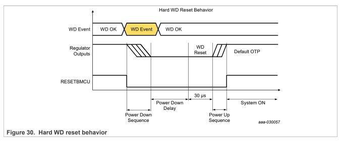
After a WD reset, the PMIC may enter the Standby state depending on the status of STANDBY pin.
