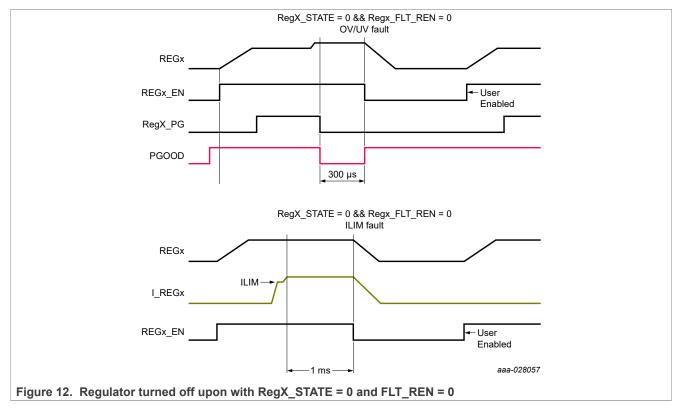
When a regulator is programmed to disable upon an OV, UV, or ILIM fault, a bit is provided to decide whether a regulator can return to its previous configuration or remain disabled when the fault condition is cleared.
