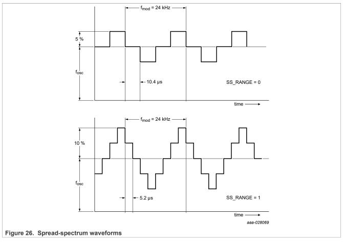
If the frequency spread-spectrum is enabled, the switching regulators should be set in PWM mode to ensure clock synchronization at all time.
