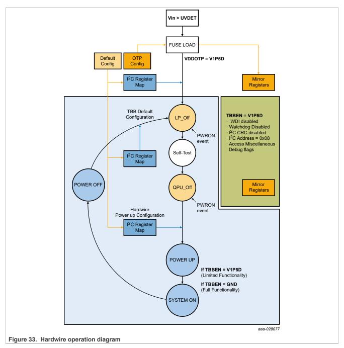
For simplicity, the default hardwire configuration in PF5023 is organized based on the OTP register map as shown in Table 58.
