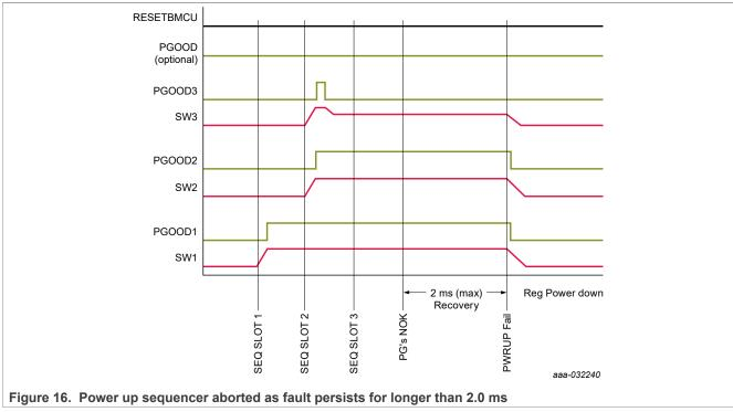
Supplies enabled after RESETBMCU are checked for OV, UV and ILIM faults after each of them are enabled. If an OV, UV or ILIM condition is present, the PF5023 starts a fault detection and protection mechanism as
