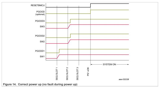
If any of the regulators are powered up before RESETBMCU is out of regulator, RESETBMCU is not deasserted and the power up sequence is stopped for up to 2.0 ms. If the fault is cleared and all internal PG signals are asserted within the 2.0 ms timer, RESETBMCU is de-asserted and the power up sequence continues where it stopped as shown in <u>Figure 15</u>.
