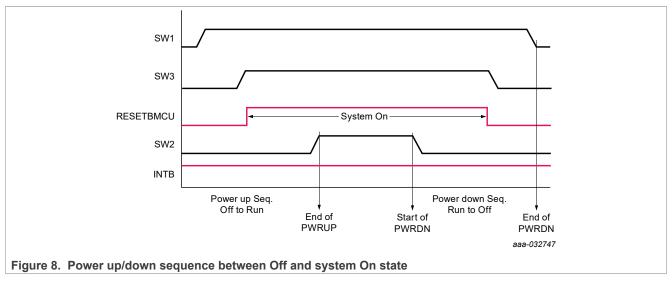
When transitioning from Standby mode to Run mode, the power up sequencer is activated only if any of the external regulators is re-enabled during this transition. If none of the regulators toggle from Off to On and only voltage changes are being performed when entering or exiting Standby mode, the changes for the voltage regulators are made simultaneously rather than going through the power up sequencer.
