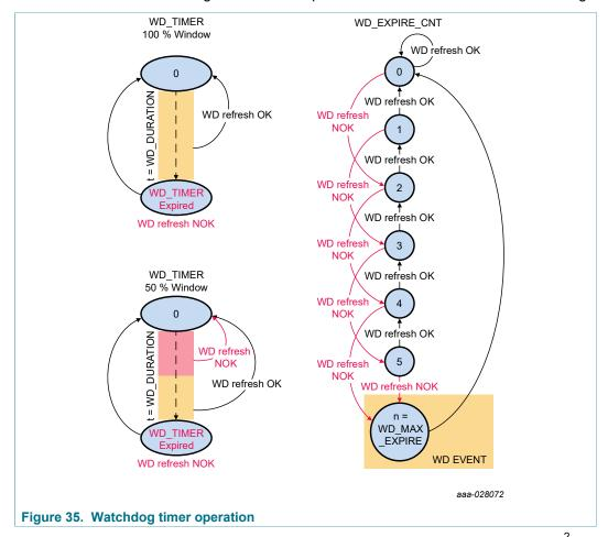
The watchdog function can be enabled or disabled by writing the WD\_EN bit on the  $I^2C$  register map. When the I2C\_SECURE\_EN = 1, a secure write must be performed to change the WD\_EN bit.
