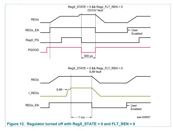
When a regulator is programmed to disable upon an OV, UV, or ILIM fault, a bit is provided to decide whether a regulator can return to its previous configuration or remain disabled when the fault condition is cleared.
