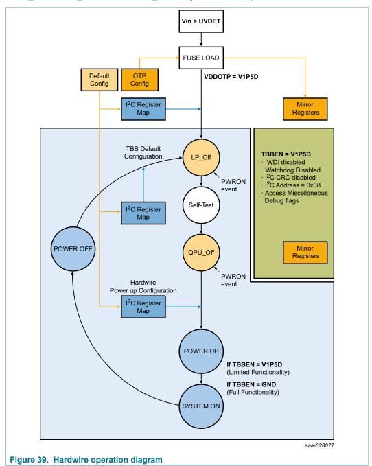
For simplicity, the default hardwire configuration in PF8100/PF8200 is organized based on the OTP register map as shown in Table 78.
