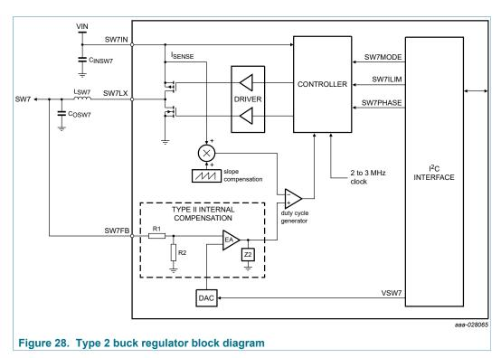
Buck regulator SW7 uses 5 bits to set the output voltage. The VSW7[4:0] sets the output voltage during the run and the standby mode.
