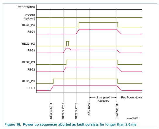
Supplies enabled after RESETBMCU are checked for OV, UV and ILIM faults after each of them is enabled. If an OV, UV or ILIM condition is present, the PF8100/PF8200 starts a fault detection and protection mechanism as described in <a href="Section 14.7">Section 14.7 "Fault detection"</a>. At this point, the MCU should be able to read the interrupt and react upon a fault event as defined by the system.
