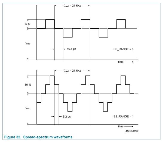
If the frequency spread-spectrum is enabled, the switching regulators should be set in PWM mode to ensure clock synchronization at all time.
