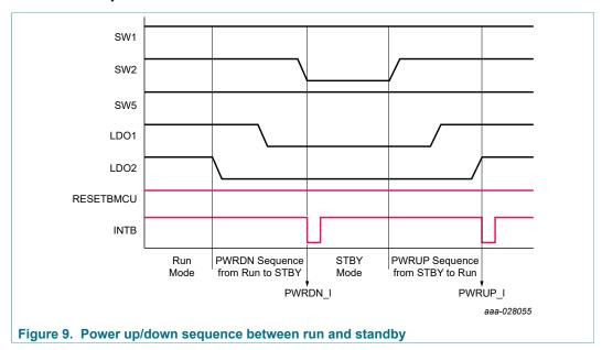
The PWRUP\_I interrupt is set while transitioning from standby to run, even if the sequencer is not used. This is used to indicate that the transition is complete and device is ready to perform proper operation.
