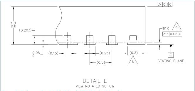
Figure 48. Package outline detail for E-type HVQFN56 (Industrial grade)
