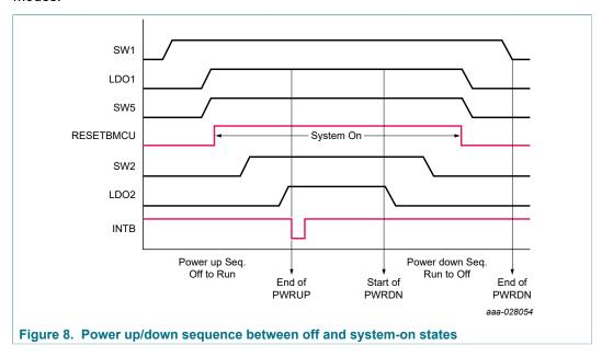
When transitioning from standby mode to run mode, the power up sequencer is activated only if any of the external regulators is re-enabled during this transition. If none of the regulators toggle from off to on and only voltage changes are being performed when entering or exiting standby mode, the changes for the voltage regulators are made simultaneously rather than going through the power up sequencer.
