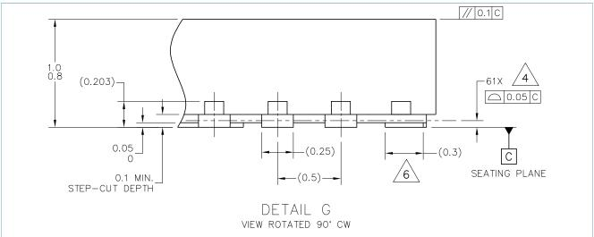
Figure 42. Package outline detail for WF-type HVQFN56 (Automotive grade)
