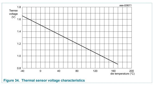
As the temperature crosses the thermal thresholds, the corresponding interrupts are set to notify the system. The processor may take appropriate action to bring down the temperature (either by turning off external regulators, reducing load, or turning on a fan).
