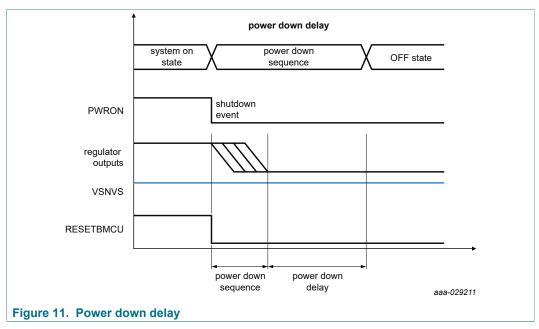
The default value of the OTP\_PD\_SEQ\_DLY[1:0] bits on an unprogrammed OTP device shall be 00.
