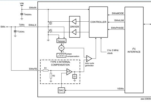
Figure 24. Buck regulator block diagram
