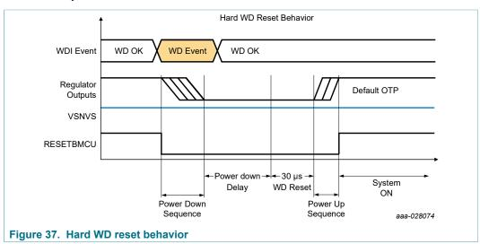
After a WD reset, the PMIC may enter the standby state depending on the status of STANDBY pin.
