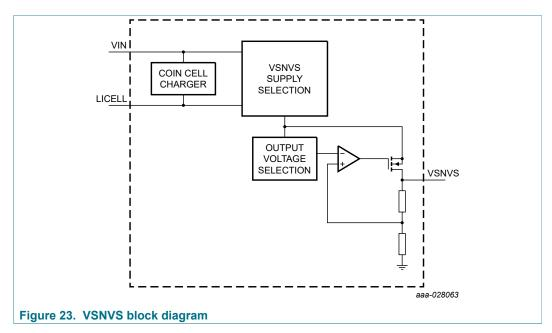
The VSNVS output keeps regulation through all states, including the system-on, off modes, power down sequence, watchdog reset, fail-safe transition and fail-safe state as long as it has a valid input (VIN or LICELL), and the output has been configured by the OTP\_VSNVSVOLT[1:0] registers.
