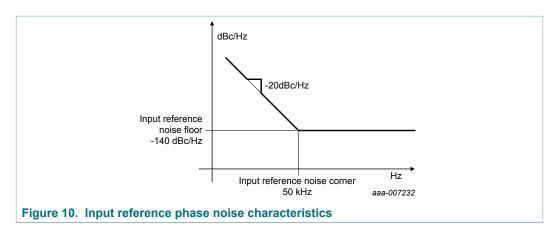
This phase noise is equivalent to an RMS jitter of 6.23 ps from 10 Hz to 1 MHz. For configuration of input frequency, refer to [8]. There are 6 pre programmed and validated frequencies for the PLL: 13 MHz, 19.2 MHz, 24 MHz, 26 MHz, 38.4 MHz and 52 MHz.
