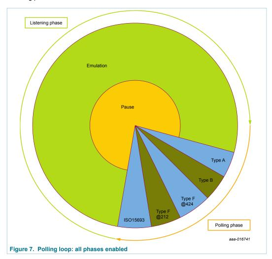
Listening phase uses Standby power state (when no RF field) and PN7120 goes to Listener mode when RF field is detected. When in Polling phase, PN7120 goes to Poller mode.
