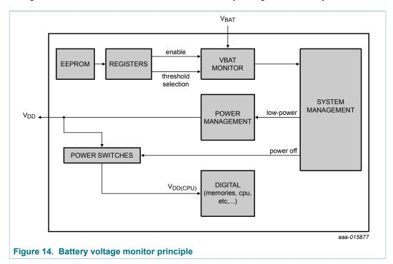
The value of the critical level can be configured to 2.3 V or 2.75 V by an EEPROM setting. This value has a typical hysteresis around 150 mV.
