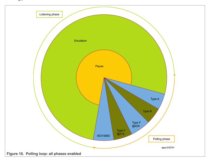
Listening phase uses Standby power state (when no RF field) and PN7150 goes to Listener mode when RF field is detected. When in Polling phase, PN7150 goes to Poller mode.
