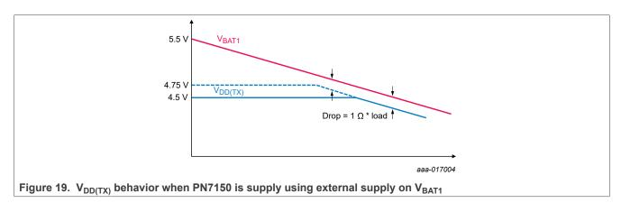
Figure 19 shows the behavior of  $V_{DD(TX)}$  depending on  $V_{BAT1}$  value.
