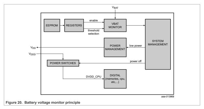
The value of the critical level can be configured to 2.3 V or 2.75 V by an EEPROM setting. This value has a typical hysteresis around 150 mV.
