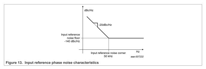
This phase noise is equivalent to an RMS jitter of 6.23 ps from 10 Hz to 1 MHz. For configuration of input frequency, refer to [9]. Thee six pre-programmed and validated frequencies for the PLL are: 13 MHz, 19.2 MHz, 24 MHz, 26 MHz, 38.4 MHz and 52 MHz.
