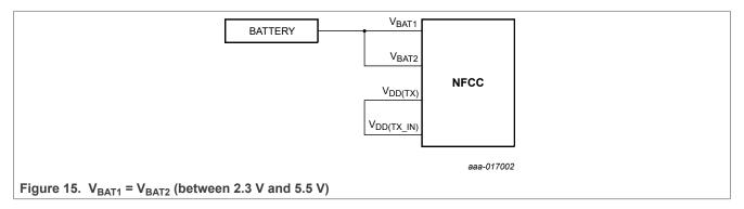
V<sub>DD(TX)</sub> value shall be chosen according to the minimum targeted V<sub>BAT</sub> value for which reader mode shall work.
