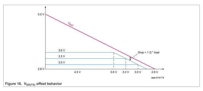
Figure 16 shows  $V_{DD(TX)}$  offset disabled behavior for both cases of  $V_{DD(TX)}$  programmed for 3.0 V, 3.3 V or 3.6 V.
