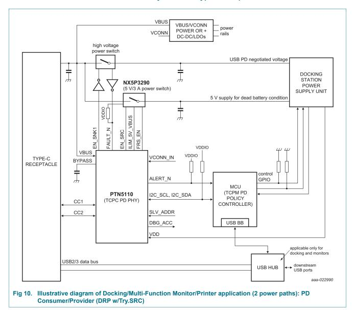
The example applications are Multi- function monitor, Dock or Printer with local power. PTN5110 is configured for DRP with preference for Try.SRC role. This would allow this platform to become a power source wherever possible including when the host platform is in dead battery condition. Once the host is powered, data role swap is performed and any relevant PD power negotiation is carried out.
