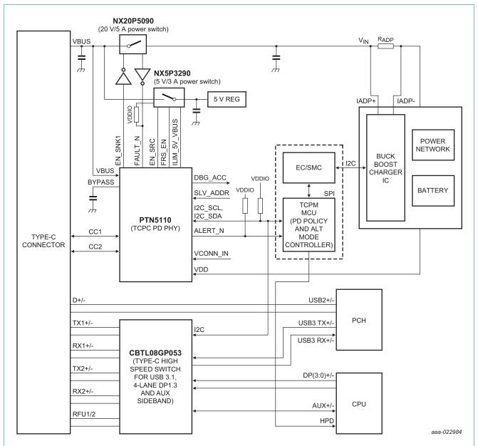
Fig 4. Illustrative diagram of Notebook/Ultrabook/Tablet application (Separate source and sink power paths): PD Provider/Consumer role (Source role under Normal power/battery; Sink role under dead battery condition)
