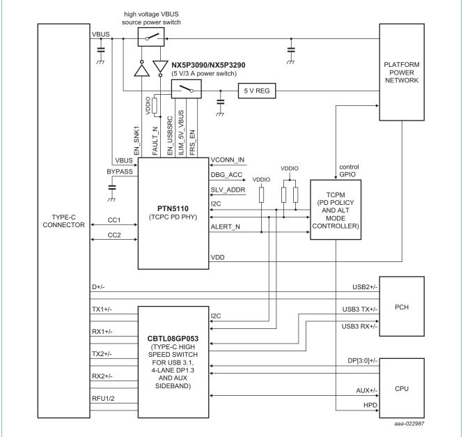
Fig 7. Illustrative diagram of Desktop PC application (2 Source power paths): PD Provider only (Source role under powered condition)
