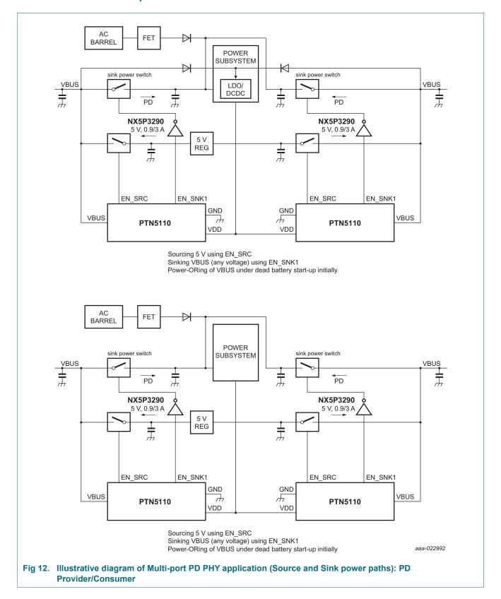
Two example scenarios are captured in the illustrations. This application can be a typical notebook PC with two-port support. Depending on whether the PC uses Buck boost charger or regular NVDC charger, the platform implementation would be different.
