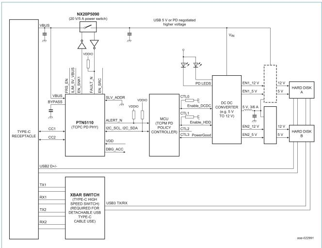
Fig 11. Illustrative diagram of Portable Hard Drive application (sink power path): PD Consumer only
