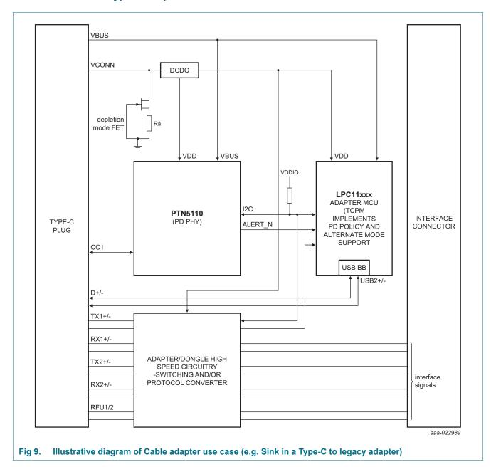
In this illustration, PTN5110 is inside Type-C cable adapter operating in Sink role. Some example use cases are Type-C to DP adapter, Type-C to VGA adapter, Type-C to Thunderbolt adapter etc. PTN5110 serves as PD PHY layer device for a Cable adapter management MCU or dedicated PD MCU wherein PD policy management, Alternate mode and VDM support are handled. The USB Billboard device is assumed to be implemented as part of adapter management MCU.
