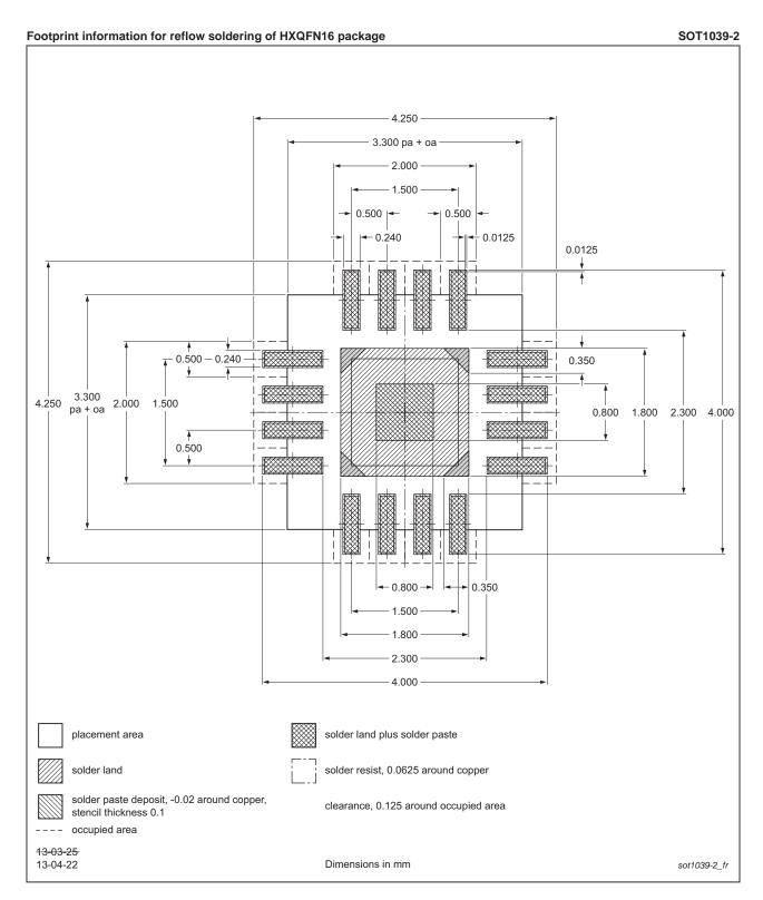
Fig 22. PCB footprint for SOT1039-2 (HXQFN16); reflow soldering
