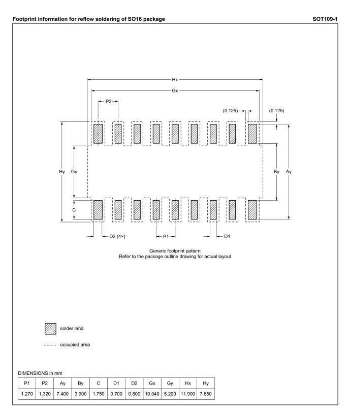
Fig 21. PCB footprint for SOT109-1 (SO16); reflow soldering
