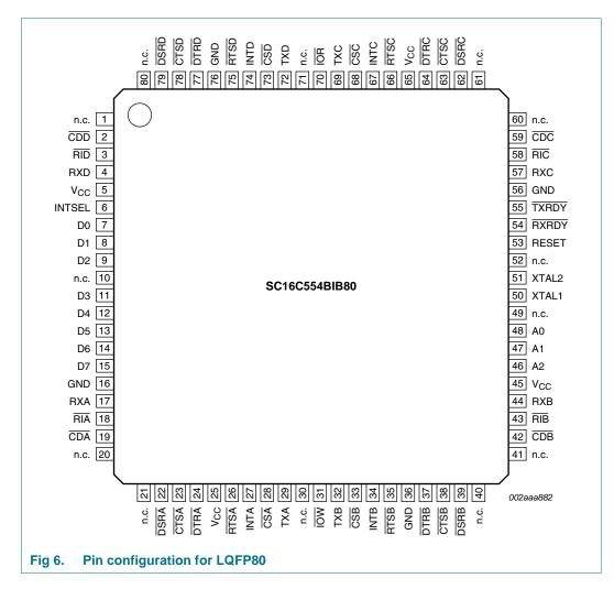
5 V, 3.3 V and 2.5 V quad UART, 5 Mbit/s (max.) with 16-byte FIFOs
