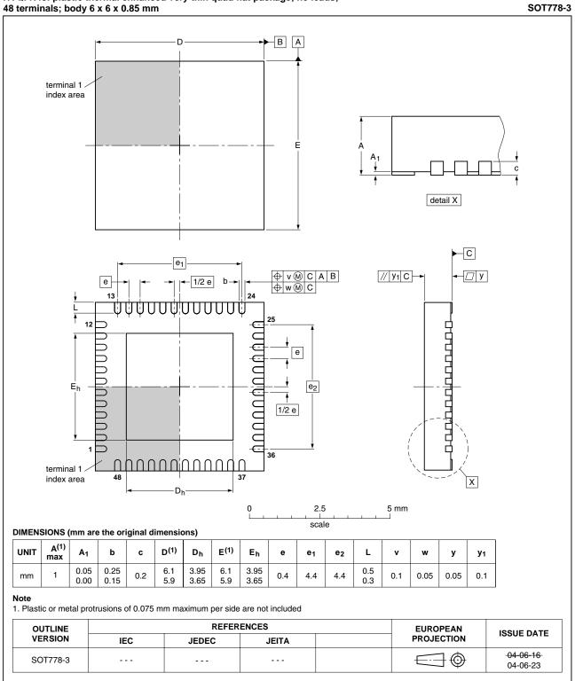
HVQFN48: plastic thermal enhanced very thin quad flat package; no leads; 48 terminals; body 6 x 6 x 0.85 mm
