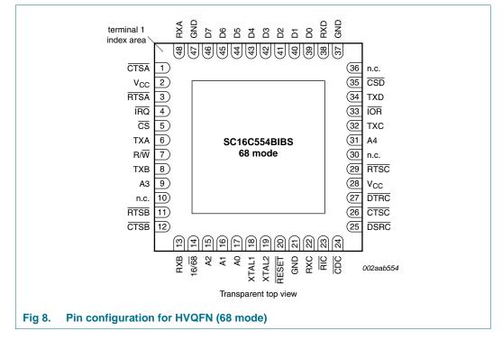
5 V, 3.3 V and 2.5 V quad UART, 5 Mbit/s (max.) with 16-byte FIFOs
