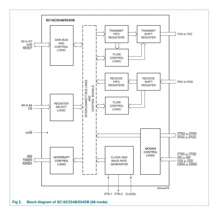
5 V, 3.3 V and 2.5 V quad UART, 5 Mbit/s (max.) with 16-byte FIFOs
