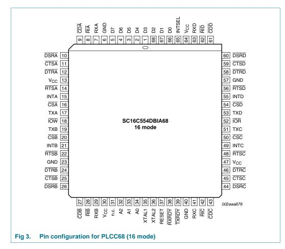
5 V, 3.3 V and 2.5 V quad UART, 5 Mbit/s (max.) with 16-byte FIFOs
