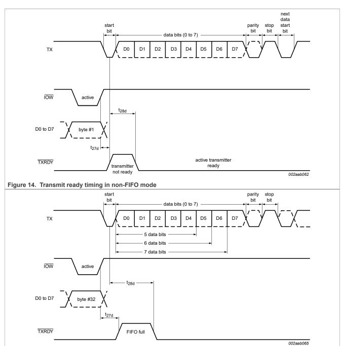
Figure 15. Transmit ready timing in FIFO mode (DMA mode '1')
