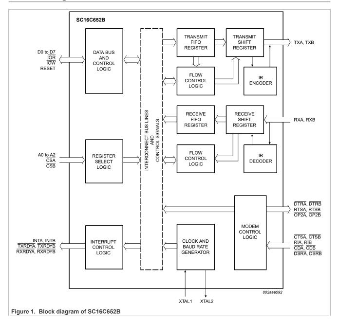
5 V, 3.3 V and 2.5 V dual UART, 5 Mbit/s (max.) with 32-byte FIFOs and infrared (IrDA) encoder/
