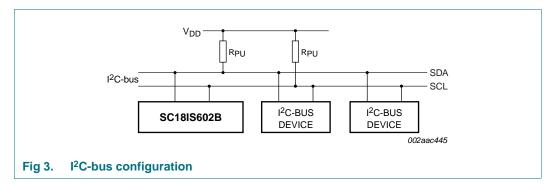
The SC18IS602B device provides a byte-oriented  $I^2C$ -bus interface that supports data transfers up to 400 kHz. When the  $I^2C$ -bus master is reading data from SC18IS602B, the device will be a slave-transmitter. The SC18IS602B will be a slave-receiver when the  $I^2C$ -bus master is sending data. At no time does the SC18IS602B act as an  $I^2C$ -bus master, however, it does have the ability to hold the SCL line LOW between bytes to complete its internal processes.
