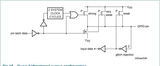
Fig 15. Quasi-bidirectional output configuration
