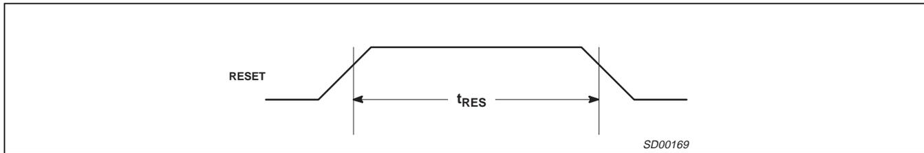
Figure 10. Reset Timing
