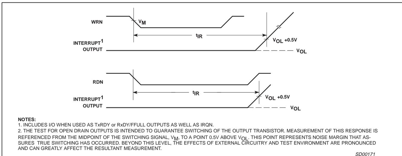
Figure 12. Interrupt Timing
