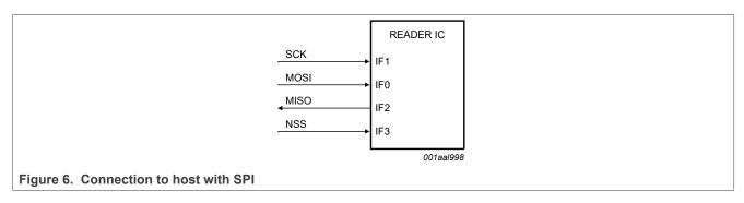
The SLRC610 acts as a slave during the SPI communication. The SPI clock SCK has to be generated by the master. Data communication from the master to the slave uses the Line MOSI. Line MISO is used to send data back from the SLRC610 to the master.
