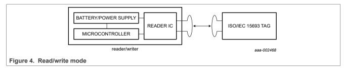
A typical system using the SLRC610 is using a microcontroller to implement the higher levels of the contactless communication protocol and a power supply (battery or external supply).
