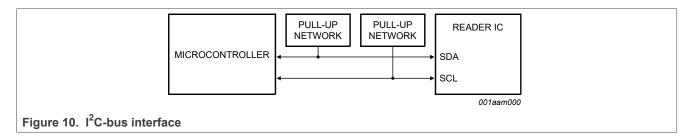
The voltage level on the I2C pins is not allowed to be higher than PVDD.
