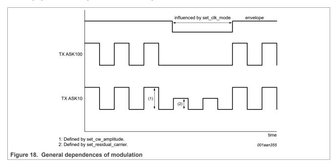
Note: When changing the continuous carrier amplitude, the residual carrier amplitude also changes, while the modulation index remains the same.
