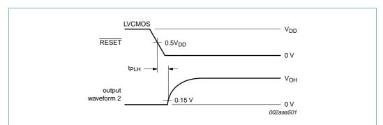
Fig 19. Voltage waveforms, open-drain output LOW-to-HIGH transition time with respect to **RESET** input
