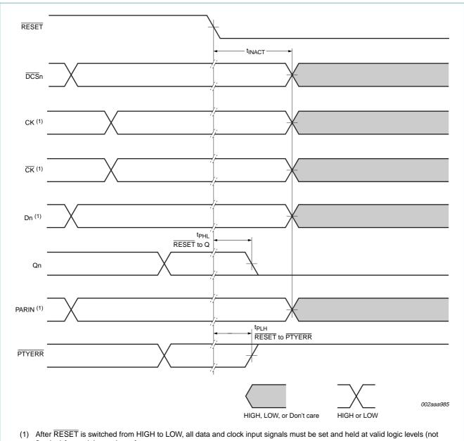
(1) After RESET is switched from HIGH to LOVV, all data and clock input signals must be set and held at valid logic levels (no floating) for a minimum time of t<sub>INACT(max)</sub>.
