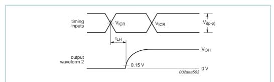
Fig 21. Voltage waveforms, open-drain output LOW-to-HIGH transition time with respect to clock inputs
