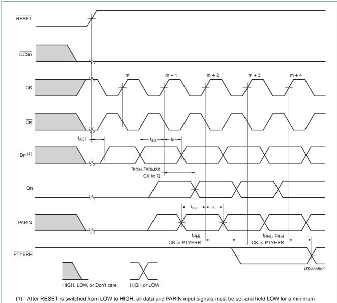
(1) After RESET is switched from LOW to HIGH, all data and PARIN input signals must be set and neid LOW for a minimum time of t<sub>ACT(max)</sub> to avoid false error.
