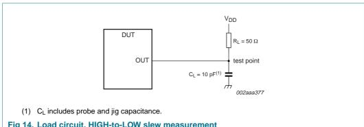
Fig 14. Load circuit, HIGH-to-LOW slew measurement
