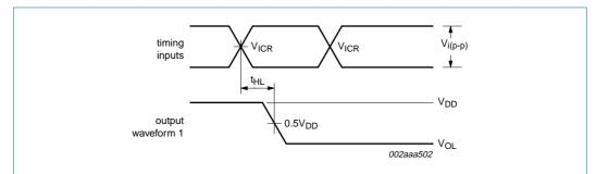
Fig 20. Voltage waveforms, open-drain output HIGH-to-LOW transition time with respect to clock inputs
