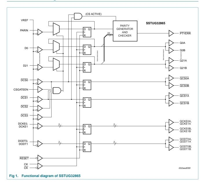
1.8 V DDR2-1G registered buffer with parity
