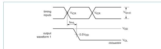
Fig 21. Voltage waveforms, open-drain output HIGH-to-LOW transition time with respect to clock inputs
