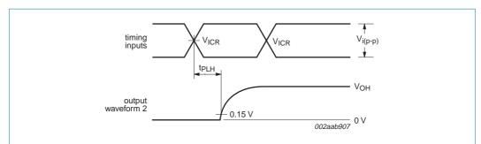
Fig 22. Voltage waveforms, open-drain output LOW-to-HIGH transition time with respect to clock inputs
