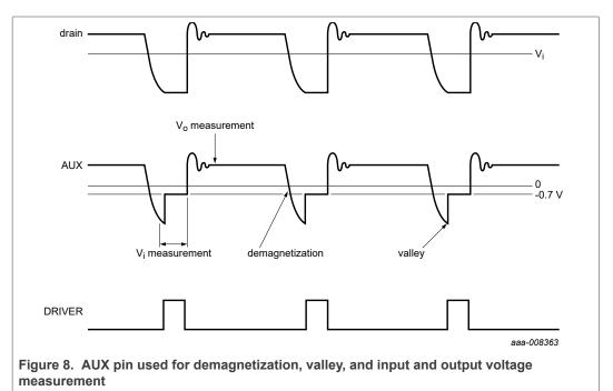
When the external MOSFET is switched on, the voltage at the auxiliary winding reflects the input voltage. The AUX pin is clamped to -0.7 V. The output current is a measure of the input voltage. This current value is internally used for an accurate OPP.
