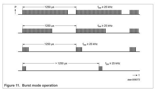
To achieve a good transient response in burst mode, the system starts switching immediately at an increased output load, allowing a shorter burst period. Eventually, it regulates to the required burst period by increasing the number of driver pulses (see Figure 12).
