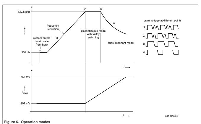
At high output power, the converter operates in quasi-resonant mode. The next converter cycle starts after demagnetization of the transformer and detection of the valley. In quasi-resonant mode, switching losses are minimized because the external MOSFET is switched on while the drain-source voltage is minimal.
