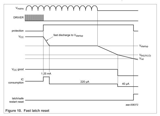
Using a 10  $\mu$ F VCC capacitor, the fast latch reset time is < 0.6 s. If the mains is not shorted but removed, a discharge of the X-capacitor can cause an additional waiting time.
