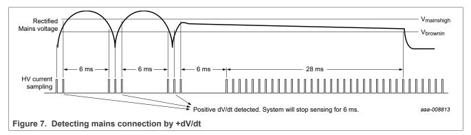
If the system does not detect a positive dV/dt for 28 ms, it assumes that the mains is disconnected. In that case, the HV pin is continuously pulled to ground, discharging the external X-capacitor.
