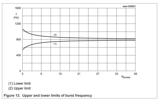
When the number of driver pulses within one burst period exceeds 40, the system switches to normal mode again.
