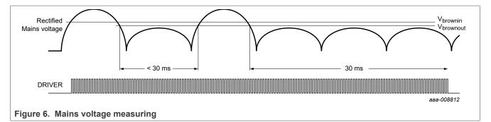
When the mains voltage is measured by pulling the HV pin to ground, the digital control calculates if there is a positive dV/dt at the mains. A positive dV/dt implies that a mains is connected.
